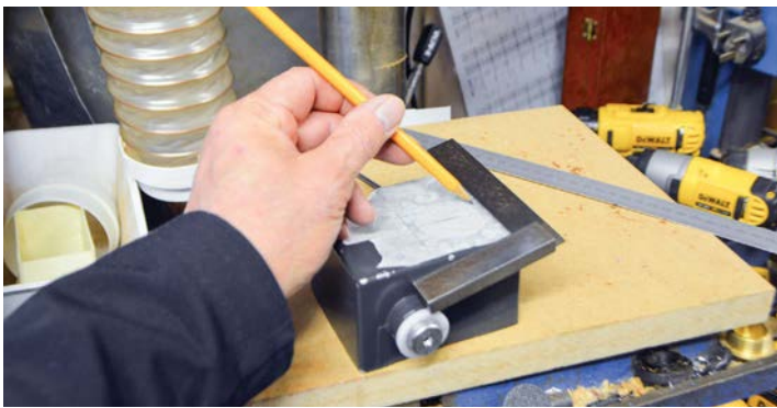
Carefully mark, punch and drill
