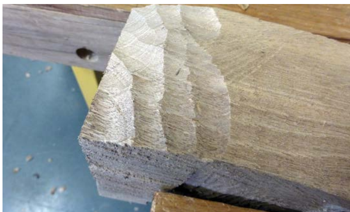
A fluted surface resulting from using the No.6 gouge
