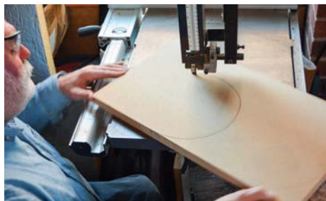
Cut MDF discs freehand
