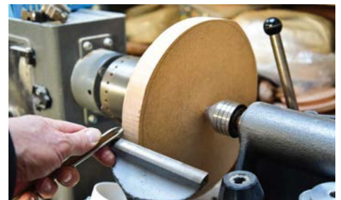
True and profile disc edges
