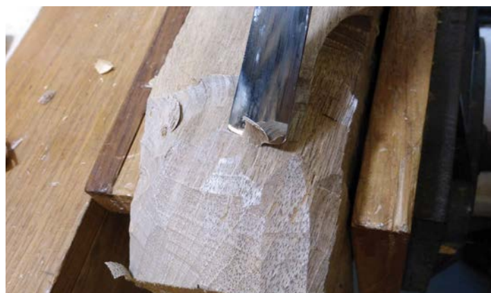
A smoother surface from the No.4 gouge
