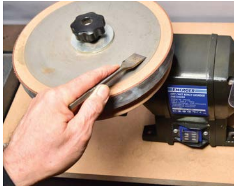
Stage two - fine grinding
