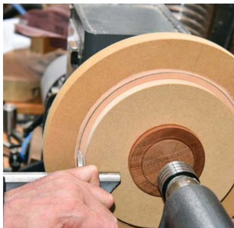
True disc edge with skew chisel
