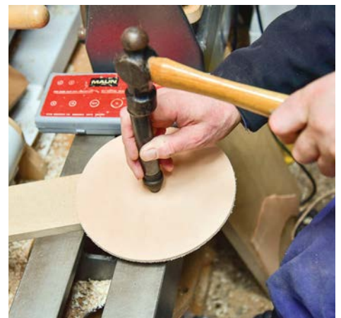
Carefully punch centre hole
