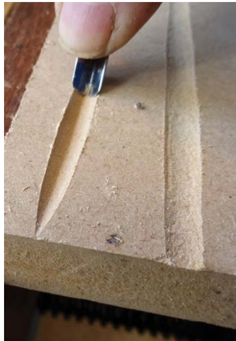
A V cut in MDF with tool being dragged backwards to hone. Shallow groove on the right is for a gouge. No compound is needed
