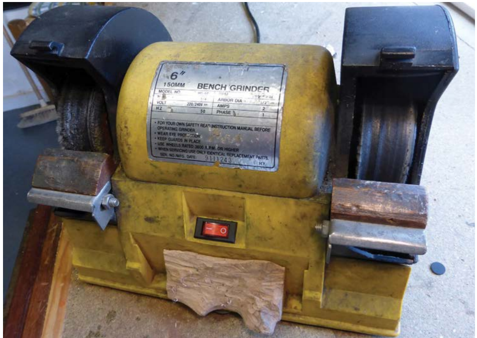
The direction of rotation has been reversed by turning the motor round, a hard felt wheel added (right) and a close stitched rag wheel (left) each with a wooden slope to give the correct angle for honing
