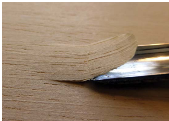
Note the grain splitting ahead of the cutting edge of the tool
