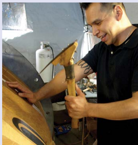
Apprentice Travis Peal uses an elbow adze to rapidly clear excess material
