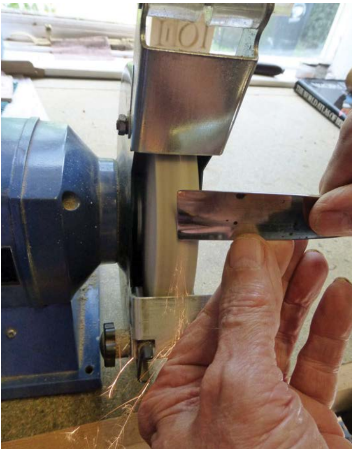
This shows the forming of a flat bevel holding the tool at right angles to the direction of rotation rocking it back and forth to keep the bevel in contact with the grinding wheel. This can be any fine abrasive wheel and the direction of rotation is unimportant. Guards have been moved for clarity
