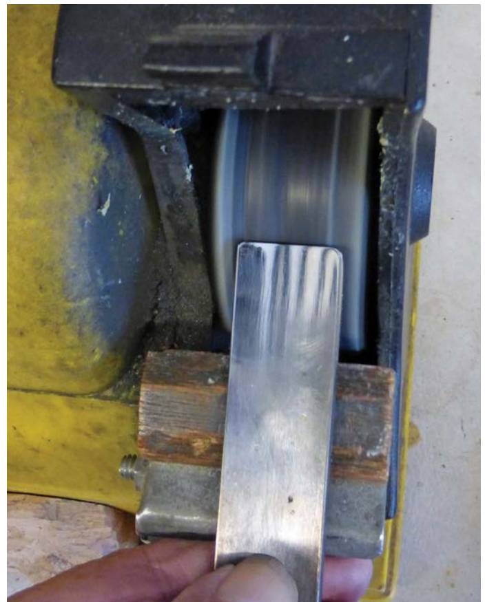
Honing is done on a rag or hard felt wheel rotating away from you at the top (opposite to the normal direction of grinding wheels). An adjustable rest can set the angle or a wooden block added if the rest is not adjustable
