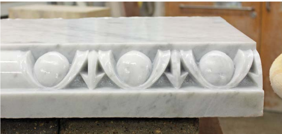
A section of Naz's egg-and-dart work in marble after rinsing
