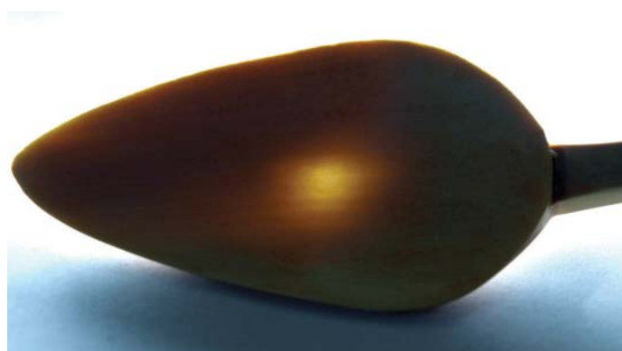
Light visible through your bowl indicates the wood is getting too thin
