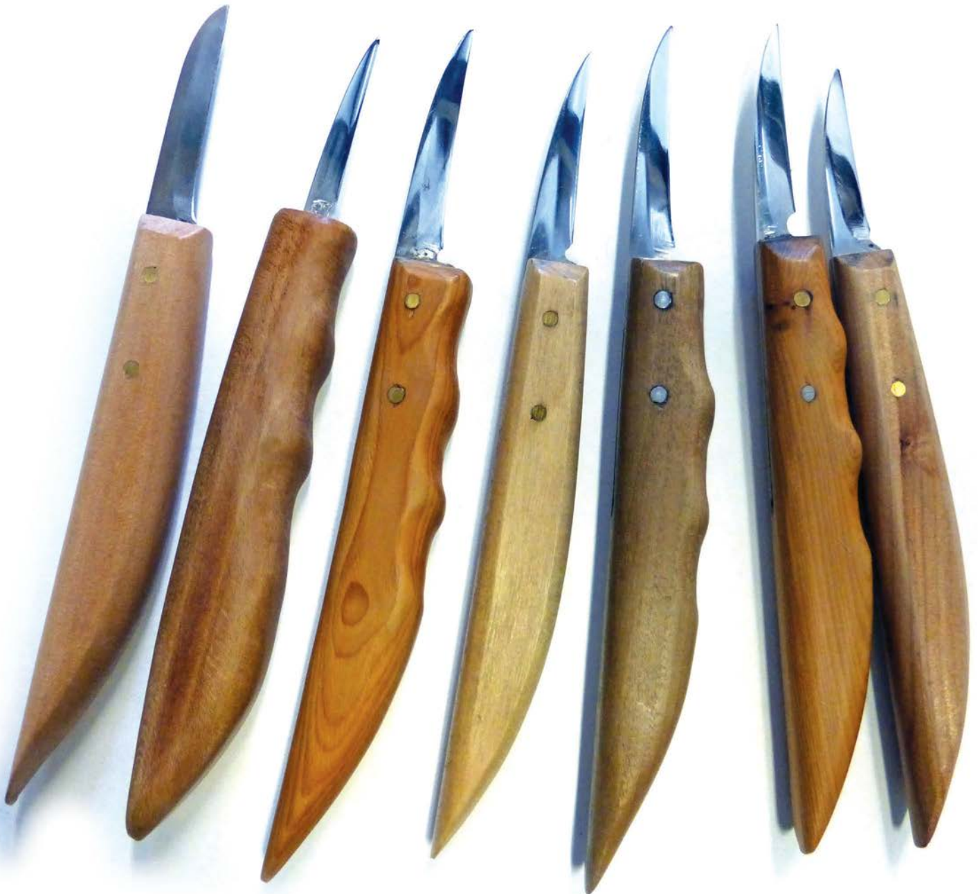
Knife blades from R. Murphy in the US. On left is standard knife and the rest are blades modified and/or handled by carvers
