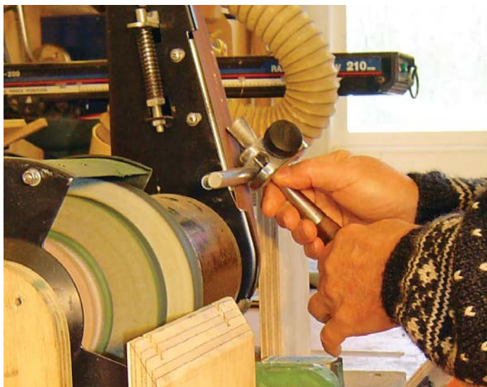
Regrinding a gouge with a Tormek jig
