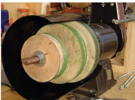
Out-board extension for shaft support
