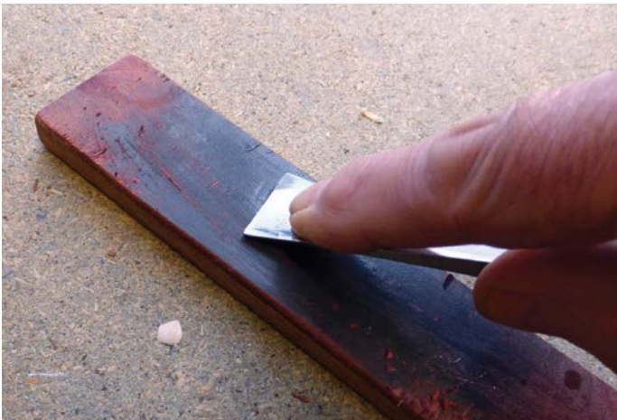
Honing on strop keeping whole bevel in contact all the time
