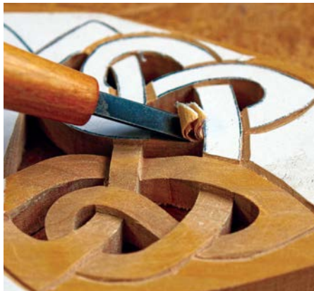
Be careful not to lever the chisel at the intersections because you run the risk of snapping off the crossing section
