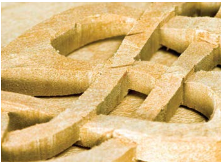
Take off as little material as possible to get the intersection level again. You may need to do this over a larger area to disguise the issue
