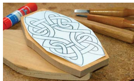
Gluing a photocopy to your workpiece is the easiest way to get started on your carving
