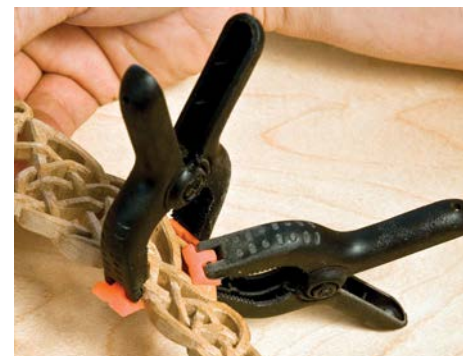
If clamps are required, be careful they don't distort the joint or generate so much force that they break another area
