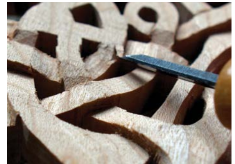
Chisel slips can knock chunks out of your line-work. Try to retain the chip if possible or hunt through your off-cuts for a similar match
