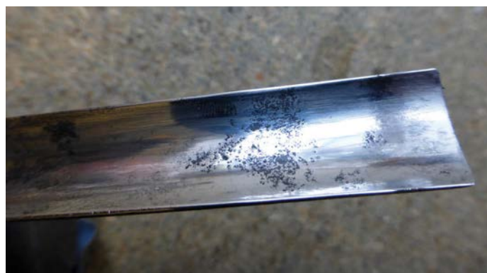
Even after cleaning and polishing pitting was evident
