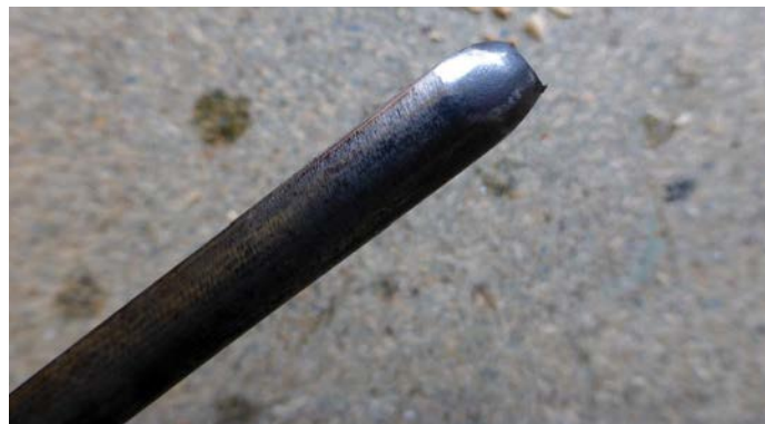
The back with the rust removed and the bevel formed
