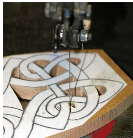
Carry out all drilling, sawing or background shaping before you start to shape the intersecting lines
