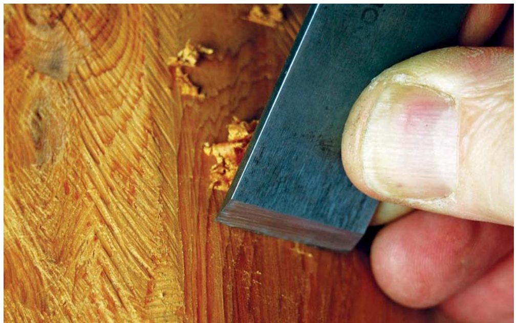
Sharpening a scraper as you would a carving tool gives a keener edge
