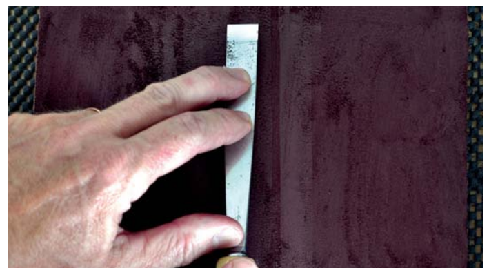
Place the tool at the far end of the strop and hold it at the precise angle of its bevel
