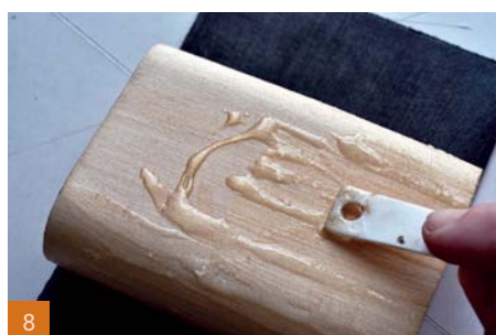
8 A strong and fast drying adhesive is a good choice for bonding the leather to the blocks
