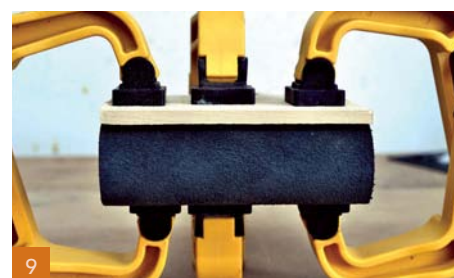
9 Place a thin strip of wood over the position where the leather joins itself and clamp it very tightly
