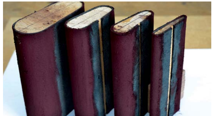
The slip strops only need the paste applied along the curved sides that come into contact with the gouges
