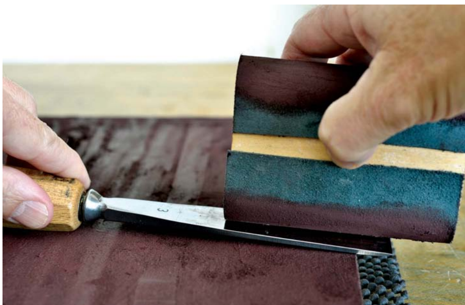
The tool to be stropped with the slip strop should always be placed firmly onto a surface and not done by holding it in the air
