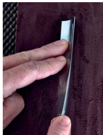
Place the gouge at the far end of the strop and hold it at the precise angle of the bevel on the cutting edge
