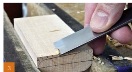
3 If you do not have a bandsaw, secure them safely in a woodworker's vice and carefully carve them back to the lines
