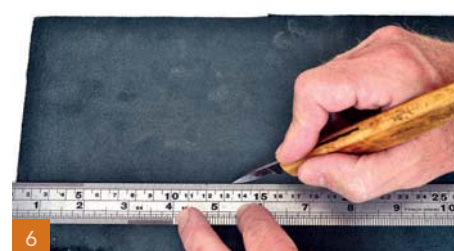
6 The leather for the sides of the strops can either be applied as one piece wrapped all of the way around them or two pieces
