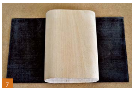
7 The leather must again be bonded with the suede side up
