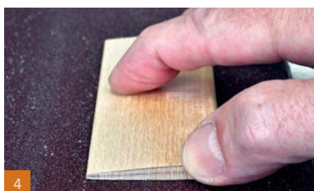
4 If you have a belt sander, carefully sand the excess wood back to the lines
