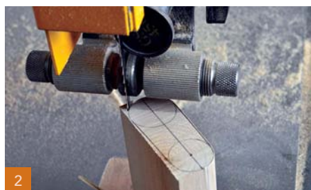
2 You have a choice of three different ways in which you can shape the blocks
