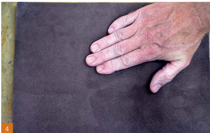
Carefully place the leather onto the wood and then smooth it out firmly, from the centre to the edges
