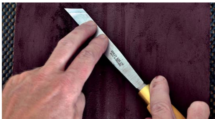
Place the tool at a parallel angle with the top edge of the strop, with the cutting edge in a horizontal position
