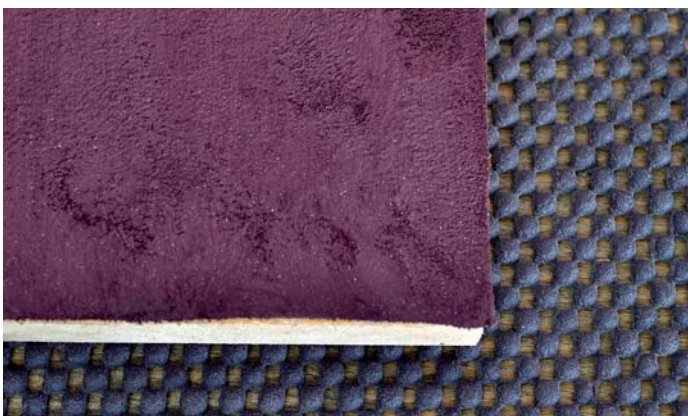
Ensure that the flat strop is either placed on top of a non-slip mat or carefully secured by some other means
