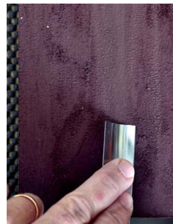
Place the tool at a parallel angle with the top edge of the strop, with the cutting edge in a horizontal position
