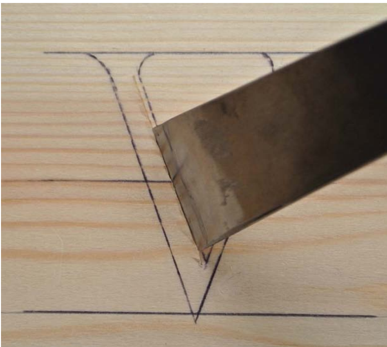
The first cut should be away from the weakness, slightly inside the line, with the second cut on the other side of the leg
