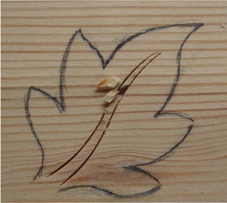
Stabbing each side of the stem will create a weakness, as will stabbing around the points of the leaf
