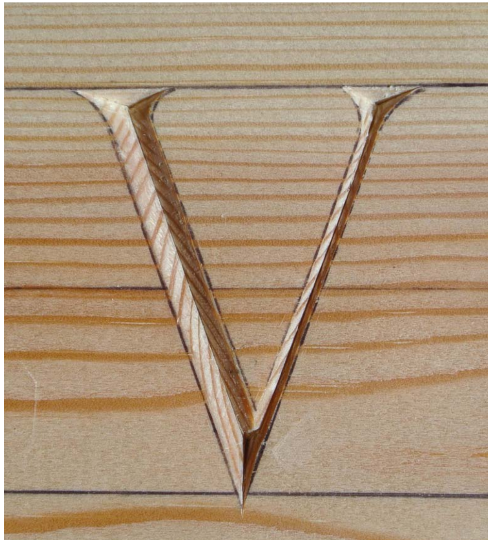
The finished 50mm high pine (Pinus spp.) letter with all the cuts at 60°, including the serifs
