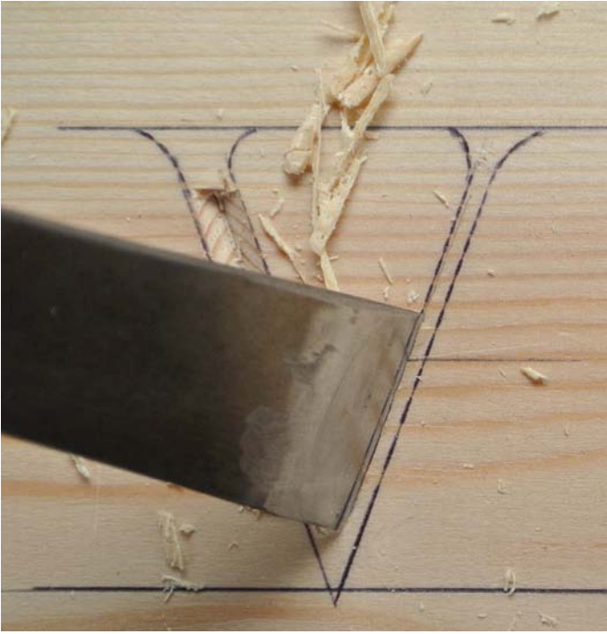
The third cut should be away from the weakness on the connecting leg, slightly inside the line, with the fourth cut on the other side of the leg
