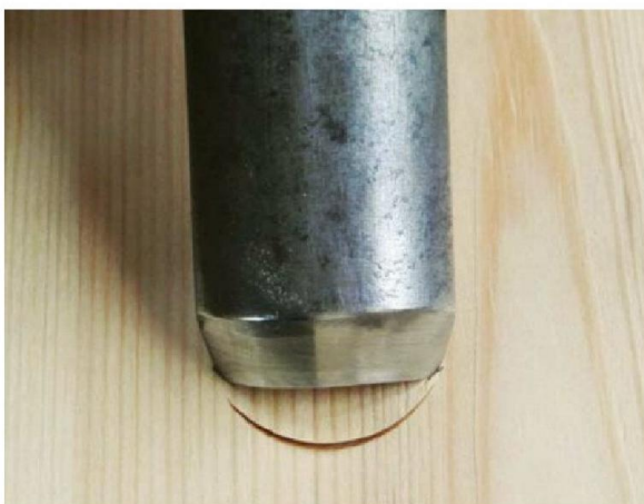
Only the outer curve may be cut with a square-ended cutting edge tool, as the corners of the cutting edge inhibit the inner cut
