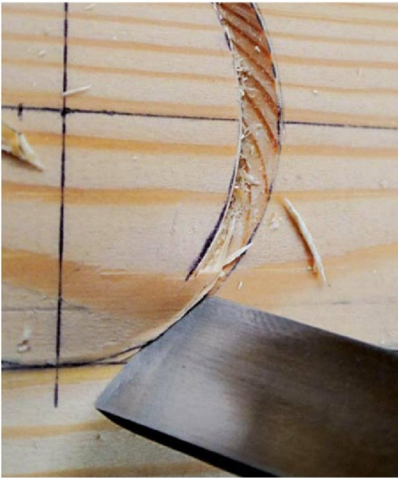
To straighten the curve, twist the handle while rolling the cutting edge to direct the cut through the line
