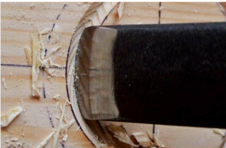
Cutting a smaller curve – 40mm high – inside the larger circle with the same chisel
