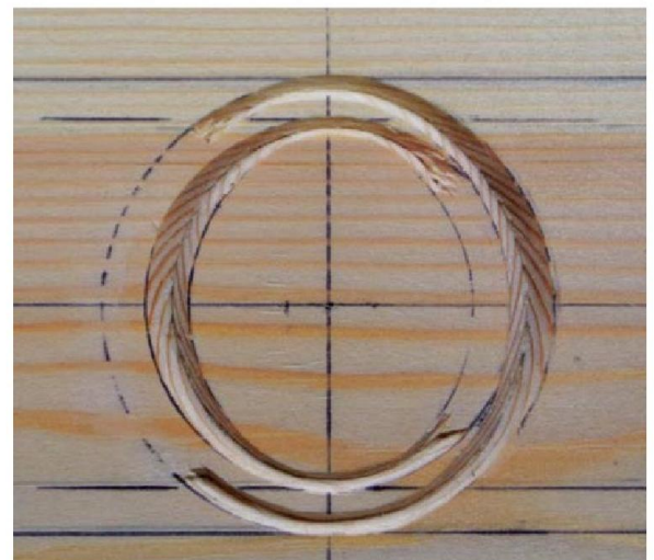
Illustrating parts of two different circles cut in an unsuitable soft pine with the same tool
