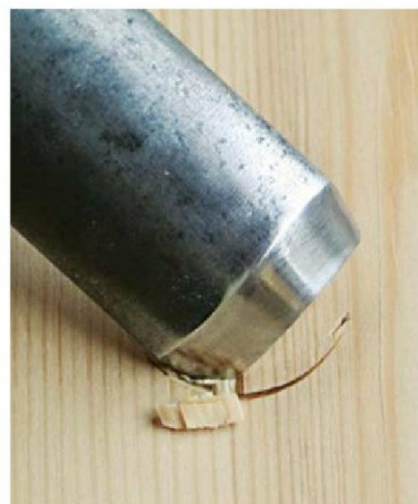
The inner curve cannot be cut with a square-ended cutting edge unless you 'chase the cut'
