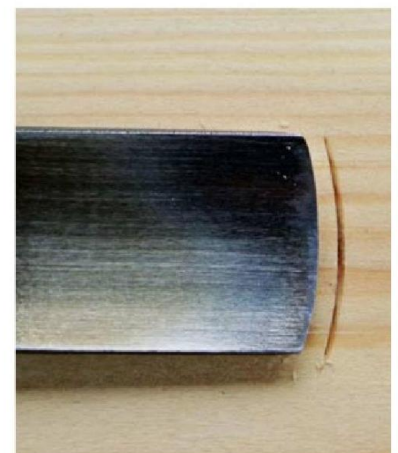
The bull-nose shape echoes the curved section of the tool without losing the corners
