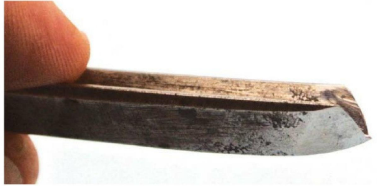
Side view illustrating the angled back cutting edge and a curved bevel
