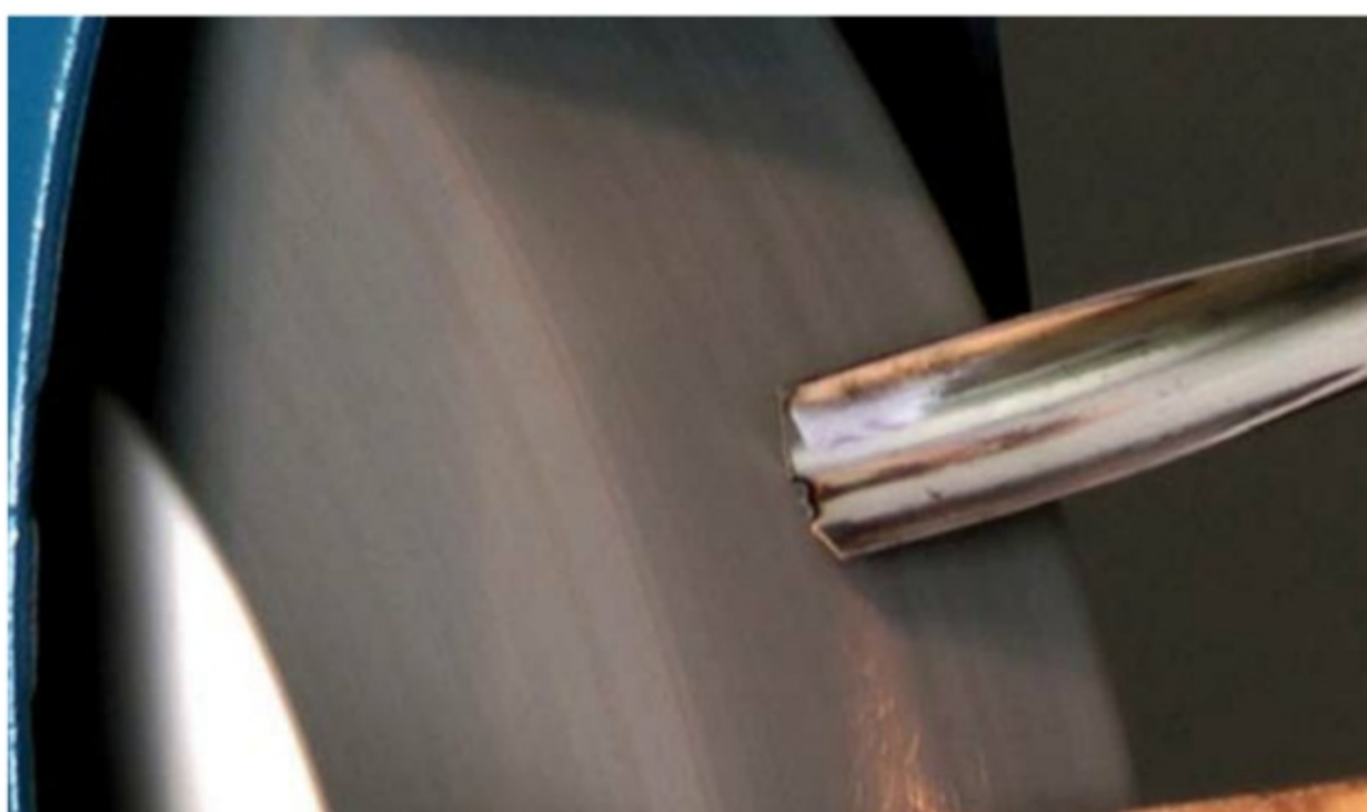
You offer up the bevel of your carving tool to the spinning wheel. All's going well, then before you can react, the cutting edge turns blue!
