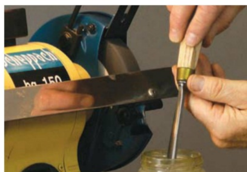
If the blade is warm, I dip the blade in the water and stir it about quickly
