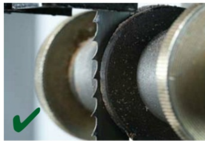
The correct setting will have your teeth proud of the side guides
