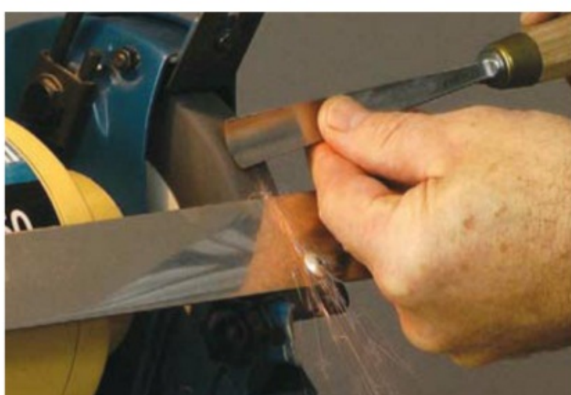
I hold the blade in my fingers, which in turn lie on the toolrest
