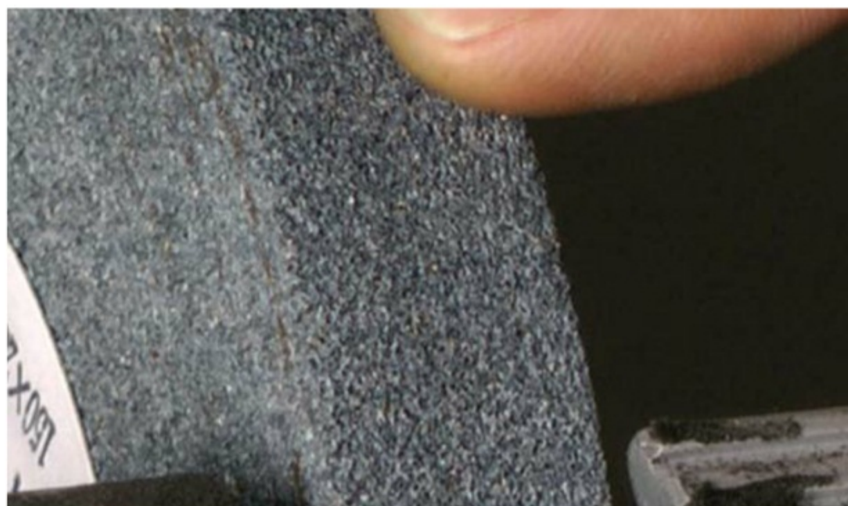
A finer wheel presents less air and more surface grit across the blade
