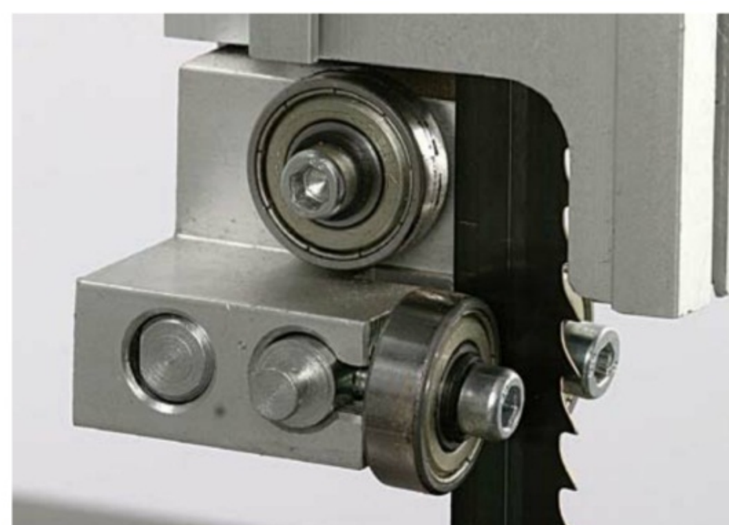
My preference is to have a thrust bearing running on edge
