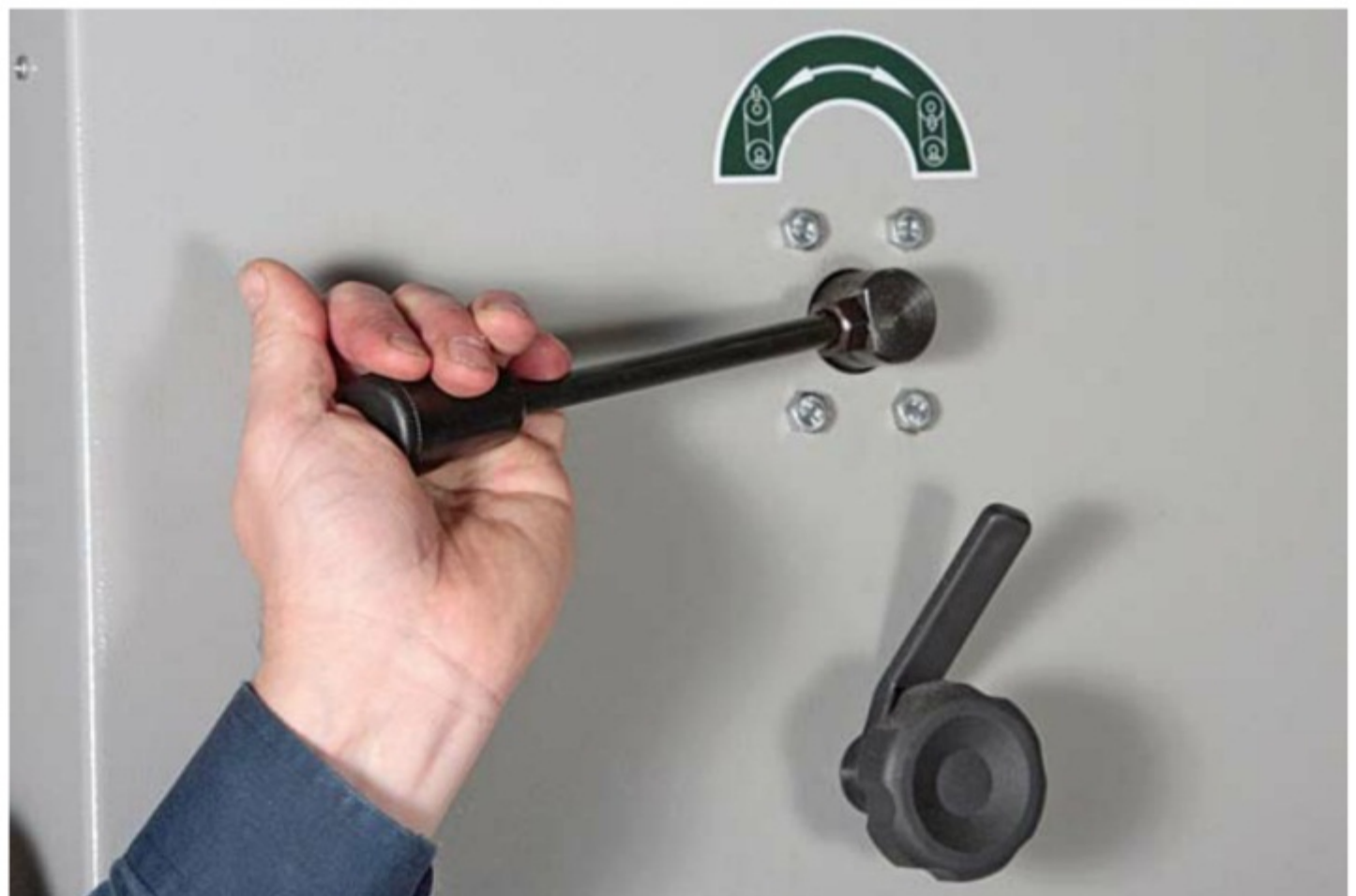
The new generation of bandsaws often come with a quick tension release mechanism
