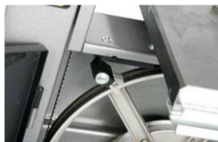
It's also important to make regular checks of the brushes in the lower case
