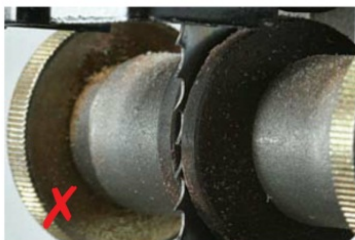
The position of these side bearings will soon render the blade useless as the teeth make contact with them
