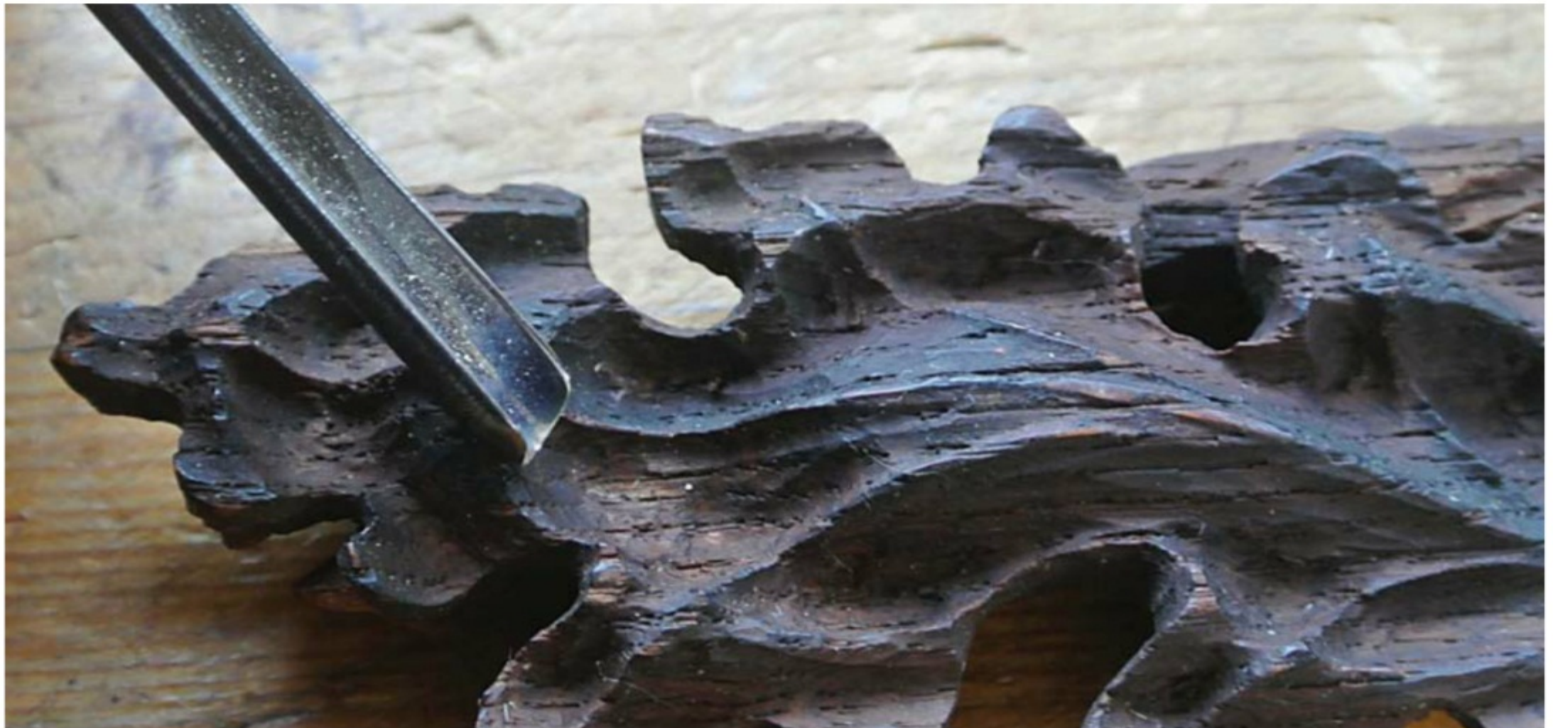
The angled cutting edge helps form deeper cuts as in Gothic leaves
