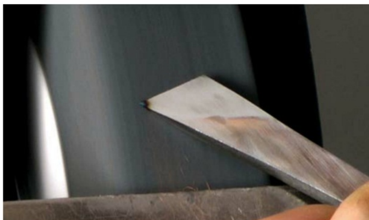
Bluing happens on corners and thin edges because the thinner the metal, the faster the rise in temperature
