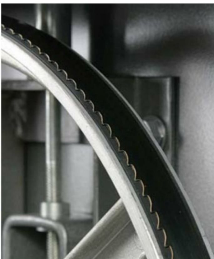
By tilting the top wheel backwards or forwards the blade can be tracked to run in the centre of the tyre
