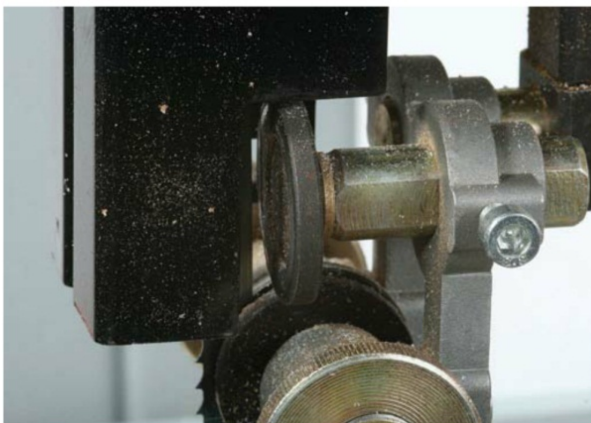
The most common type of thrust bearings are the ball race type – shown on the left – and hardened pads – shown in the photo on the right
