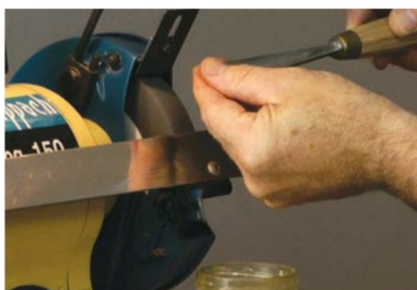
I frequently slide the blade back into my fingers and check the temperature
