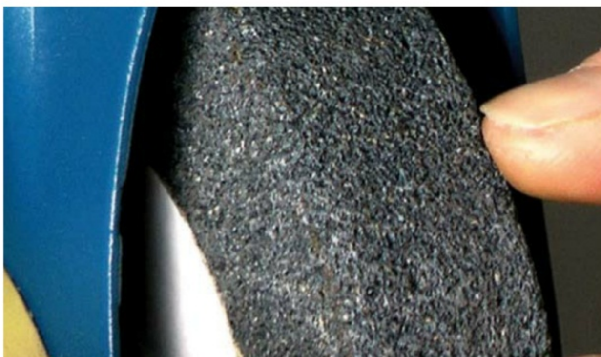
A coarser wheel presents more air and less surface grit across the blade
