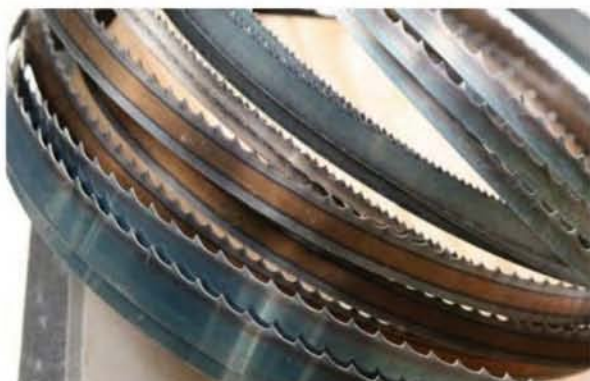
Blades with skip or hook teeth have fewer teeth per inch and for most woodcutting the common pitches are between 3-6tpi
