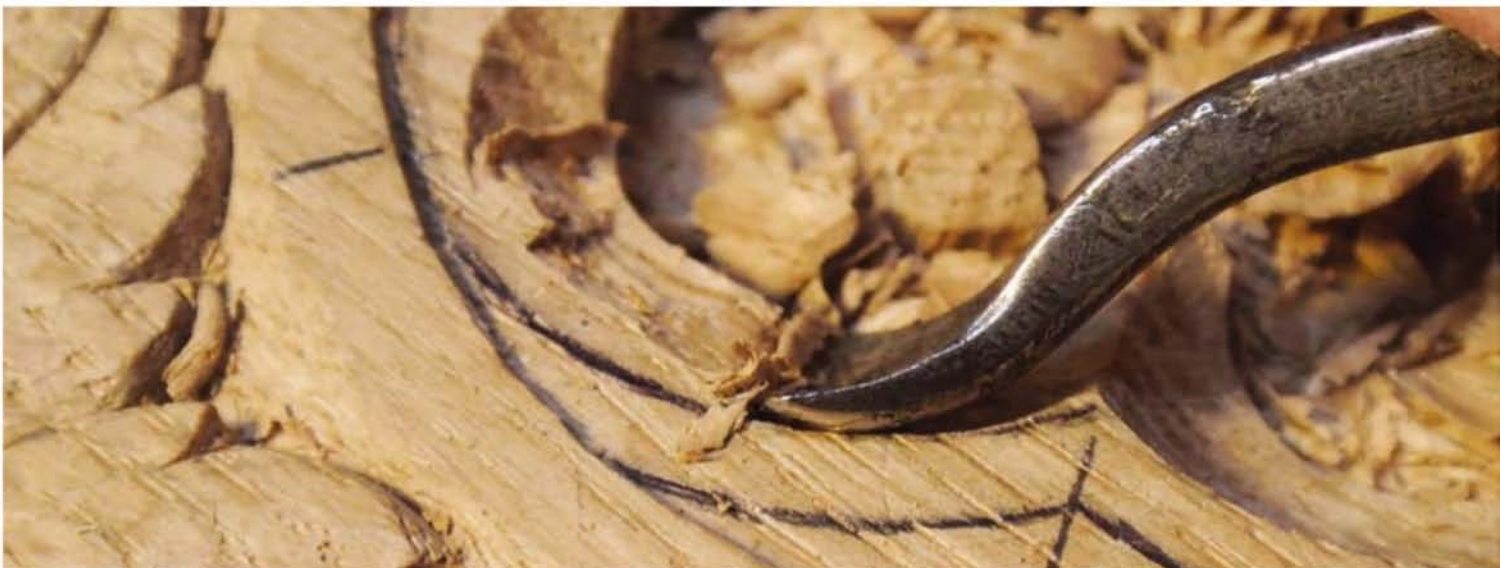
The hooked shape allows you to create hollows around tight inner curves
