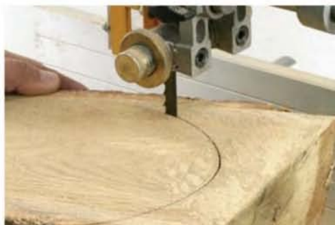
If you're cutting mainly curves, the radius of the smallest curve will determine the most suitable width of blade...
