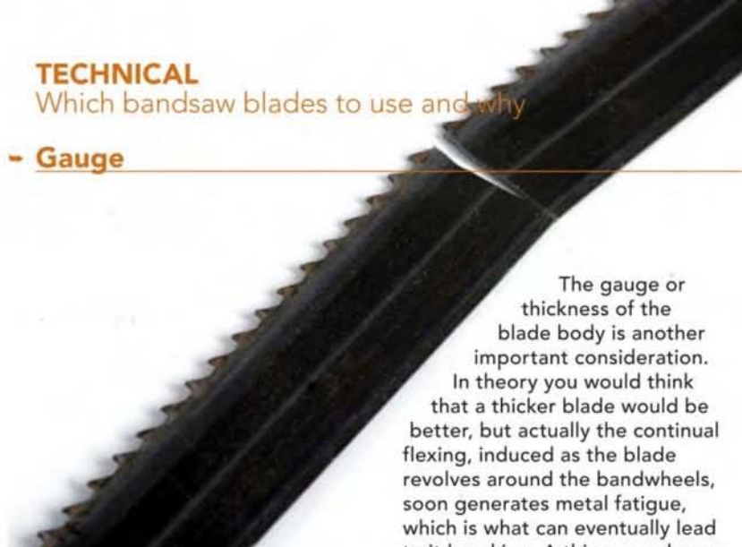
A broken blade caused by metal fatigue
