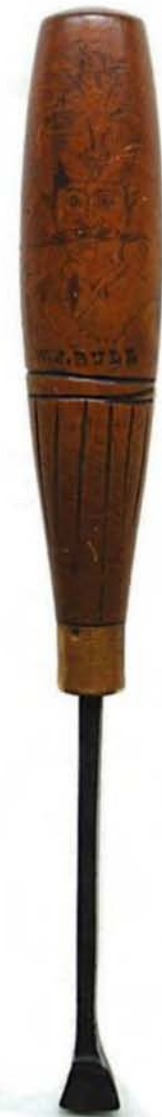
This tracery chisel shows the correct 'fish tail' shape. It originally belonged to the foreman woodcarver at the company I worked at, Mr. W. J. Bull – Bill Bull – who retired around 1960. His name is stamped on the handle together with a face etched in ink
