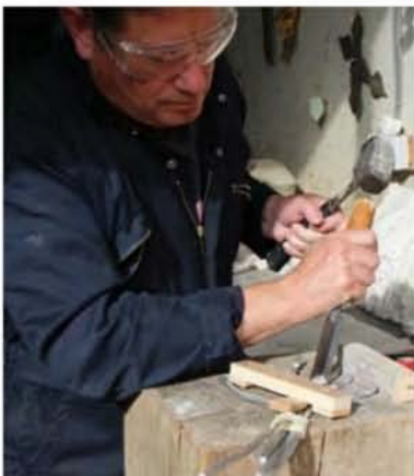
Using an old but relatively sharp wood chisel I chopped out 'V' sections to allow me to bend the digits at the required sharp angles
