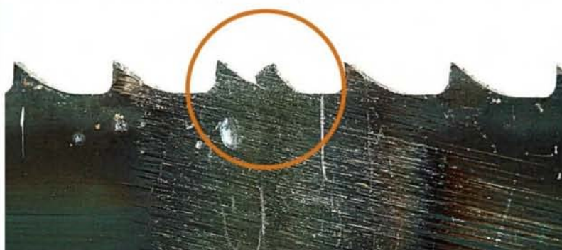
An irregular tooth pattern at the weld can result in a rough finish
