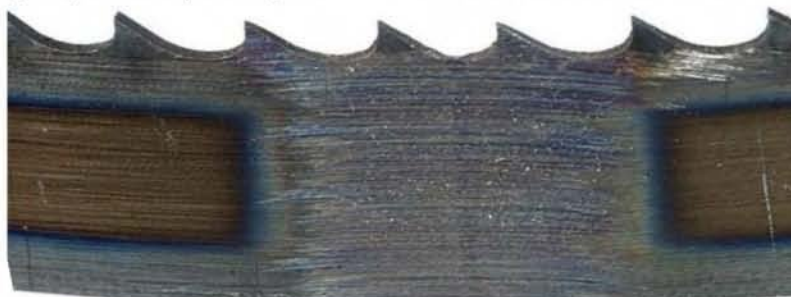
A quality blade can often be identified by the cleanliness of the weld. A uniform thickness and unbroken tooth pattern are good indicators
