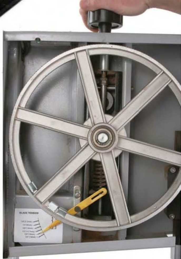
A thinner and more flexible blade will always last longer, and is easier to tension correctly without straining the tensioning mechanism on the saw
