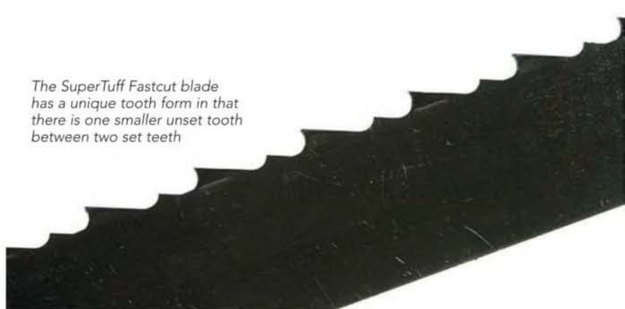
... they are also particularly good for resaw work as they have the least tendency to follow the grain
