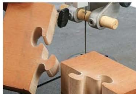
... an 1/8in blade with its wide kerf to width ratio allows you to cut really tight radii
