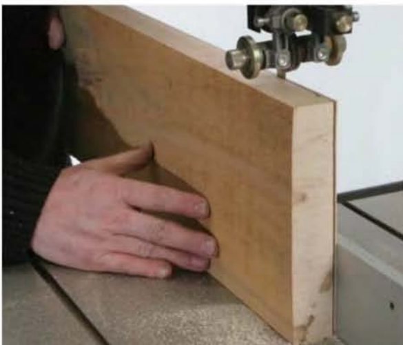
... they are also particularly good for resaw work as they have the least tendency to follow the grain
