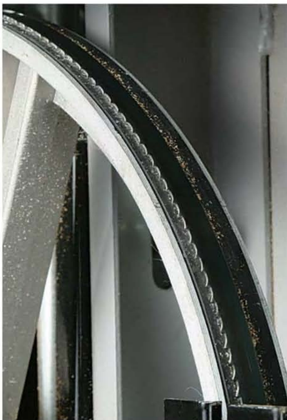
Blades with hardened teeth can be run in the middle of the bandwheel, which makes it much easier to set up
