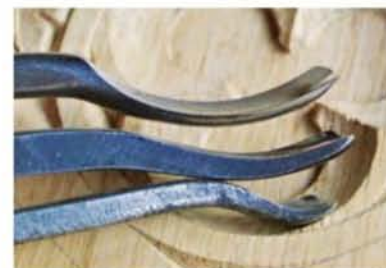
The traditional tracery chisel above fits the curve while the two more modern tools above it do not
