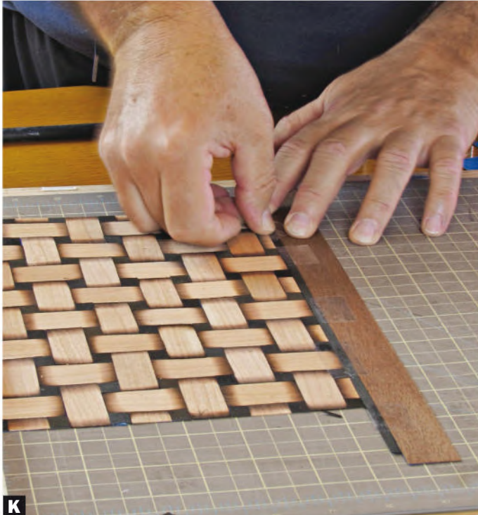
K Wrap the pattern. Use transparent tape to affix the black border strip to the frame strip. Then tape that assembly to the edge of the basket-weave panel.
