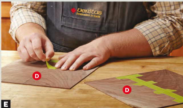
C A bit of light-colored earlywood adds interest. A blank similar to the rear piece yielded these two pieces with an accent at one corner on the first resaw.
