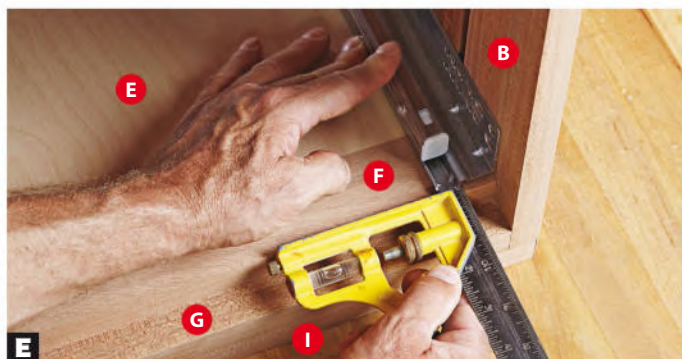
E Position the slides. To keep the panels loose, screw the slides only to the stiles (B, C). You may have to drill new mounting holes through the slides.
