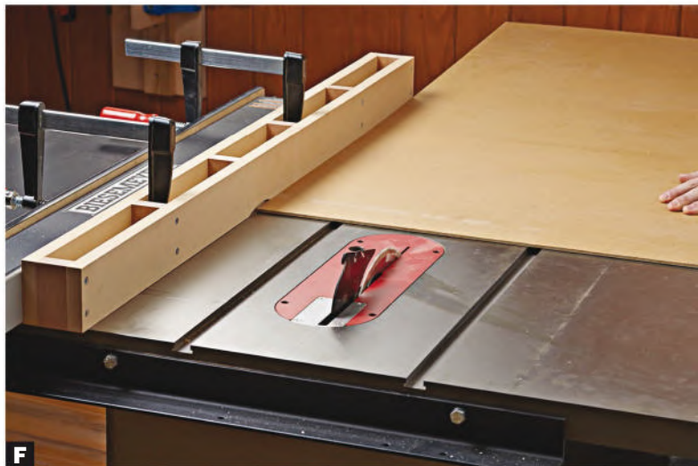
F Off to a good start. When dealing with long or awkward stock, such as sheet goods, clamp the auxiliary fence so it overhangs the front edge of the tablesaw. This will help stabilize the stock before it reaches the blade.
