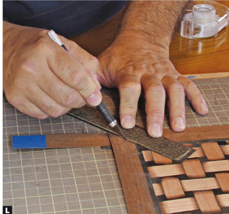
L Slice perfect miters. Cut diagonally with several light passes to miter each corner of the border.
