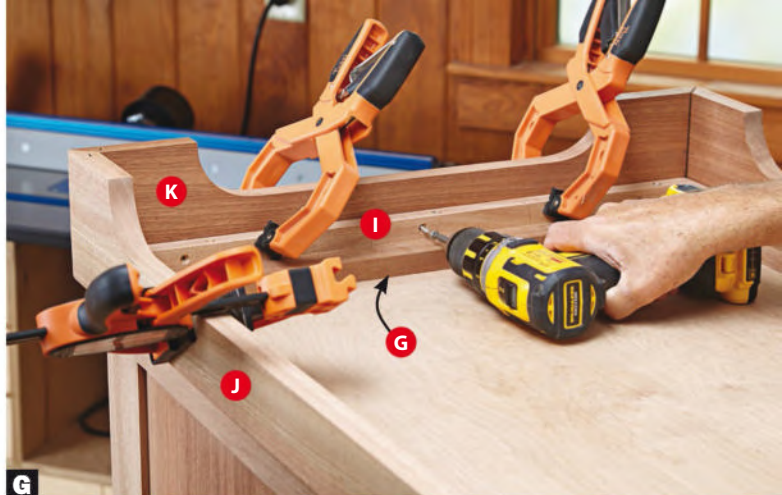
F Attach the side trim (J) first, above. Place the top edge 1\frac{1}{8} " above the bottom of the cleat (H). Then, glue and biscuit the miter-cut ends and attach the base end trim (K), above.
