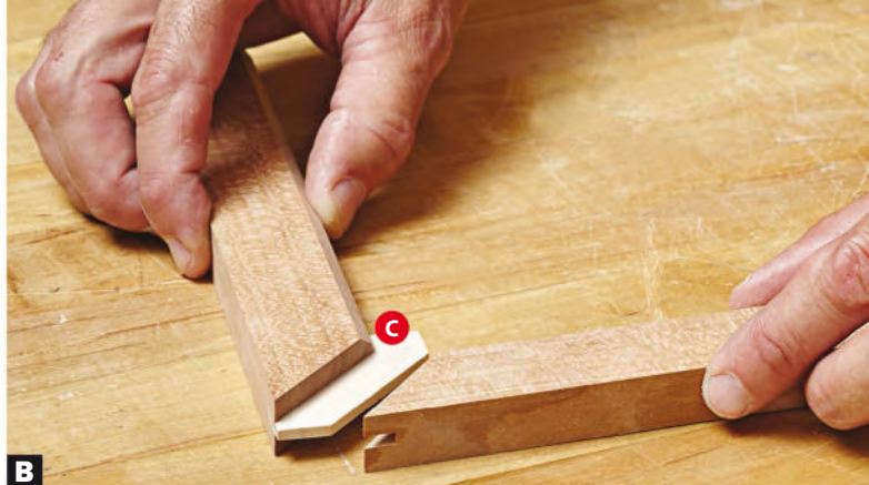
B Apply glue to the groove and rub the spline back and forth a couple of times. Make sure the spline's outer tip sits flush to the frame edges.
