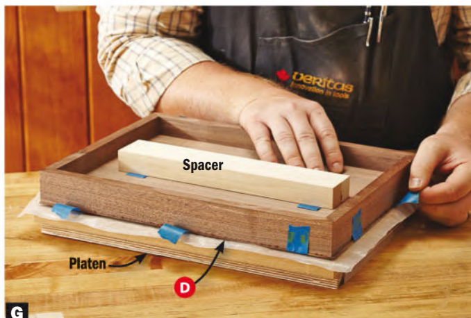
G Reuse your veneer press. Tape the veneer to the lid with \frac{1}{16} " overhanging on all sides. A scrap spacer \frac{1}{32} " thicker than the lid depth distributes pressure to the center of the lid when you apply the top plywood platens. Place strips of tape below the spacer if you need to elevate it slightly to allow the plywood to make contact.
