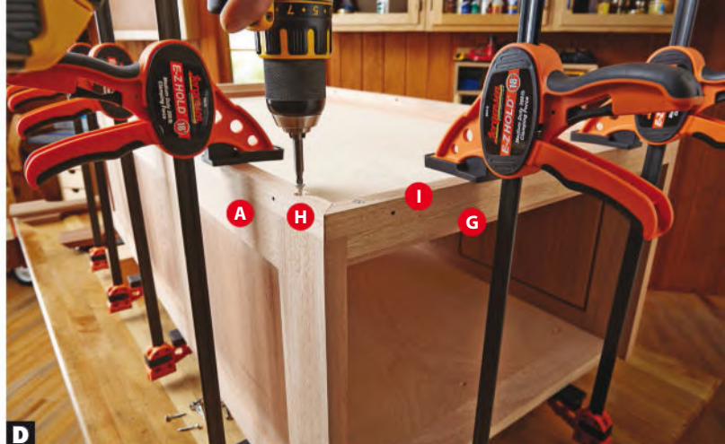
D Install the base cleats (H, I). Keep the outer faces of the cleats flush with the rails (A) and bottom supports (G) as you attach them to the carcass.
