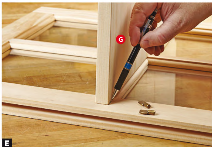
E Mark the shelf-pin locations. Use a movable shelf (G), centered on the window muntin, as an aid in locating holes for shelf pins.
