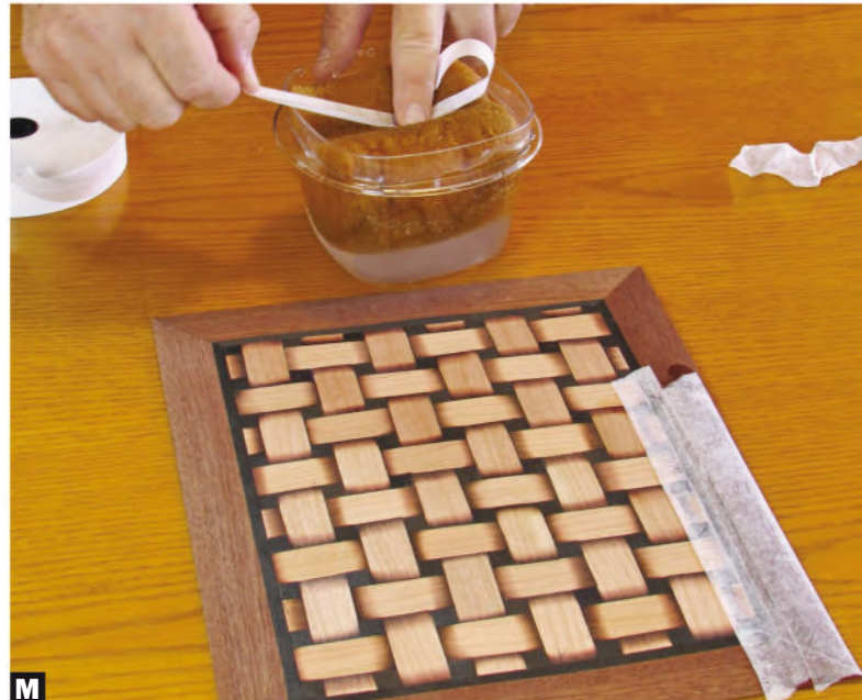
M Layer on the veneer tape. Run the tape over a wet sponge to moisten it, then apply it to the face of the pattern. The veneer tape shrinks as it dries, tightly pulling the joints together.
