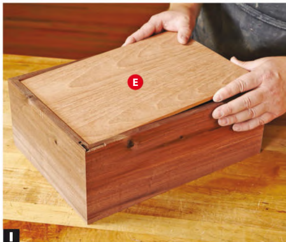
I Cut the liners to slide in. You'll remove them from the lid and box before applying a finish to the inside of the humidor.
