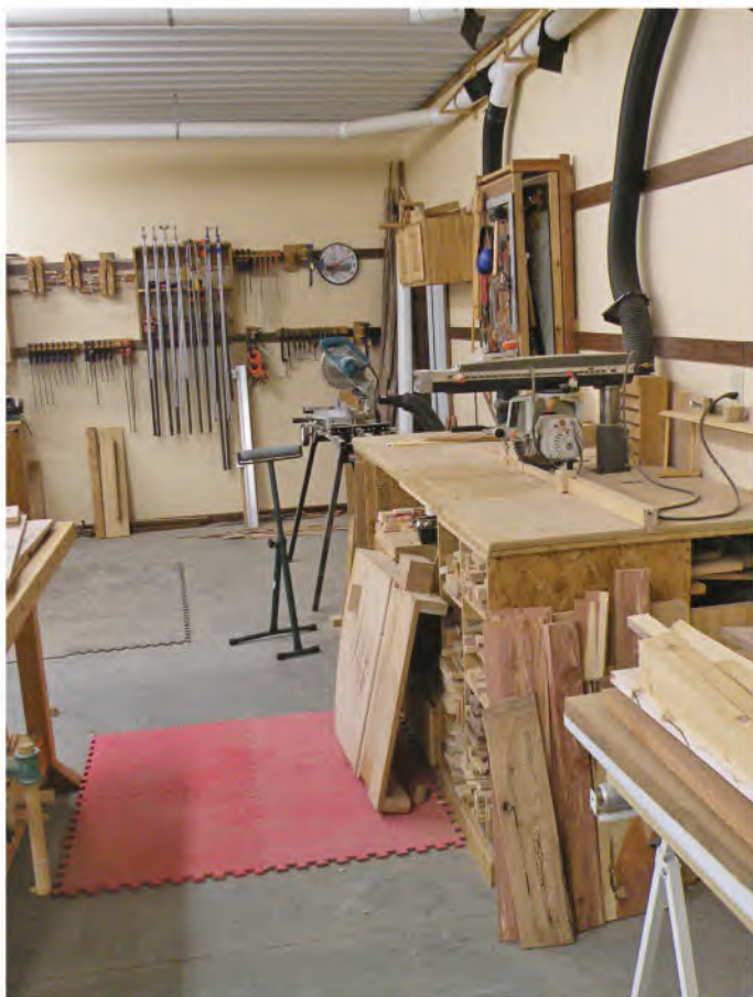
Rick mounted French cleats along each wall to make the installation of storage racks and cabinetry simple and very adjustable.
