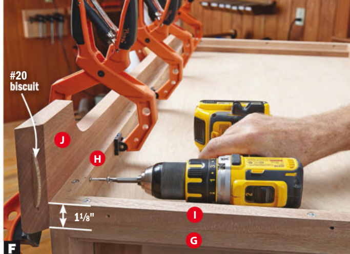
F Attach the side trim (J) first, above. Place the top edge 1\frac{1}{8} " above the bottom of the cleat (H). Then, glue and biscuit the miter-cut ends and attach the base end trim (K), above.
