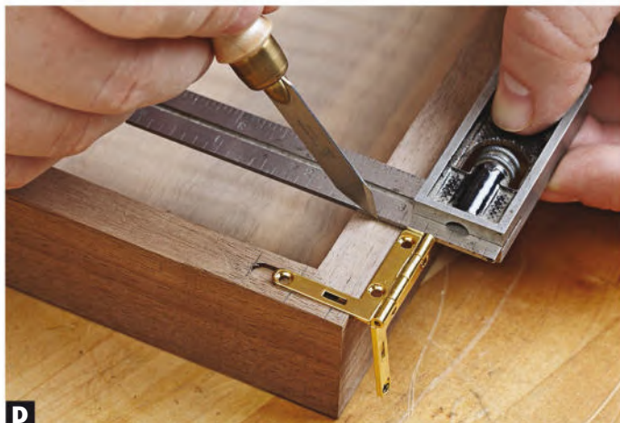
D With a leaf snug in the recess, and the edge of the back leg against the back of the lid, mark the length of the leg.
