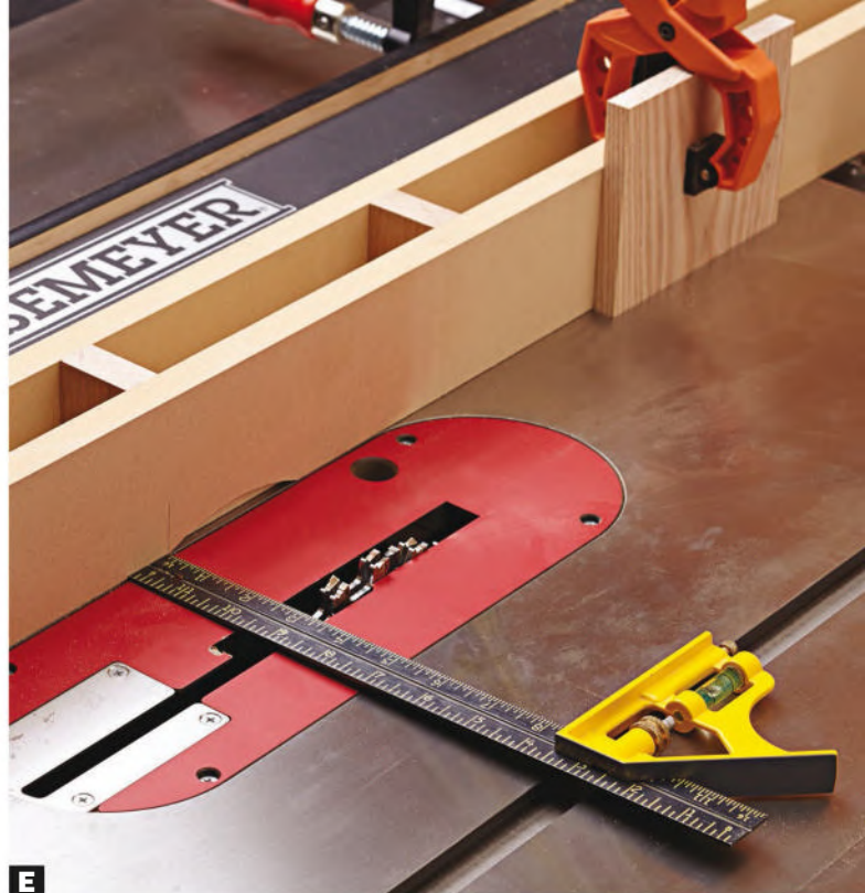
E Measure and mark your setback. Need a 12"-long stopped groove? Clamp a stopblock to your fence 12" from the front-most tooth of the blade.
