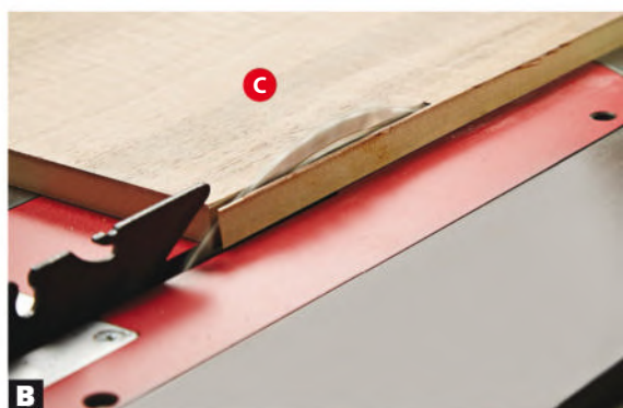
Trim both edges and ends to bring the box top and bottom to final size. If veneer overhangs both edges, sand or plane one edge flat first, then run that edge against the rip fence.
