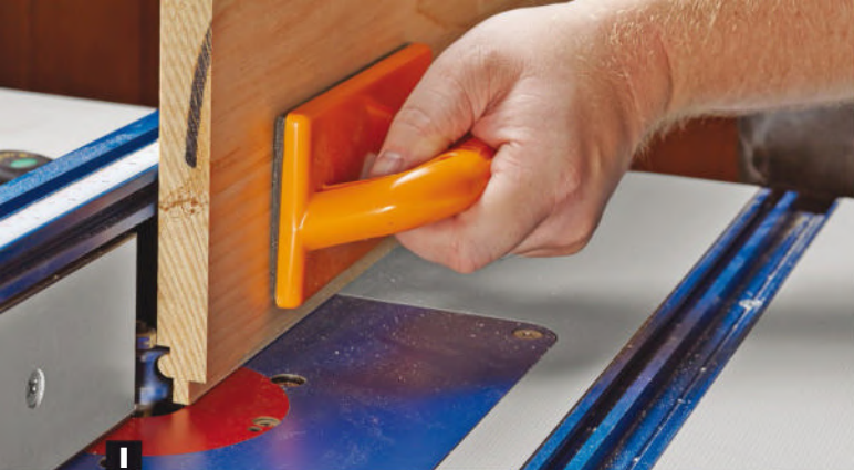
I A bead at every tongue. Adjust the height of the beading bit to cut a full bead on the face side of each slat at the base of every tongue.
