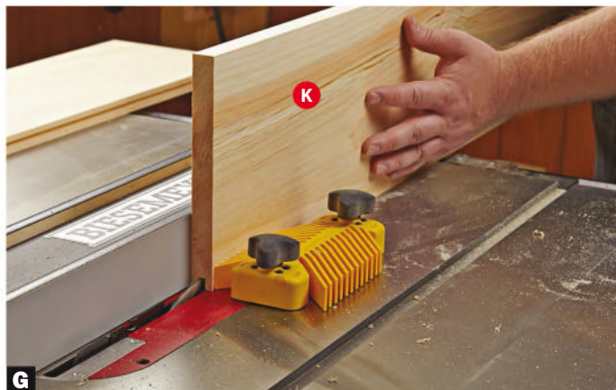
G Get in the groove. Cut the 1/4" groove by making two passes over a full-kerf blade raised 3/8" high. Place opposite board faces against the fence to ensure a centered cut.
