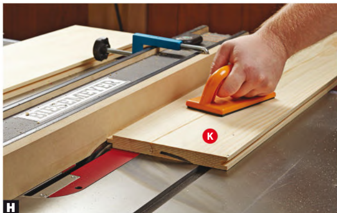
H Cut a tongue to match. Mount an auxiliary face to your tablesaw fence and adjust it so the dado blade cuts a 3/8"-long tongue. Raise the blade in small increments, flipping the board with every cut, until the tongue snugly fits a groove.
