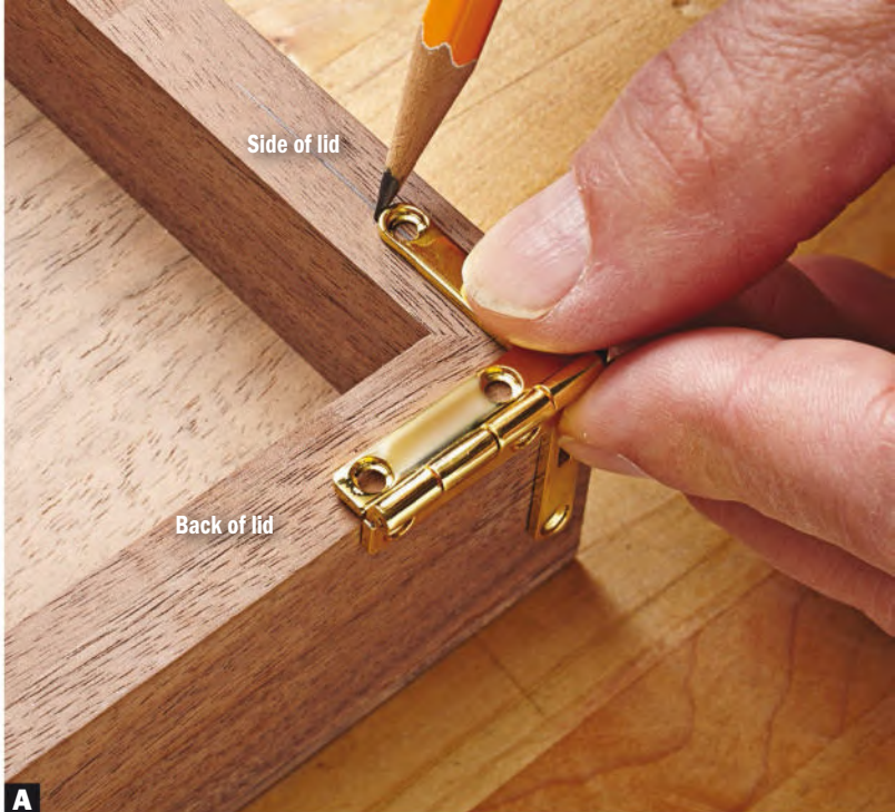
A Center a hinge on the thickness of mating corners of the lid and box, with one leaf pressed against the back face of the box or lid. Mark the leaf length on the mating edges.
