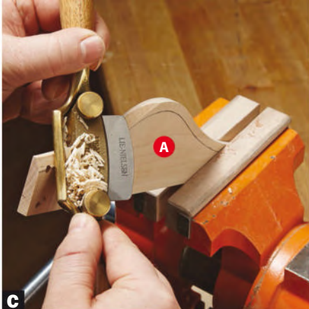
C Shape the sides' top edges. Draw a line \frac{1}{4} " from the sides' top edges with a pencil, following their curves. Use a spokeshave to chamfer to that line. (The edge is too narrow to use a router bit.)
