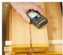
► A handheld moisture meter ($80-$400) proves a worthy investment for gauging wood moisture levels at the store and at home.
