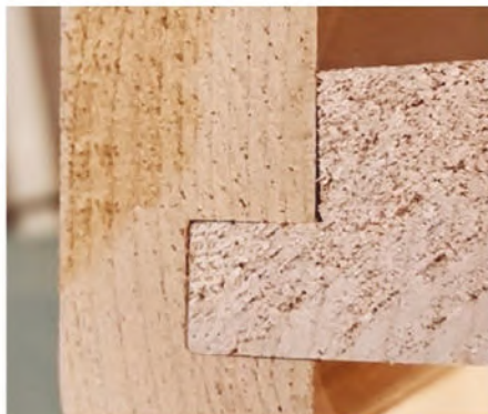
Oops. Unfortunately I put the rabbet on the wrong side of the figured panel, leaving a stub protruding.
