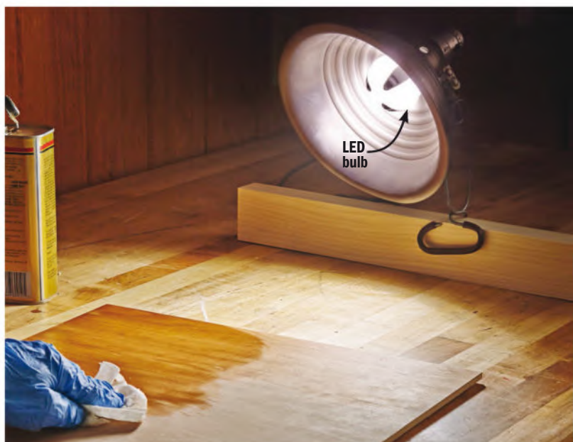
A spring-loaded clamp grips an edge to hold the light where it's needed. A cool-burning CFL or LED keeps the shade cool to the touch.
