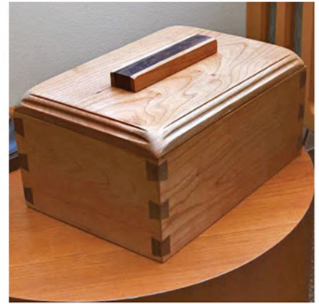
What tear-out? Though unintentional, the rounded lid corners draw your eye to the dovetails, enhancing them.
