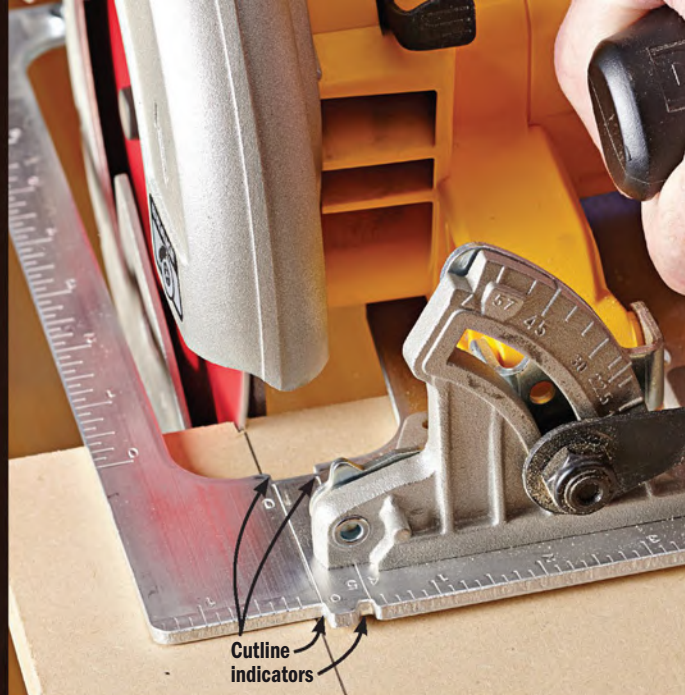
Track the line. Cutline indicators on the front and inside edges of DeWalt's footplate help you start a cut and then keep the blade cutting along a straight line.
