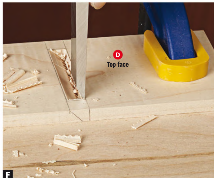
Make the mouth. Select a drill bit sized to fit between the marked lines on the sole (D) and drill out the waste. Then, flip the sole to its top face and, using a wide chisel, clean up the mouth edges.
