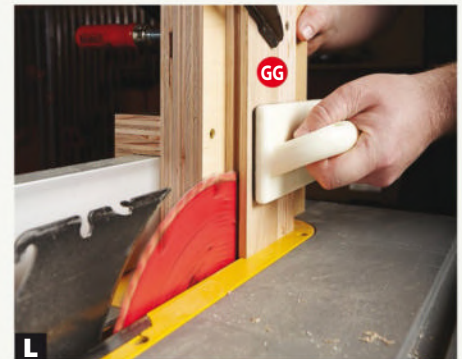
L Cut mortises in the lower stiles. For best results, the jig must slide smoothly over the rip fence. Clamp the workpiece to the jig.
