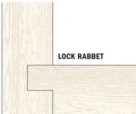
What a lock rabbet should look like. The corner joint for a blanket chest I built should have looked like this.
