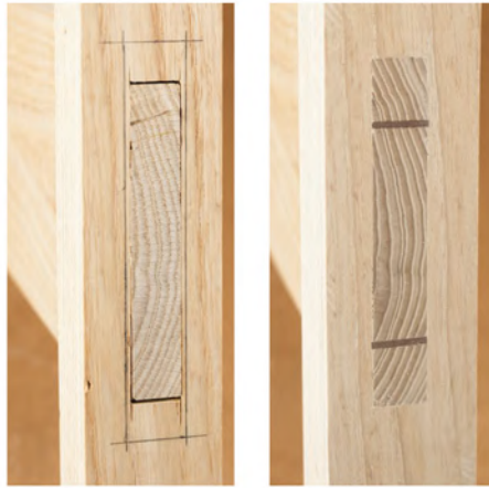
The repair for this too-loose tenon—wedges—provides an opportunity for a pop of contrasting wood that improves the final look.
