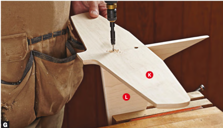
G Stabilize the stabilizers. With the vertical stabilizer (L) held in your vise, drill countersunk pilot holes through the horizontal stabilizer, careful to keep the two pieces square and perpendicular to each other.
