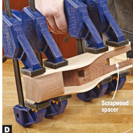
D Clamp up the body. With the bottoms of the infills (B, C) flush with the bottom edges of the sides (A), glue and clamp the assembly together. Insert a scrapwood spacer in the tote (E) slot to avoid damage from the clamping pressure.
