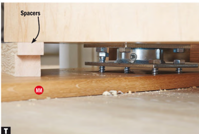
T Tighten the lag screws. Use a box wrench or open-end wrench and be patient. It's a tight area to work in so you'll only get small turns of the wrench.
