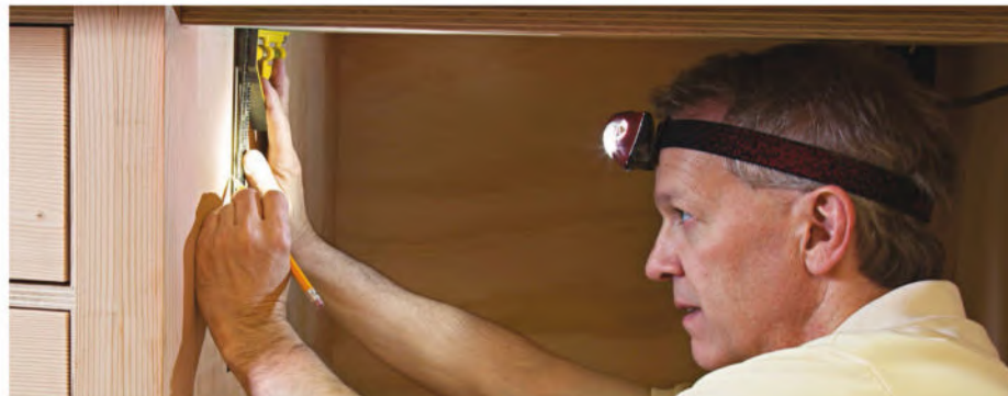
Free your hands. A pivoting multi-LED fixture with an elastic strap (find them at home centers and camping stores) can be adjusted from bright to super-bright.
