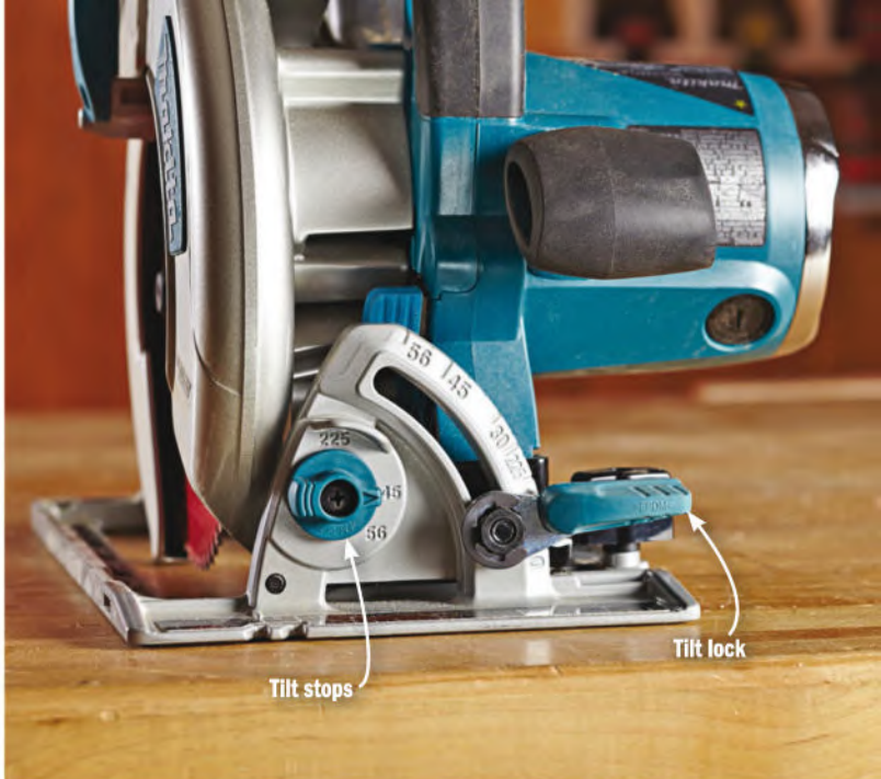
Easy tilting. Makita's footplate tilts to 56°, and has stops for the more commonly used 22½° and 45° cuts.
