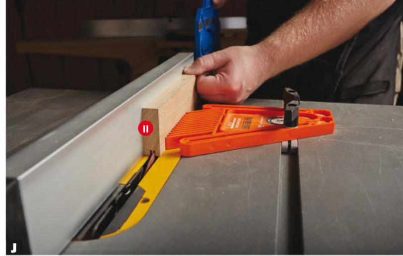
Center a groove. Attach a featherboard in front of the blade, and make a pass with each face against the fence to center a groove in the lower door rails and stiles.
