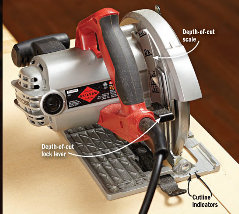
Back-door help. The SkilSaw Sidewinder also has cutline indicators at the rear edge of the footplate to help you stay on course as you complete a cut.
