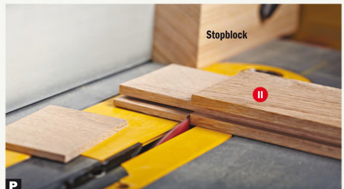
P Complete the tenons. A stopblock clamped to the rip fence establishes the tenon length and provides clearance for waste to move away from the blade.
