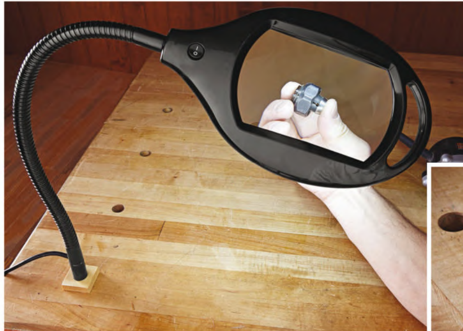
Ready for your close-up? A shop-made bench dog (right) allows for positioning the magnifier in any doghole on your bench. Or secure the fixture to the edge of a benchtop, shelf, or tool with the provided clamp base (not shown).
