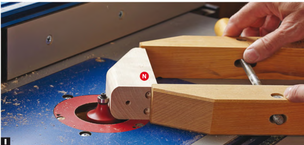
I A handscrew protects fingers. When routing the round-overs on the engines (N), hold the parts with a handscrew.
