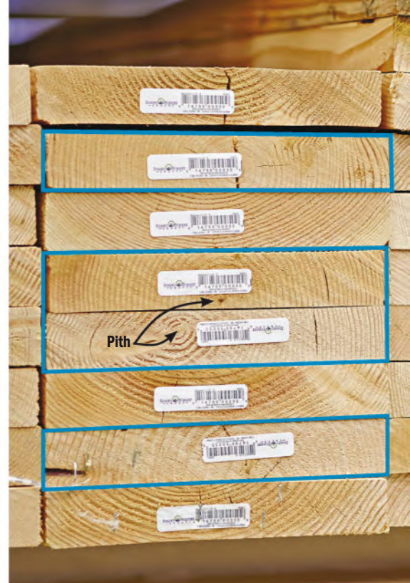
Good grain awaits. Most of these 2x12s could prove pesky to work with, but the highlighted ones, with quartersawn grain (minus the pith), would make for stable project lumber.
