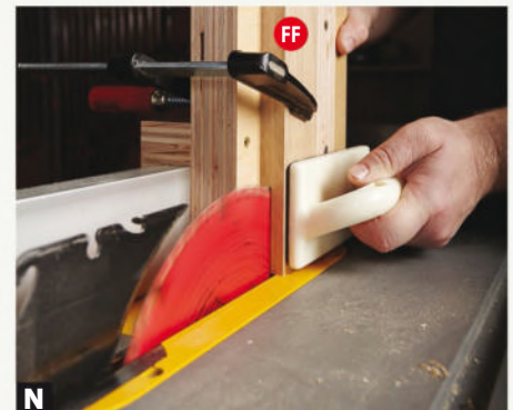
M Reset for the upper door stiles. Using the rails for the upper doors as gauges, set the blade height to match the full width of the rails, then cut the mortises as you did on the lower stiles.
