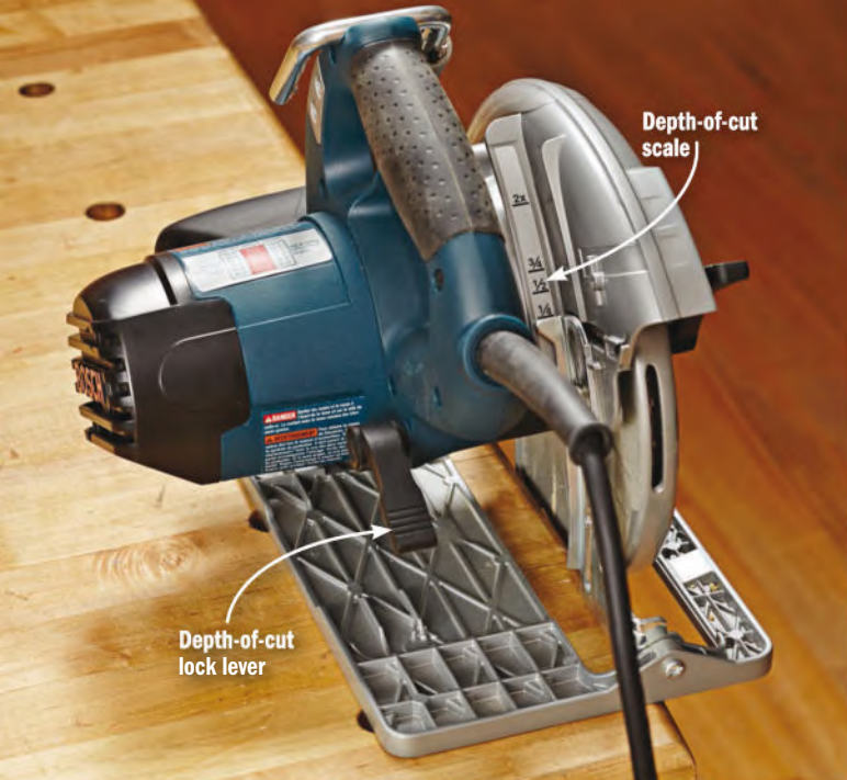
Quick lift. Setting the cutting depth on the Bosch saw is easy because the lever is easily accessible and the scale marked in common board thicknesses.
