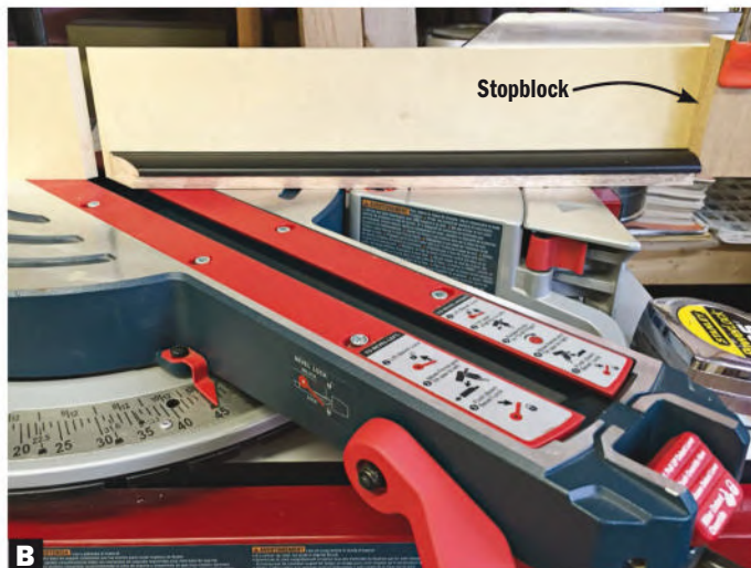
B Start with a stopblock. Clamp the stopblock in position to provide just a bit of extra length on the workpiece. I allow about \frac{1}{4} ".
