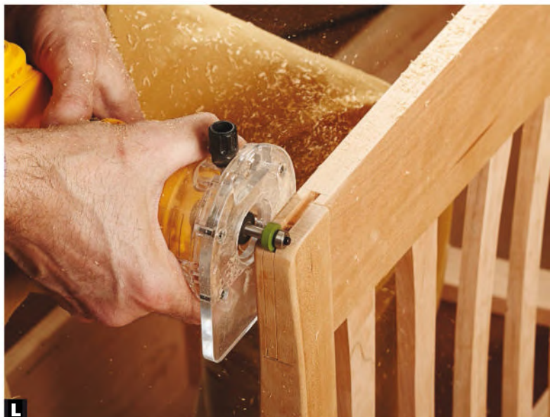
L Rout carefully. Mount a \frac{1}{4} " slot-cutting bit in a trim router and cut \frac{1}{8} "-deep grooves between the marks, steadying the router against your leg. Chisel the ends of the grooves square.
