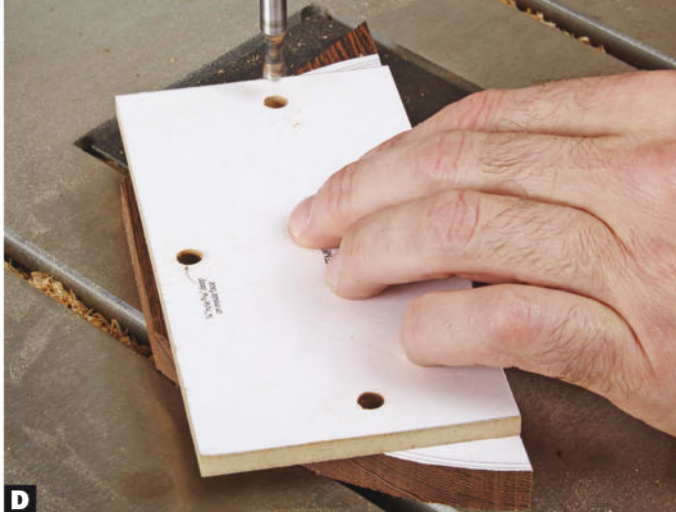
D One template does it all. By using the same template to drill the box sides and legs (shown here under the template), the holes will always align.
