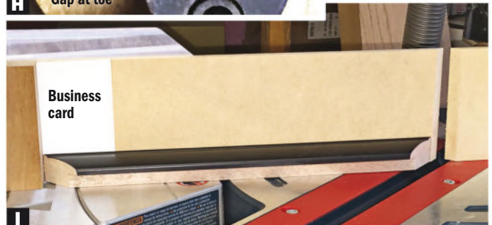
I Fix the toe. Cutting more of the heel than the toe is done the same way, with the sticky note or business card placed between the fence and the far end of the mitered stock.
