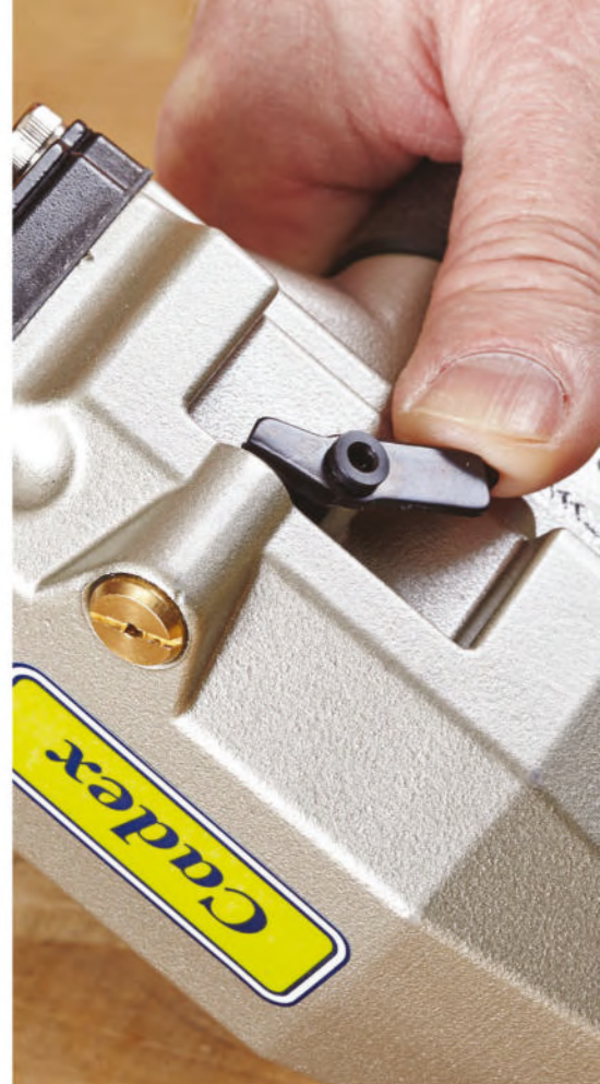
Give it a blast. To blow air through the Cadex nozzle, push the spring-loaded lever.
