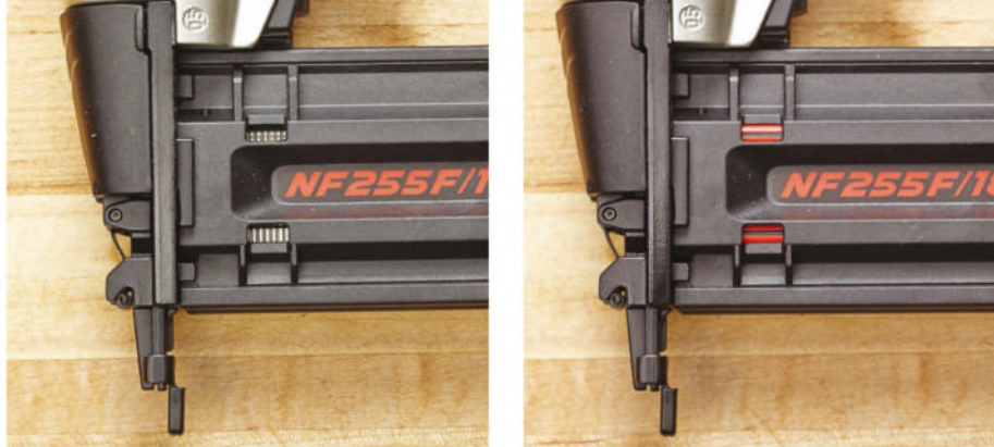
Window warning. The view window on the Max nailer shows plenty of brads remaining (left), and the red indicator in that window calls for a refill (right).
