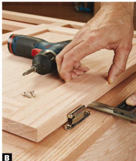
B Four points define a door location. Using a combination square, measure near the top and bottom of the door to ensure parallel. Repeat using the face-frame rail.
