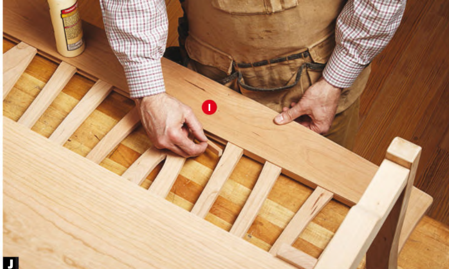
J Fill the grooves. Rest the bench on its back, then cut and glue in place filler segments to fit between each slat. To minimize glue squeeze-out, apply glue only to the face of the filler that contacts the bottom of the groove.
