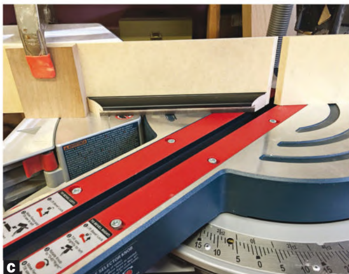
C Fine-tune your length. This is where that extra \frac{1}{4} " length comes in handy. You can now dial in the exact cut on one length of molding and use the stopblock so the second piece matches it.
