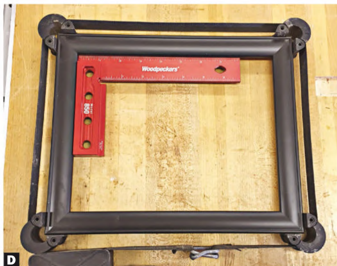
D Join the band. A band clamp is ideal for assembling a frame. Turning the handle cinches up the band and spreads pressure equally to each corner clamp.
