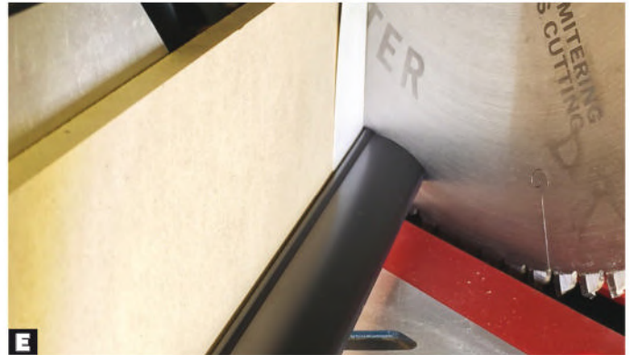
E Avoid the teeth to shave a whisker. With the saw off and the blade held down, slide the edge of the mitered molding against the blade body (not the teeth). While holding the molding in place, raise the blade, turn on the saw and cut the molding's edge. The amount of material removed equals the offset of the blade's teeth from the body of the blade.
