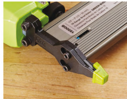
Tool needed. Grex's nailer requires a hex wrench (not included) to open the nose and free a jammed nail.
