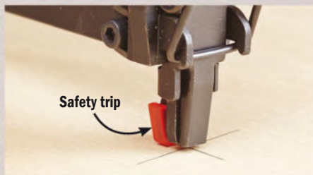
Better. Senco's rear-mounted safety trip allows good sightlines from the front, but side-to-side is still a bit iffy.
