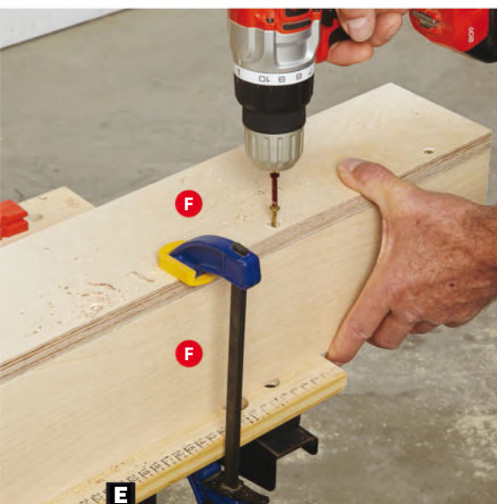
E Get a leg up on your bench. Align and clamp one leg side (F) on top of another on a worksurface with the edges and ends flush. Drill, countersink, glue, and screw them together.
