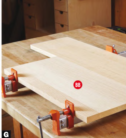
G Glue up; don't cut down. Rather than glue up a rectangular panel for the side table tops/bottoms (BB) then cut it to shape, glue together two smaller panels to form the cutout.
