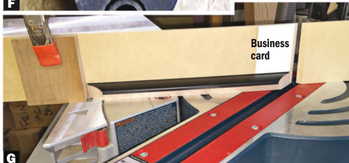
G Fix the heel. To trim more from the toe of the miter than the heel, place a sticky note or business card shim between the fence and the end of the workpiece nearest the blade.
