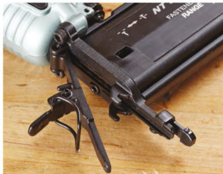
Easy open. Tool-free latches, shown here on the Hitachi, help you clear nail jams quickly.
