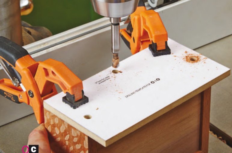
C A template ensures consistency. Whether you're making one box or dozens, guarantee accurate hole placement and depth by using a drilling template and a drill press.
