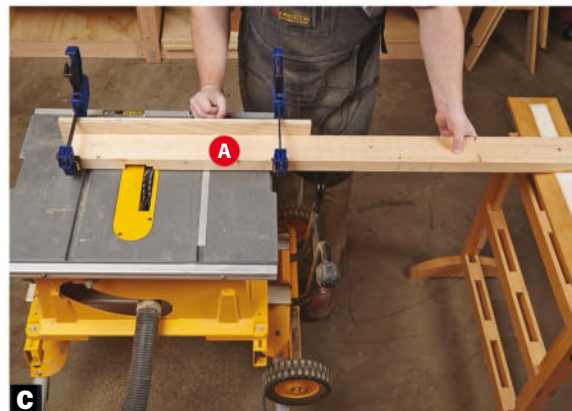
C Handle long parts easily. To steady the back uprights (A), set up a support to the side of the saw and clamp the workpiece to a miter-gauge extension.
