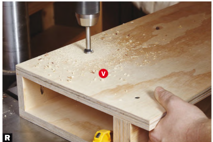
R Drill dowel holes. Drill \frac{1}{2} "-deep holes on the marks to accept \frac{3}{4} " dowels. Using the drill press ensures perpendicular holes so the dowels will drop into the dogholes easily.
