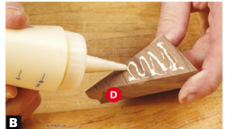
B Don't overdo the glue. Limit yourself to a thin layer of glue to ensure that the alignment lines aren't obscured and the block doesn't float during clamp-up.
