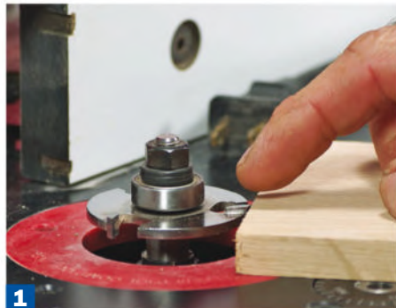
1 Set the height of the slot cutter so the top of the cutter is flush with the top of your test material.
