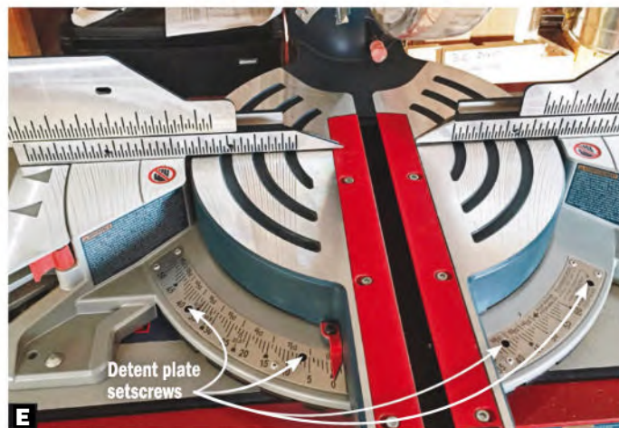
E Adjusting a fixed fence. Loosen the setscrews found on each side of the miter scale to fine-tune the angle of the blade to the fence.
