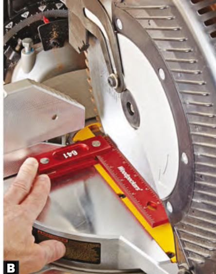
B Square the fence to the blade. Place the square's handle against the fence and check for a gap between the square's blade and the plate (not the teeth) of the saw blade.
