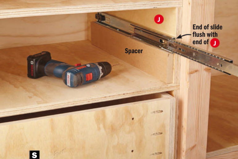
S Mount drawer slides easily. Rest a drawer slide on a spacer and secure the slide with two screws in the horizontal slots to allow for adjustment. Repeat on the other side.
