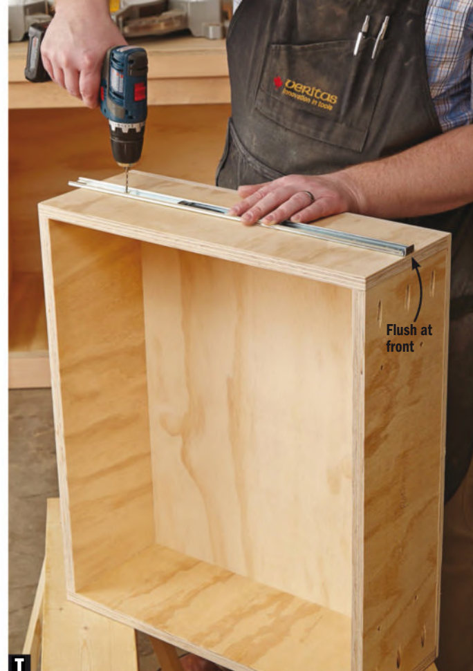
T Screw on the drawer half. Align the drawer half of the slide flush with the front of the box and centered on the drawer height.
