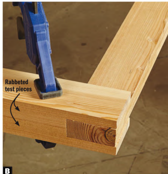
B Two rabbets make an open mortise. Sandwich the two test pieces together with the rabbets facing each other; a cutoff from the rails (C) should fit snugly in the resulting mortise.
