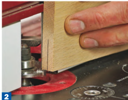
2 Position the fence for a 1/4"-deep cut (one-half the 1/2" material thickness).
