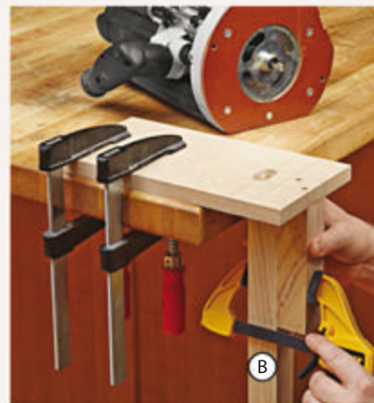
After cutting the first mortise, slide the workpiece down to cut the second.
