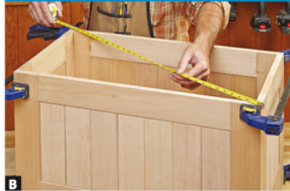
B To ensure the box assembly (A-G) goes together squarely, measure its diagonal dimensions. They must be equal.
