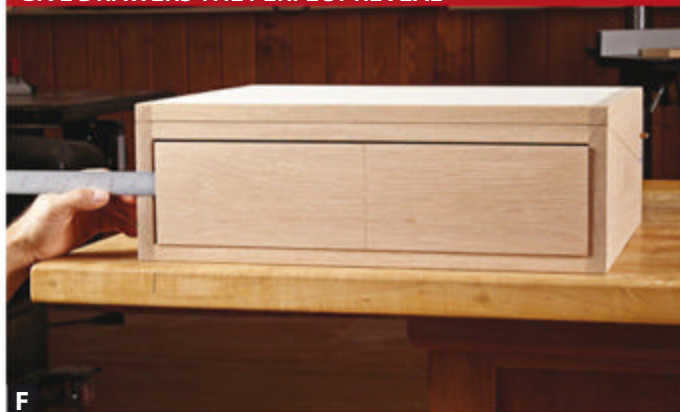
F Place the false fronts (L) inside the case, snug to one side. Measure the gaps between the false fronts and the case ( above ). Divide the vertical gap by three
