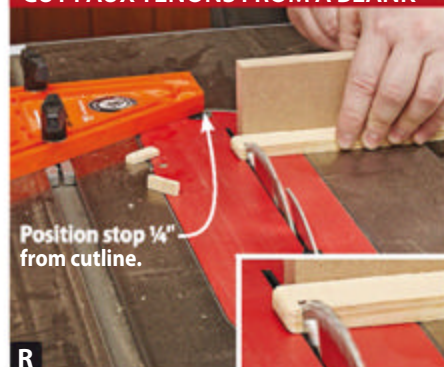
R Position a stop to leave a \frac{1}{4} " gap between the stop and the blade. Round over each end of the blank, cut off a faux tenon from each end, and repeat.
