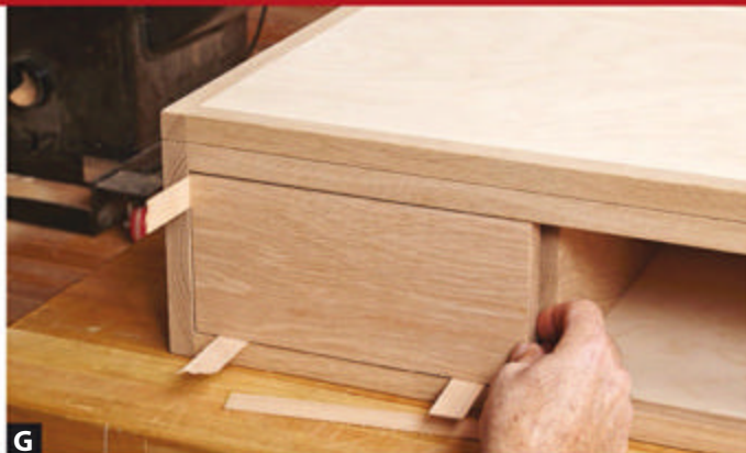
G to determine the thickness of the shims needed for an even reveal side-to-side, and divide the top gap by two for the top/bottom reveal ( above ).
