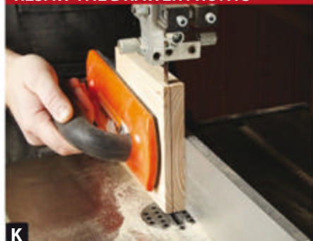
K Mount a sharp, wide blade in your bandsaw and cut slowly to achieve the smoothest surface. Even with saw marks, the pieces will mate up again perfectly.
