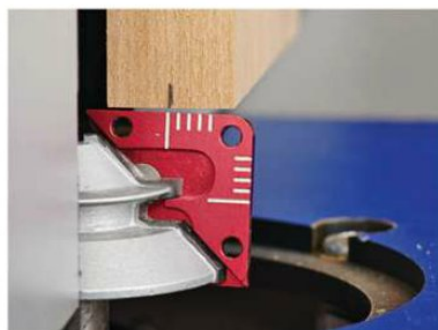
Jig must touch the bit below this cutter.
