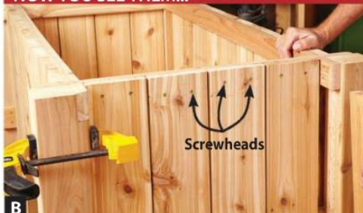
B Screws securing the slats on this planter disappear behind glued-on moldings that create the appearance of a frame.
