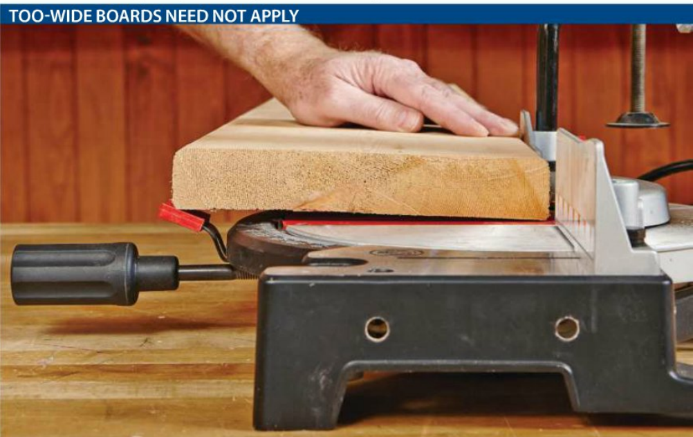
The miter-detent lever release on the Chicago Electric and Craftsman saws protrudes above table height, impeding wide workpieces, such as this 2×10 (which you'd have to cut, flip, and cut on this size saw anyway).
