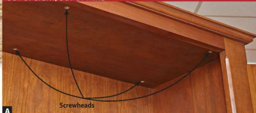
A The top of this 40"-tall bookcase sits below eye level of most viewers, so only the nosiest inspector will see the screws securing the top to the carcass.
