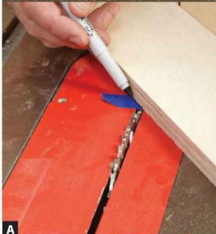
A Slide the plywood fence forward until it just touches the nearest tooth tip. Mark a line along the fence edge onto the painter's tape.
