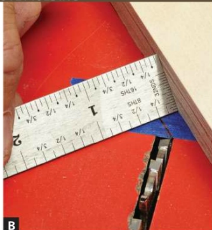
B Holding a steel rule perpendicular to the fence edge, slide the fence \frac{1}{4} " away from the blade and then mark another line on the tape.
