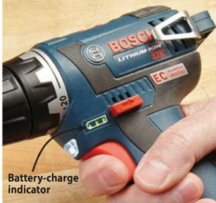
Battery-charge indicator LEDs, shown on the Bosch PS32-02, show more lights lit when the pack has a full charge.
