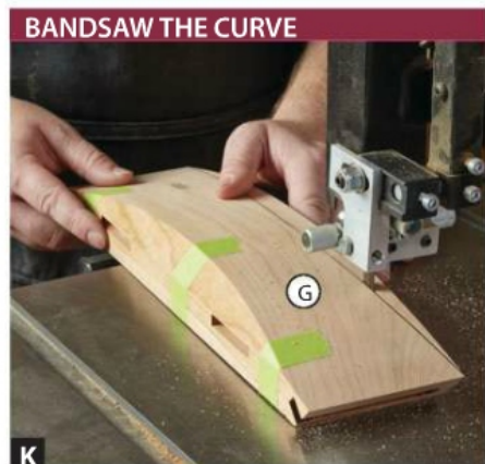
K To allow the back rail (G) to sit flat on the bandsaw's table during the cut, tape the bandsawn cutoff back in place.
