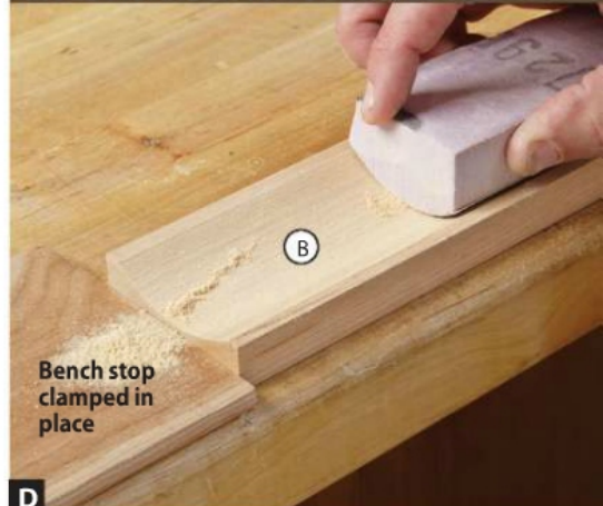
D Start sanding with 80-grit sandpaper to remove the saw-blade marks. Then follow up with 120, 150, 180, and 220 grit for a smooth, scratch-free cove.
