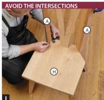
I When shaping the seat (H), leave flat the areas where the seat meets the back legs (A) to ensure the seat fits tight after shaping.
