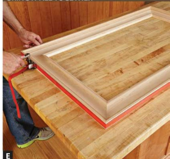
E Assemble the frame on a flat surface to ensure it remains flat. A band clamp applies even pressure to all four corners at the same time.
