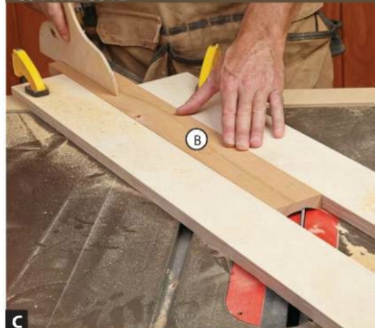
C Hold the big-cove blank (B) down to the tablesaw top while using a pushstick to move the blank forward. Feed slowly and take shallow cuts.
