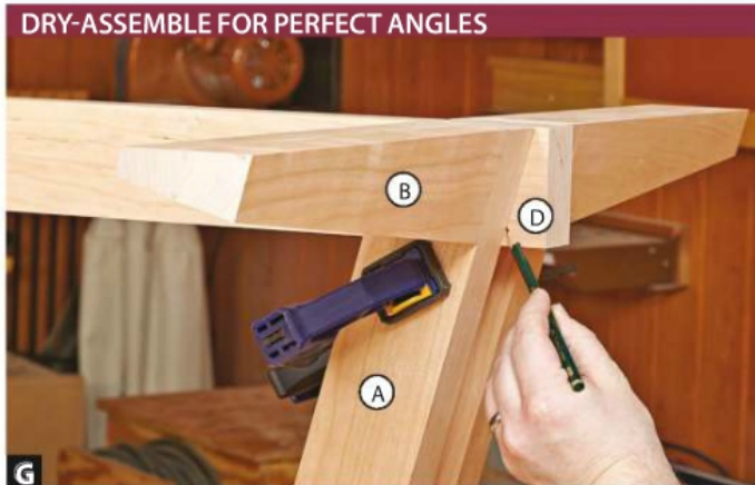
G By dry-assembling the base, you can scribe the stretchers (D, E) along the legs (A) to perfectly match the angle.
