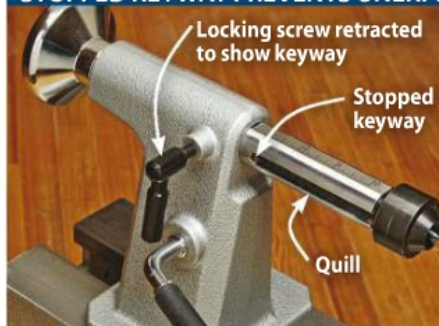
A quill with a stopped keyway, shown on the Delta.
