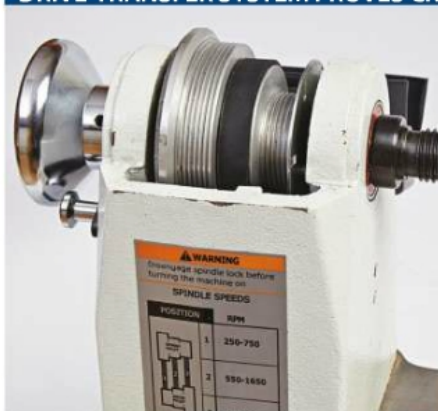
Rikon's 1/2"-wide rubber belt and three-step pulleys help generate superior spindle torque.
