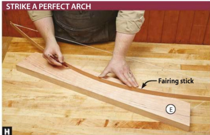
H With only a piece of a string and a long, thin cutoff, you can make a fairing stick like the one shown to make perfect, repeatable arches [More Resources].
