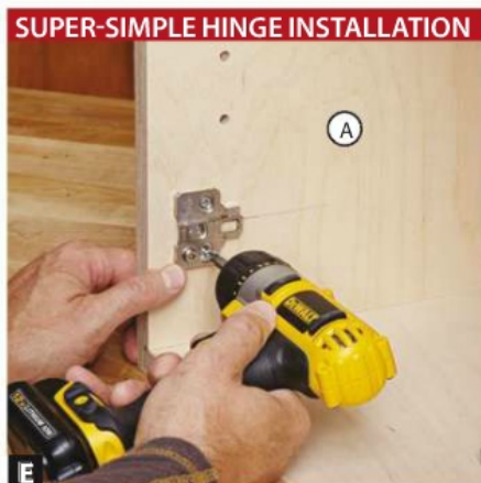
E Align the hinge plates along the centerlines on the sides (A) and drive the screws provided with the hinges into the holes drilled earlier.
