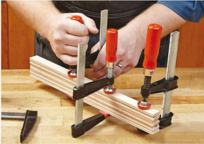
F The oversize stock used for the edge (C, D) strips and score strip (E) leaves spare material to square the edges if the laminations weren't perfect.
