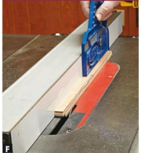
F The oversize stock used for the edge (C, D) strips and score strip (E) leaves spare material to square the edges if the laminations weren't perfect.
