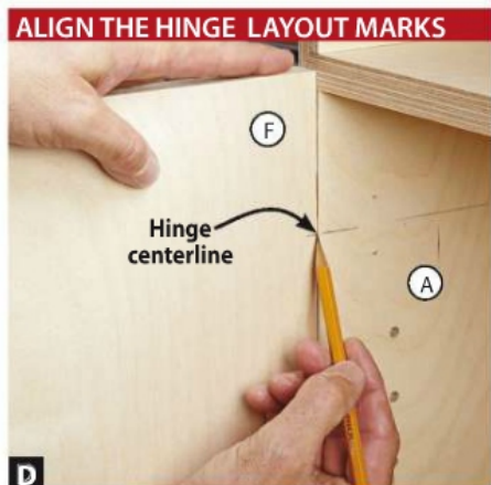
D Transferring the hinge-plate centerlines from the side (A) to each door (F) simplifies locating the holes for the hinge cups.
