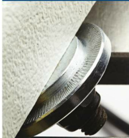
The stepped washer on Rikon's banjo has serrations that add grip when cinched tightly against the bed ways.
