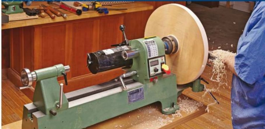
The General International headstock rotates 180° so you can turn 19"-diameter blanks, but the lack of torque becomes more apparent with larger workpieces.
