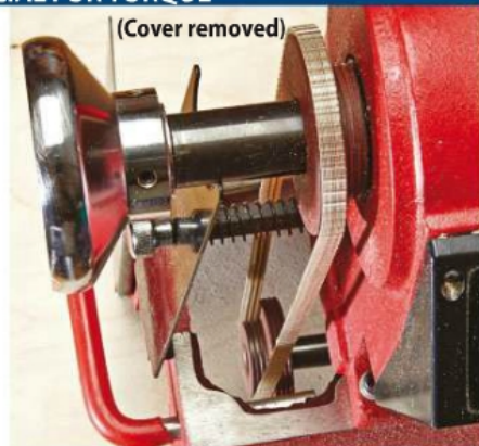
Penn State's narrower poly belt slipped regularly on the two-step pulleys during high-demand turning.
