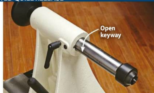
A quill with an open-end keyway, shown on the Jet.
