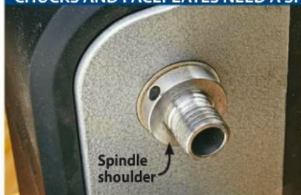
A broad spindle shoulder provides lots of bearing surface to better support faceplates and chucks.
