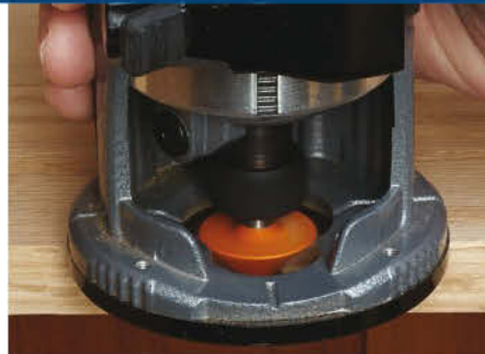
A metal base that wraps halfway around the base and the lack of an LED light make the MLCS Rocky 30 more difficult to use when you need to see the bit.
