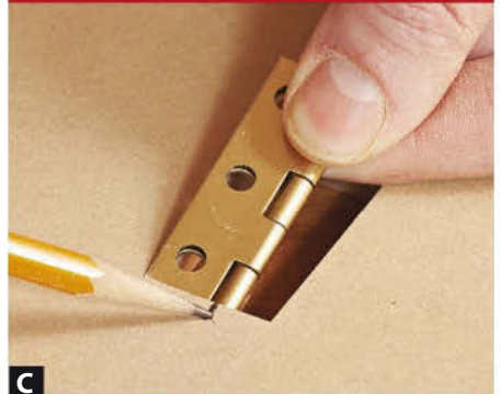
C Hold the closed hinge inside the bit opening, leaf-side tight to an edge. Mark the jig at the center of the hinge barrel—the location of the support arm.
