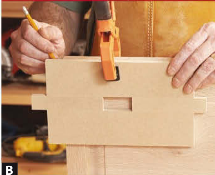
B Line up the bit opening with the hinge location on the edge of the door. Mark the jig along the door's end. Repeat for the other end of the door and jig.
