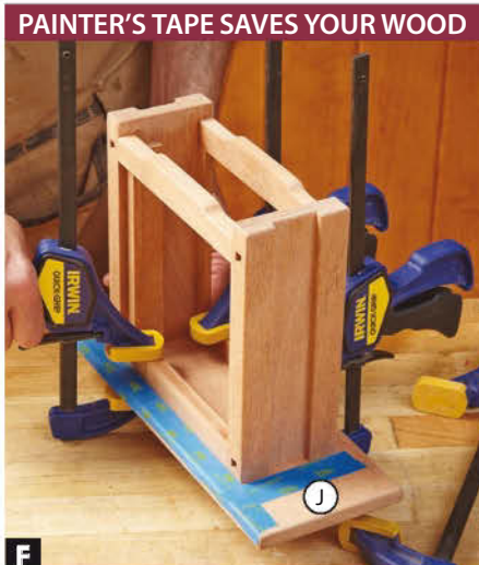
F Capture glue squeeze-out for easy cleanup by outlining the location of the clock's case assembly (A–F) with painter's tape.
