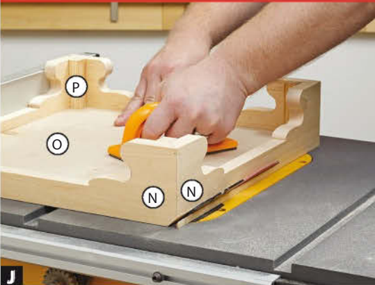
J When bevel-ripping the assembled base (N–P) at the tablesaw, push on the plywood panel rather than the aprons.
