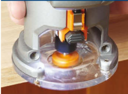
The combination of an LED light and a clear plastic subbase enhanced the Ridgid's bit visibility, even with larger-diameter bits.
