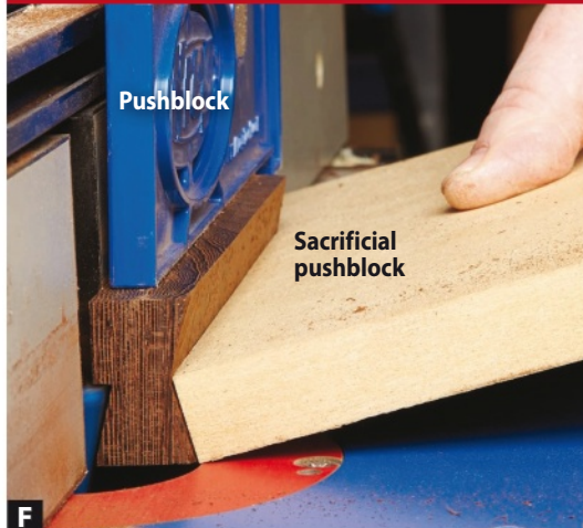
F Use a pair of pushblocks to keep the bowtie key stock tight to the fence. Sneak up on the final width of the key by making additional passes as necessary.
