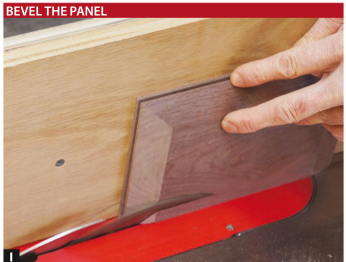
I Tilt your tablesaw's blade to 15° to cut bevels in the panel. By cutting the end grain first, the long-grain cuts will remove any tear-out.
