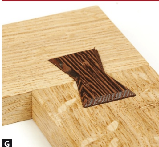
G On raised bowtie keys (and splines) carefully add a bevel to the proud edges using a sharp chisel after the frame has been assembled.
