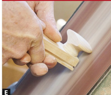
E When sanding a small part, such as this drawer pull, secure it to a piece of scrap with a screw or double-faced tape to keep your fingertips safe.
