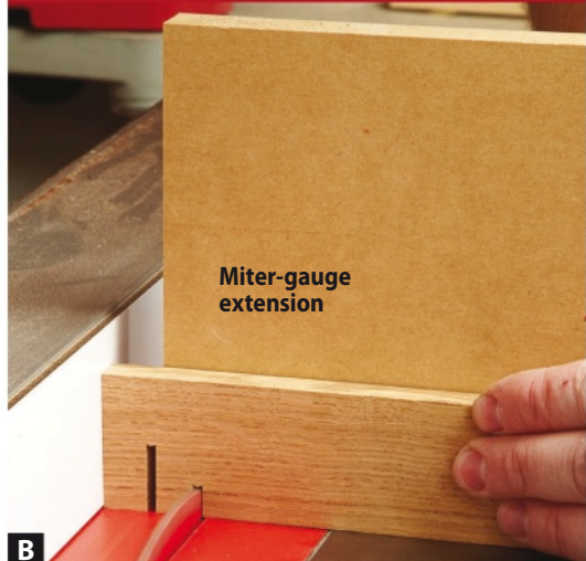
B Without moving the tablesaw's fence, hold the adjoining piece to the miter-gauge extension. Make the matching cuts.
