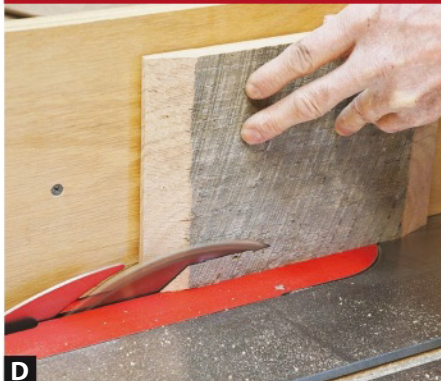
D Tilt the tablesaw's blade to 17°, attach a tall auxiliary fence to support the box top during the cut, and set the fence \frac{3}{16} " from the blade.
