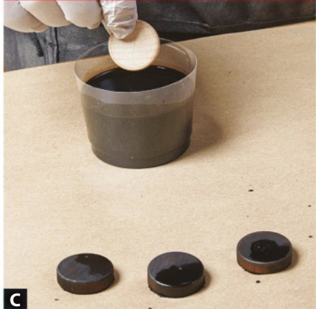
In a wide-mouthed container, mix up a water-based dye in your desired color. Wipe excess liquid from each game piece before laying it down to dry.
