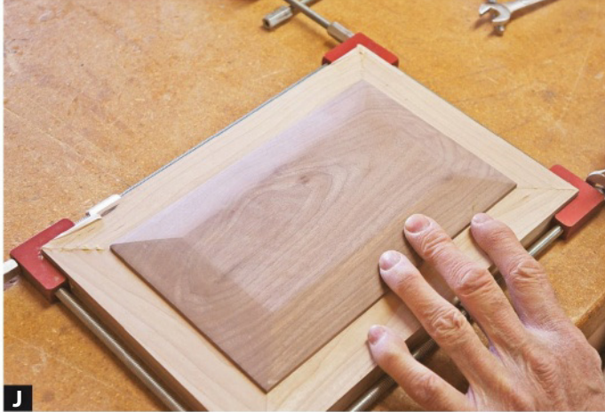
J Apply a small amount of glue to the grooves in the frame and to the frame's miters. Use corner or framing clamps to keep the assembly tight as it dries.
