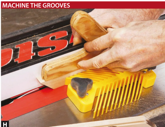
H Use a pushstick and featherboards when cutting grooves in the frame pieces to keep hands safe. Apply even pressure throughout the cut.
