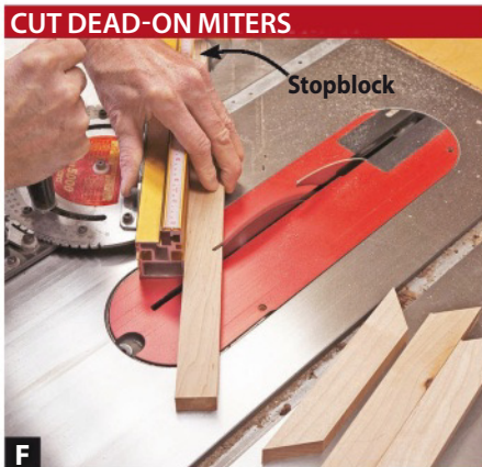
F For tight joints, set your miter gauge to exactly 45° and clamp on a stopblock to make certain opposing sides come out the same length.
