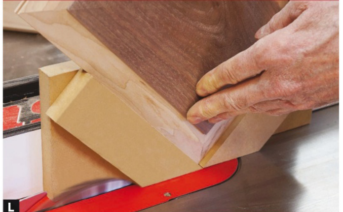
L A simple splining jig made of scrap sheet goods will help you cut kerfs for holding accent splines. Those splines also strengthen the top's miter joints.
