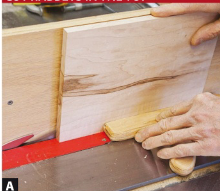
A A tall auxiliary fence on your tablesaw supports the top during machining and prevents any damage to the fence when running the blade flush against it.
