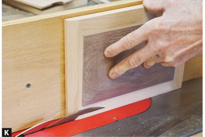
K After adjusting your tablesaw's blade to 17°, use a tall auxiliary fence to support the top as you cut bevels in the frame's top face.
