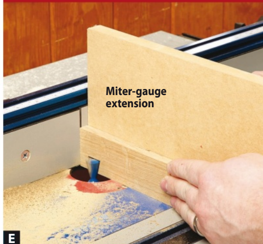
E Without moving the router table's fence, clamp or hold the second piece to the miter-gauge extension and against the fence. Make the matching cut.
