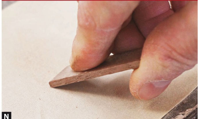
N Round over the ends of the lift tabs to fit the rounded slots. Use a piece of 100-grit, self-adhesive sandpaper on a flat surface.
