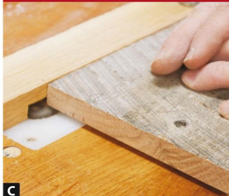
C Rabbet the ends of the lid first so the subsequent cut along the sides, such as the one shown, will remove any end-grain tear-out that may occur.
