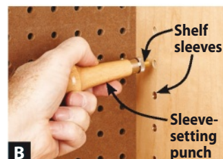
B A sleeve-setting punch ($16) helps you install the brass shelf-pin sleeves after redrilling the holes. This model has five tips for different-size sleeves.
