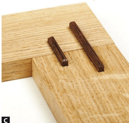
C Match the spline stock width to the thickness of the frame for a flush fit, or \frac{1}{8} " wider so they stand proud.
