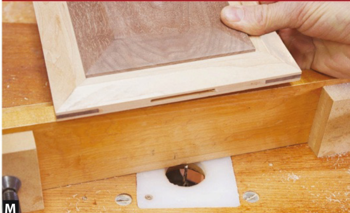
M Adjust the router-table fence so the slot aligns with the top's splines. Set the bit \frac{3}{16} " high and use stopblocks to center the cut.
