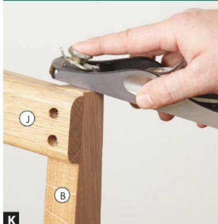
K Use a low-angle block plane to shave the tops of the back legs (B) until they are flush with the curve of the top back rail (J).
