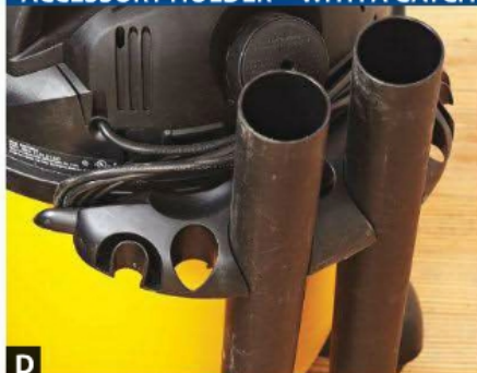
D Six Shop-Vac models have friction-fit accessory hangers that interfere with the cord wrap and allow extensions to slip to the floor.
