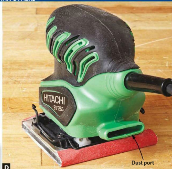
D The square or rectangular ports on most orbital sanders fit their provided collection bags or canisters, but are tricky to adapt to shop vacuums.
