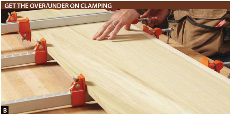
B By alternating clamps above and below the glue-up, Kevin and John ensure that any cupping is neutralized by the opposing clamping pressure.
