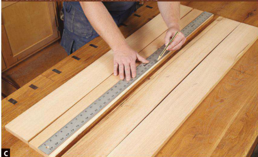
C John marks lines on the board faces parallel to the edge to remove sapwood and other imperfections.
