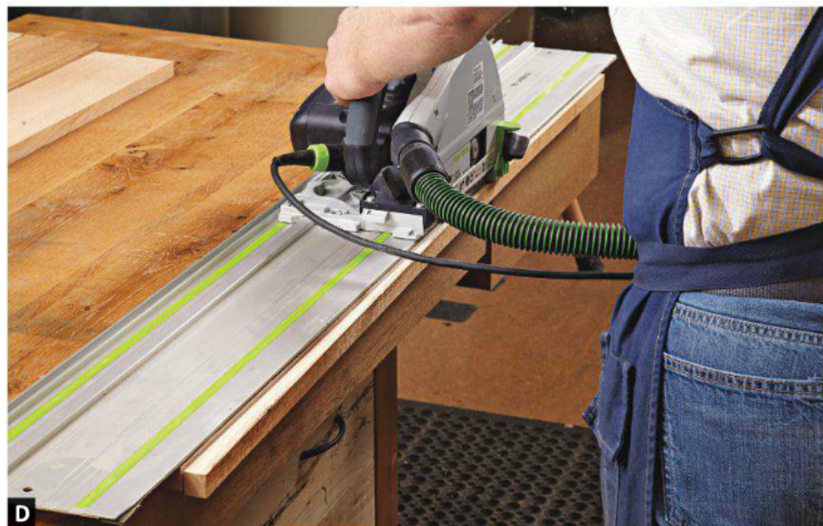
D Then, using a circular saw and guide, track saw, or bandsaw, he cuts along the marked line.
