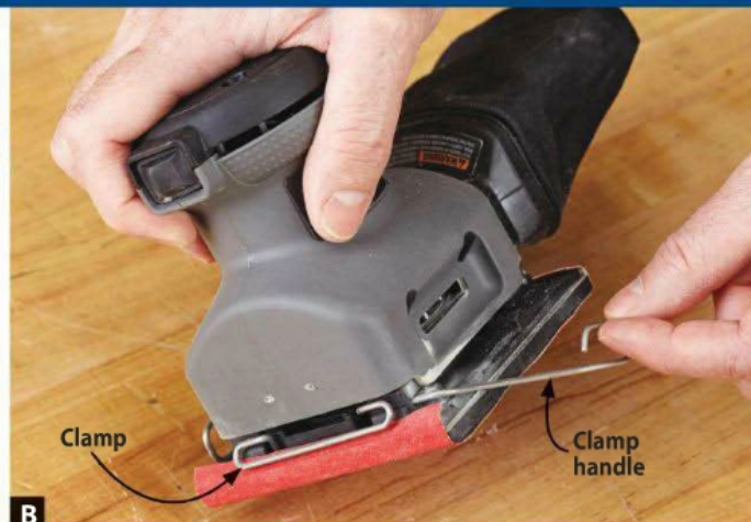
B Orbital finishing sanders use cam-action clamps to hold sanding sheets in place, but the sheets can be awkward to install.
