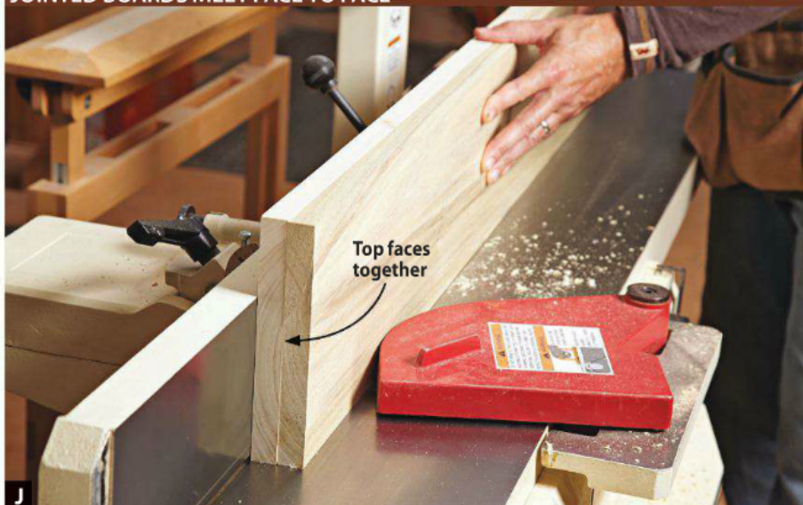
Placing adjoining boards face-to-face ensures complementary angles even if the jointer fence isn't perfectly square to the tables.
