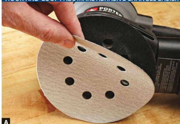
A With random-orbit sanders, you quickly and easily apply hook-and-loop discs to the pad. This makes sequential-grit sanding a breeze.
