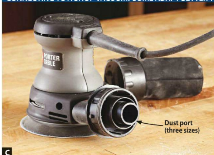
C Although sized differently from brand to brand, round dust ports on most random-orbit sanders adapt relatively easily to a shop-vacuum hose.
