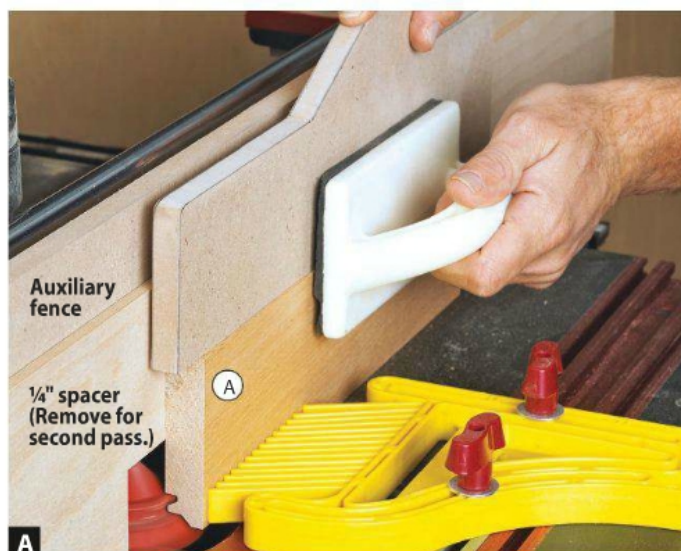
A spacer makes the first cut shallow; remove it for the second pass. Use a featherboard and pushblocks for safe, accurate routing.
