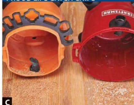
C Lipped tub rims that flare inward (Ridgid WD1680, left) catch debris when dumping. Smooth-rimmed vacs (Craftsman XSP 12007) dump cleanly.
