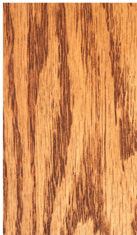
Sanded to 220 grit: No visible scratches visible after staining.
