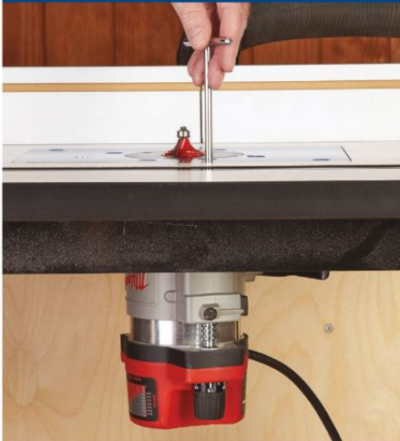
You adjust bit height with the Milwaukee 5625-20 fixed-base router by using the included T-wrench to reach through a hole in the insert plate.
