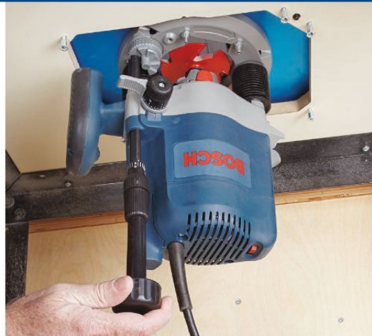
Although you still have to reach below the table, Bosch's extension handle makes it easy to raise and lower the router as you eyeball the bit.
