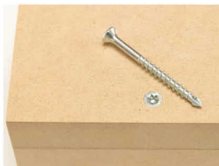
Self-drilling, multi-material screws, such as these from Spax, prevent splitting while eliminating the time-consuming job of drilling pilot holes.
