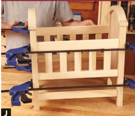
J Use bar clamps to draw the bed components together, checking for square as you tighten; then, allow the glue to dry before final sanding.
