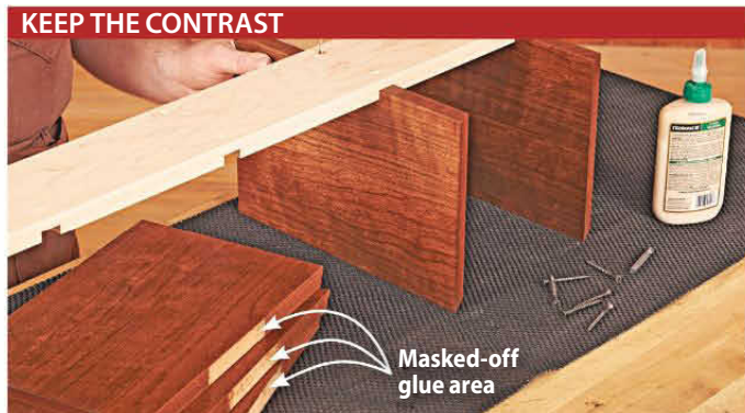
Staining these shelves before screwing them in place gives easy access to all sides of them and eliminates stain creeping onto unstained parts.
