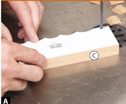
A We used a bandsaw equipped with a ¼" blade to shape the subtop (B) and subbase (C), but a #7 blade in a scrollsaw works well, too.
