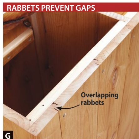
G As each slat expands or contracts, the rabbets slide over each other, preventing see-through gaps from opening up between slats.
