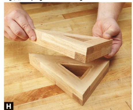
H Glue and clamp the subassemblies together to create the stand. For the tablet-stand version, position the subassemblies with extended bases as shown on the previous page.
