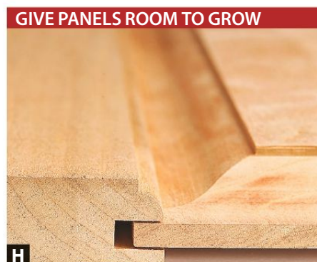
H When sizing a solid-wood panel to fit within a frame, allow about ⅛" between the edge of the panel and the groove bottom.
