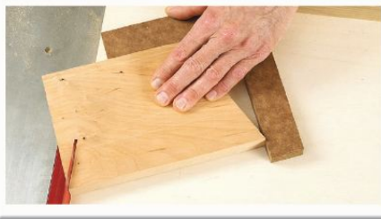
G Glue and clamp a second base piece (C) on top of the first base piece to complete a subassembly.
