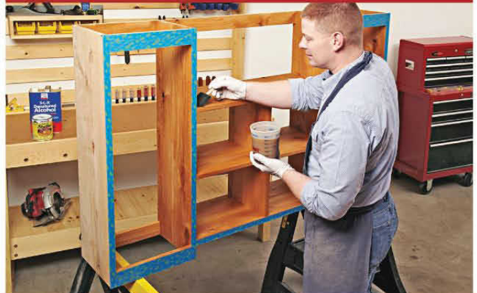
Staining a partial assembly provides better access to its interior. Painter's tape masks glue surfaces for the face frame added later.
