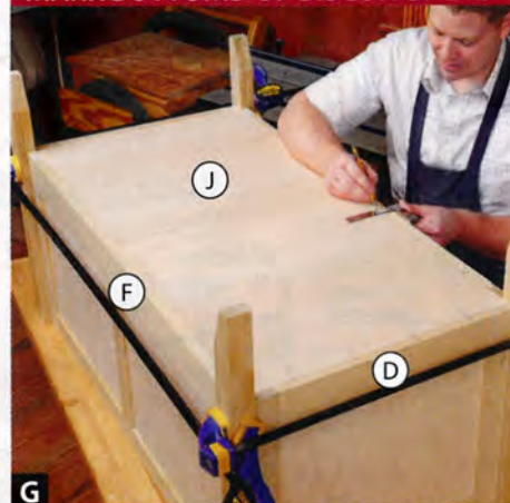
G With a square and pencil, mark across the bottom (J) and adjoining rails about every 6" to locate biscuit cuts.
