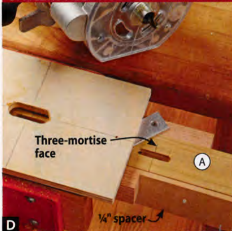
D To offset from center the mortises on the three-mortise face of each leg, position a \frac{1}{4} " spacer against the tapered face of the leg.
