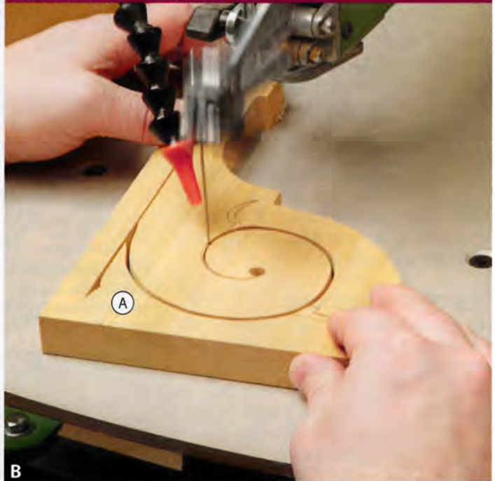
B Keep steady, moderate pressure on the workpiece to prevent burning. Forcing the work flexes the blade, causing a less-than-square cut.
