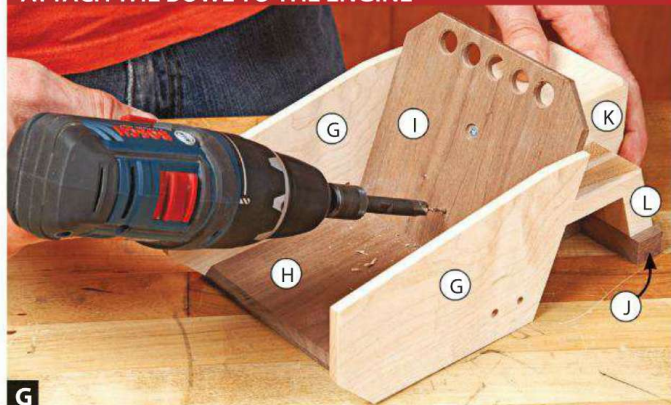
G Rest the bowl assembly (G/H/I) and the rear assembly (J/K/L) on your bench, drill countersunk pilot holes, and glue and screw the assemblies together.
