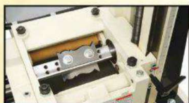
Easy Access Cutterhead for Trouble-Free Blade Changing
