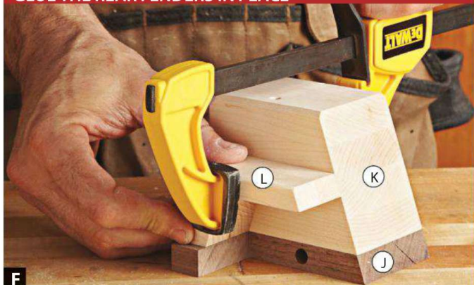
F Align the rear fenders (L) with the rear chassis (J) and rear engine (K) as shown. Clamp lightly, check the fender positioning, then tighten the clamp.
