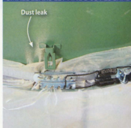
Band clamps don't always form a tight seal when securing a bag, which is usually oversize, to the machine's rim, creating a dust leak under pressure.
