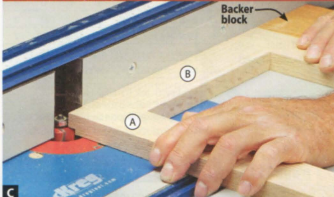
C Employ the same tenon-cutting technique used on the ends of the support rails (B) to form a tongue along one short edge of both support frames (A/B).
