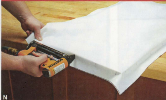
N Staple along one long edge of the filter frame (BB/CC) first. Then, pull the filter fabric taut as you staple along the remaining edges. Trim off the extra material along all edges before gathering the corners and trimming those, too.
