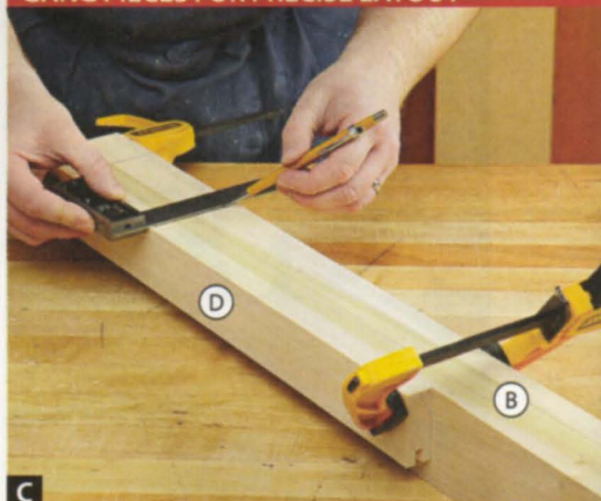
C To match the locations of mortises on mating workpieces, clamp them together and mark the locations using a square and sharp pencil.
