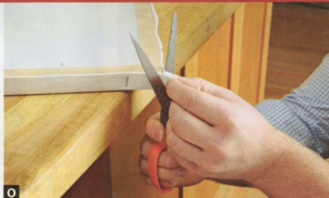
N Staple along one long edge of the filter frame (BB/CC) first. Then, pull the filter fabric taut as you staple along the remaining edges. Trim off the extra material along all edges before gathering the corners and trimming those, too.
