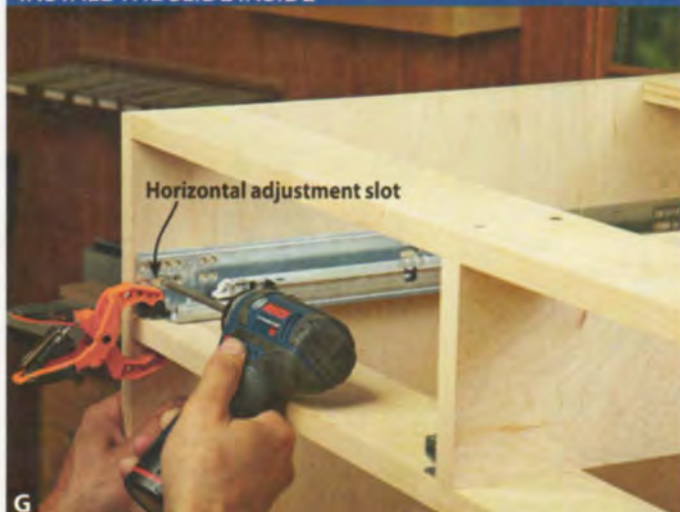
G Clamp the slide flat against the stretcher and \frac{1}{16} " back from the cabinet edge. Screw through the horizontal slot to allow for later adjustments.
