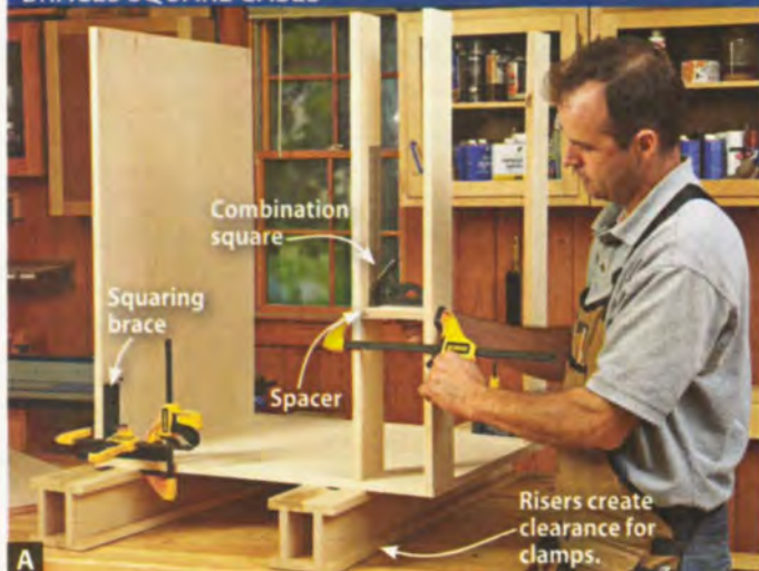
A Squared up and clamped in place, the spacer maintains the correct stretcher position. Squaring braces align the top rear stretcher and bottom.
