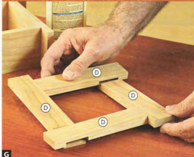
G First, tip the outside edge of each rail pair up. Then, slide the rabbets into the mating dados. Finally, tip the pairs down, flattening the frame.
