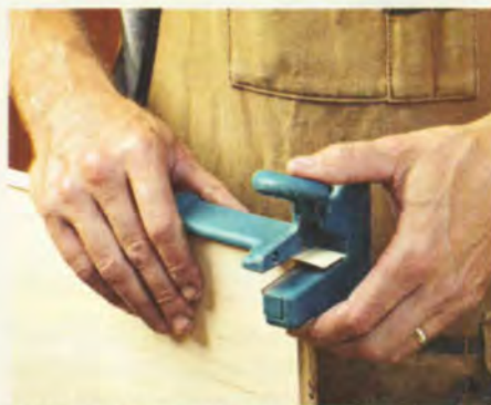
As the glue cools, seal the banding tight by burnishing it with the shaft of a screwdriver. Then use a veneer guillotine (above) to create a flush, square cut at the ends of the panels.
