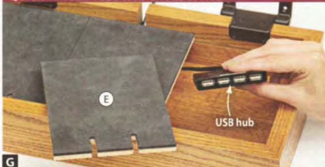
G Rather than cram a power strip and chargers under the trays (E), drop in an AC-powered USB hub to charge your devices instead.
