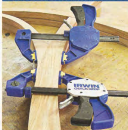
The jaws of the Quick-Grip XP600 can pivot, allowing them to conform to curved and angular shapes, an otherwise difficult clamp-up.
