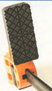
The wafflelike pattern on the Jorgensen clamp pads left indentations (revealed here by pencil rubbings) on softer woods when clamped tightly.
