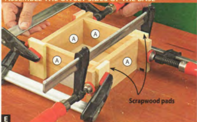
E Apply glue sparingly to the side (A), dados, and grooves, and glue and clamp the sides, capturing the bottom (C) within the grooves.
