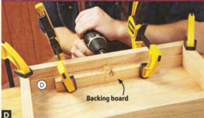
D Before drilling the bottom of the power-cord slot, clamp a backing board to the tray support (D).
