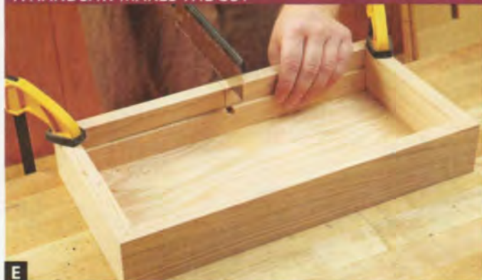
E For optimal results, use a short backsaw (a handsaw with a stiff rib on its back) with 14–22 teeth per inch when cutting the slot.
