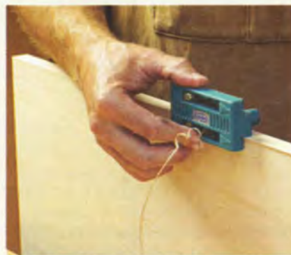
Last, use a veneer edge trimmer to pare away the excess along the faces. A smooth cut requires only light pressure. Clean up all the cuts with a light sanding pass using 220-grit sandpaper.
