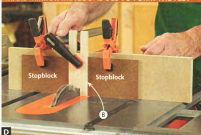
D Center the foot (B) blank on the dado blade, and flank it with stopblocks. Cut one notch, flip the blank, and cut a second notch.
