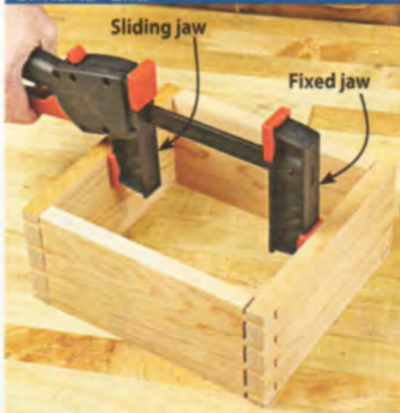
Bessey's DuoKlump proved easiest to convert to a spreader: Swap the pads to the opposite jaw sides and rotate a dial on the sliding jaw.
