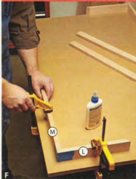
F Tape the base sides (M) and ends (L) together in pairs. Add glue to the miter, fold, wipe away excess glue, and clamp the assembly to your worksurface.
