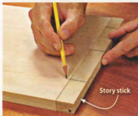
A story stick ensures marking accuracy, especially when laying out multiple parts or transferring measurements among workpieces.
