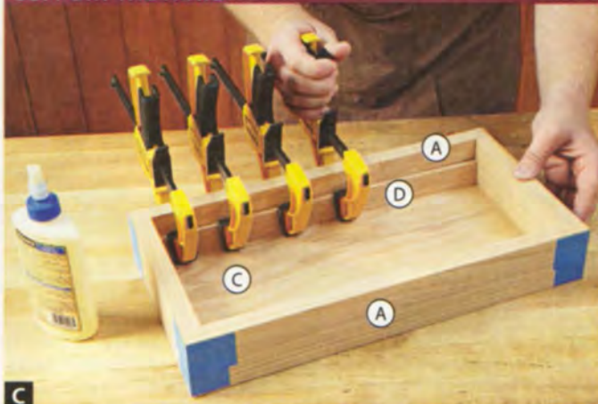
C With two tray supports (D) cut to length, glue and clamp them to the inside faces of the valet's front and back (A), tight against the bottom (C).
