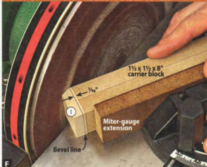
F Fasten the top face of the handle (I) to the end of a 1½×1½×8" carrier block, and disc-sand the bevels to the marked lines.
