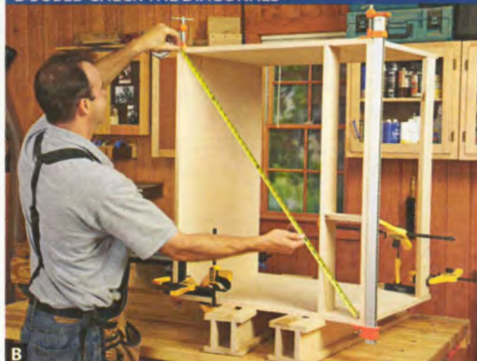
B When the diagonal measurements in both directions are equal, the case is square. Otherwise, loosen the clamps, adjust the case and retighten.
