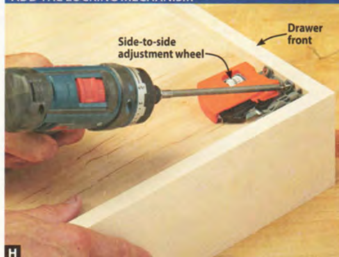
H The locking mechanism captures the front of the slide and features a side-to-side adjustment wheel that allows for fine-tuning.
