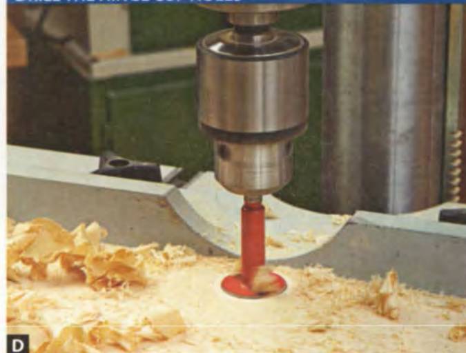
D Although the hinge instructions call for 35mm holes to fit the hinge cups, a 1 3/8" Forstner bit matches close enough to save buying a bit.
