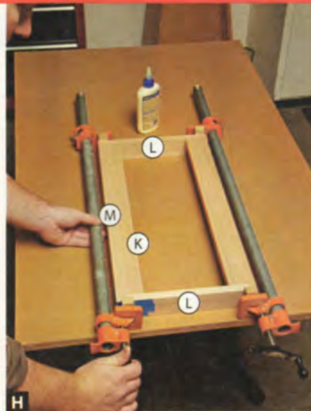
H Glue and clamp two half-bases (K/L/M) together using clamping blocks. The cleats (K) register against the ends (L) to square the assembly.
