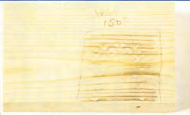
The wafflelike pattern on the Jorgensen clamp pads left indentations (revealed here by pencil rubbings) on softer woods when clamped tightly.
