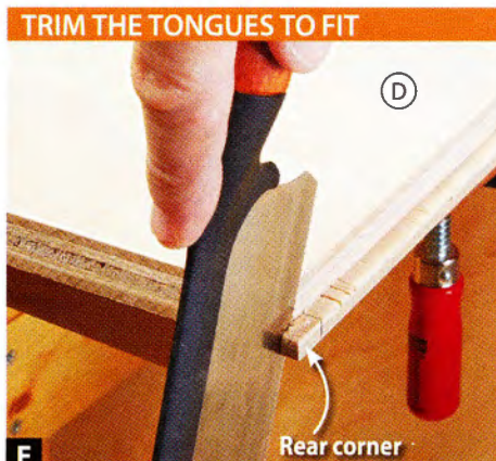
E To allow the shelves (D) to extend past the sides (B) at the rear of the table, use a handsaw to cut \frac{1}{2} " from the rear of each tongue.
