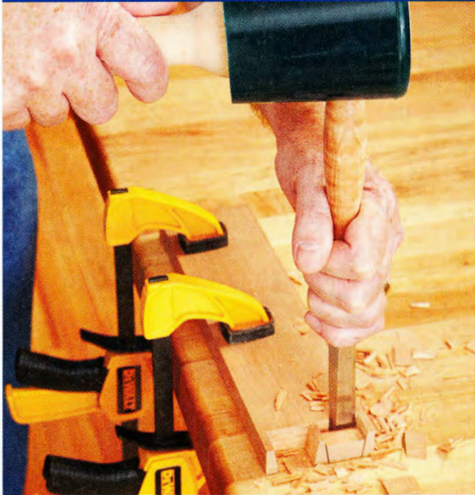
When chopping dovetails or mortises, we grab a fistful of handle to maintain the best control. Try the tool first by holding it in this manner.
