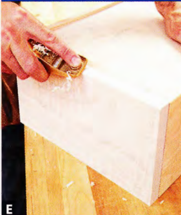
E Plane a small chamfer along the bottom edge of the false front, test fitting the drawer frequently to ensure an even reveal.
