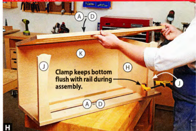
H Glue the remaining edges of the back/bottom (H-K), rails (J) and biscuit slots. Carefully position the leg assembly (A-D) and clamp the case.
