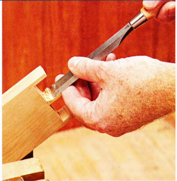
And for light-duty paring, such as trimming dovetail pins, we like to use one hand to guide the blade and the other to push. Test the feel this way, too.
