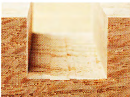
The stacked dado set that cut this channel left ridges in the bottom caused by slight height variances between chippers and blades.
