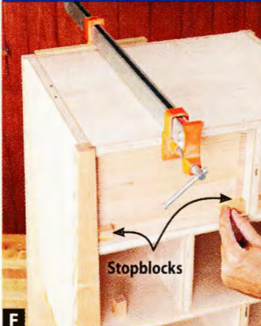
F Clamp a scrap on the case front and press the drawer against it. Glue in stopblocks; avoid gluing the drawer to the case.
