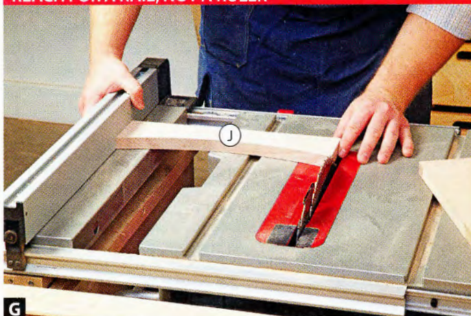
G To ensure a square case, use the length of the top rail (J) to position the fence before cutting the back (K) and bottom (H/I) to final width (about 13 3/4 inches).
