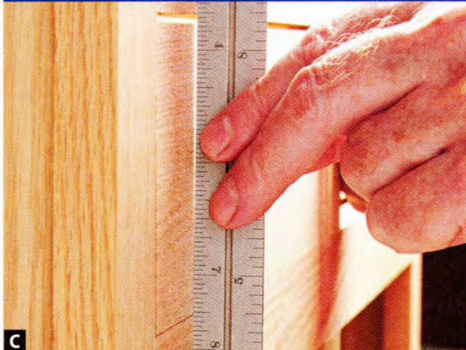
C A steel rule and back light help you quickly check the alignment of the drawer front. Unequal gaps or protrusions require slide adjustments.
