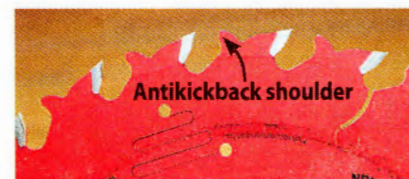
The shoulder behind each tooth on this 24-tooth rip blade limits how deeply the next tooth will cut.
