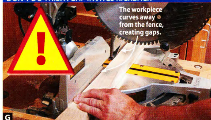
G With gaps behind the cutline, the rotation of the blade can shift the workpiece backward, pinching the blade.
