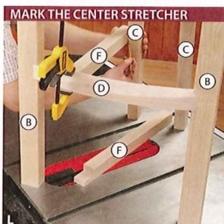
L Align the center stretcher (F) with the edge of the back leg (C), and clamp it to the front stretcher (D). Mark the center stretcher's length.
