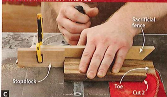
C Tilt the blade to 45° and move your miter gauge to the other slot. Position the wedge assembly (A/B) so the second cut hits a blade's thickness from the cut end of the extension. Cut the toe and set it aside.
