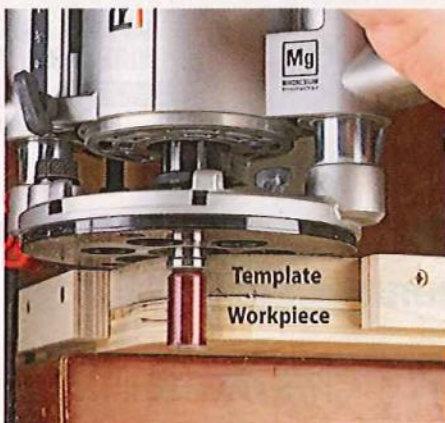
Handheld routing with a pattern bit keeps the template on top, improving visibility and avoiding potential marring from the router's subbase.
