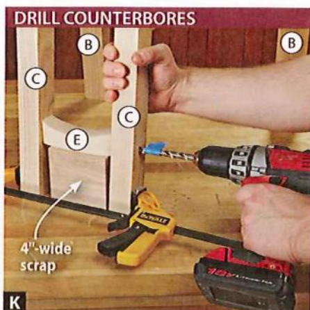
K Support the lower back stretcher (E) with a scrap block while drilling the counterbores and shank holes through the back legs (C).
