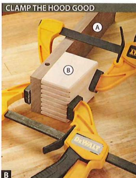
B Glue the hood (B) above the front axle holes, aligning the front and edges of the hood with the front and edges of the chassis (A).
