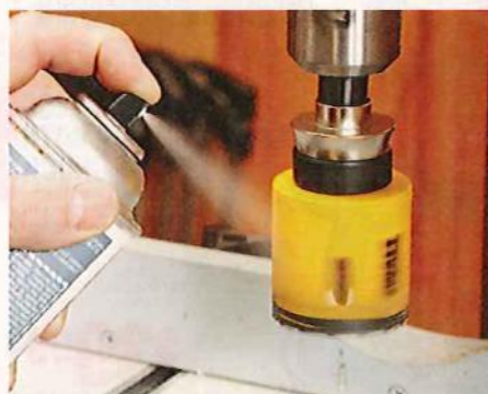
With the drill press running, spray the lubricant onto the holesaw's outer and inner walls and teeth. Leave it running until dry.
