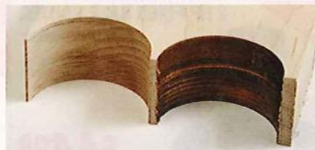
In maple, we made the hole on the right using a new holesaw. The unburned hole (left) was made using relief holes and dry lubricant.
