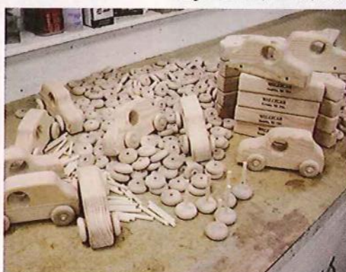
WallyCar parts—bodies bandsawn and branded by the couple and purchased wheels and axles—await assembly.
