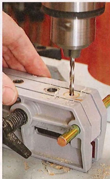
With your drill-press table squared to the bit, use the jig to hold the dowel and bore a \frac{3}{16} " hole down its center.
