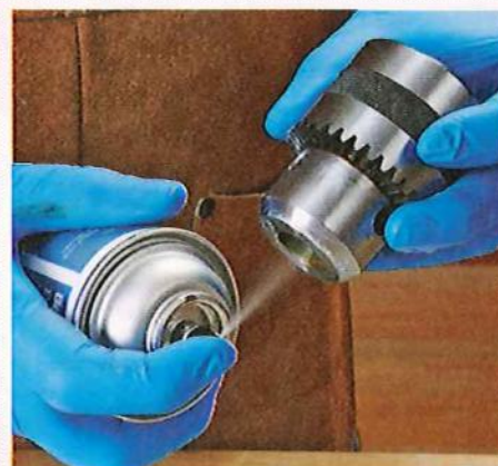
Spray on a couple of coats of a quick-drying lubricant, with jaws open and closed, before reinstalling your chuck onto the drill press.
