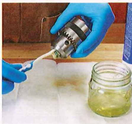
Hold the chuck jaws down to avoid getting solvent on the bearings; solvent could erode the bearing seals and lead to a bigger repair.
