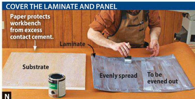
N When spreading cement on a wide area, work quickly and make sure to cover the entire surface. A roller speeds work on large surfaces.
