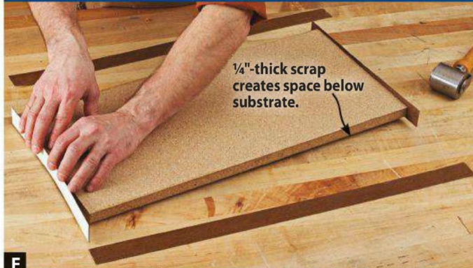
F A spacer below the substrate allows room for the over-width edging to extend past the bottom face. Roll the edging firmly after application.
