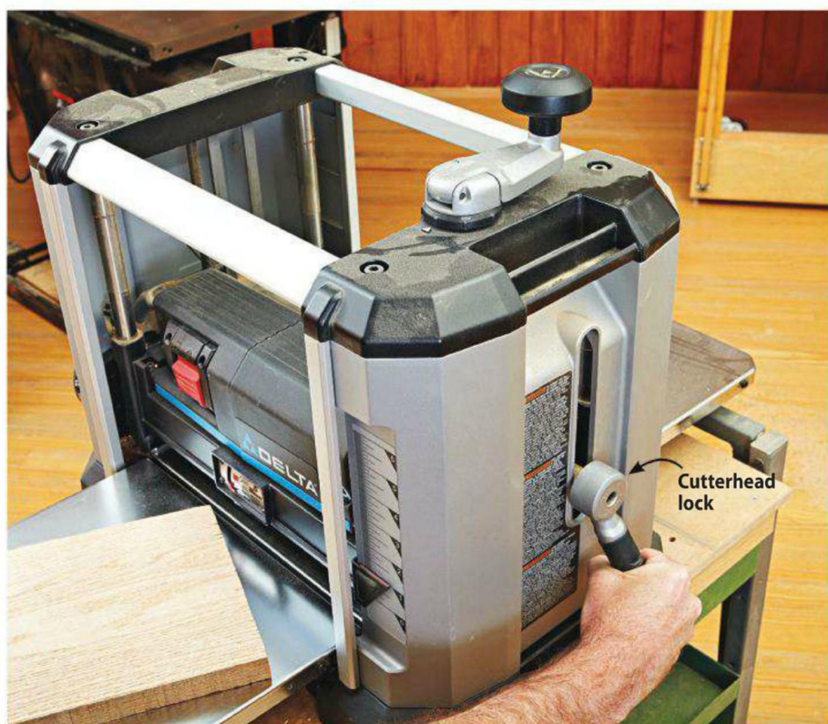
The cutterhead lock found on many benchtop planers helps to alleviate snipe on the ends of boards.
