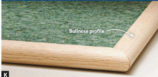
K Use biscuits (or rout grooves in the substrate and edging, and then use splines) to help align the edging and laminate flush.
