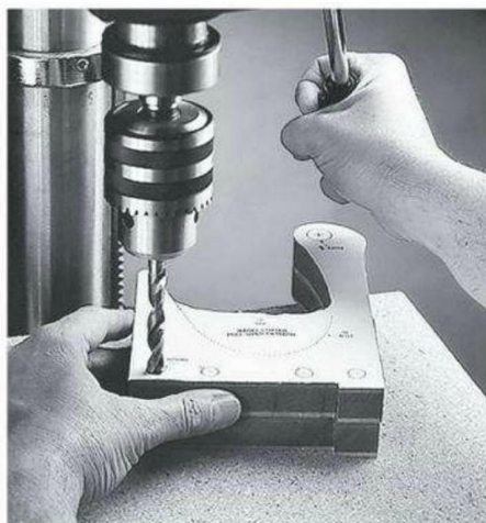
Drill through both body halves at once. This way, the sides will mate accurately.
