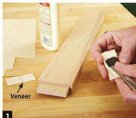
1 Use a craft knife and straightedge to trim veneer pieces slightly larger than the tenon cheeks, and glue them in place.
