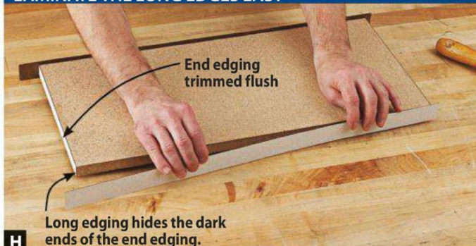
H Position the two remaining pieces so they extend past the end edging. Roll the edging firmly; then trim it flush.
