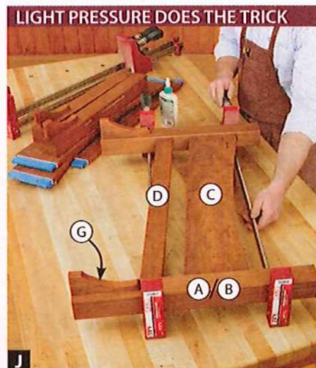
J The clamp heads don't align with both ends of the stretchers (C, D), so to avoid flexing the legs, apply only enough pressure to close the joints.
