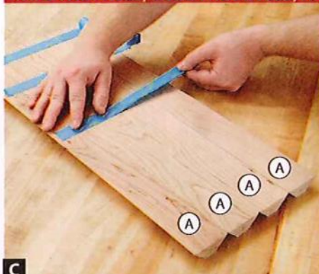
C Place the leg faces (A) edge to edge, outside-face up, with their ends flush, and apply several strips of painter's tape across all four faces.
