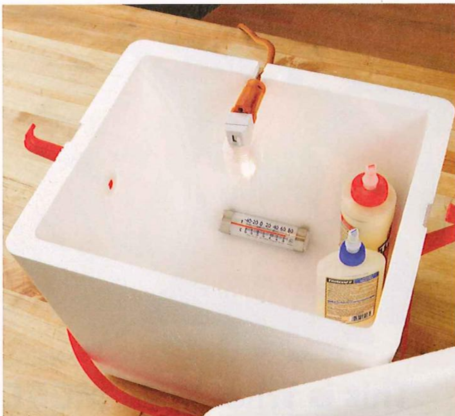
A 4-watt night light bulb supplies enough heat to maintain the temperature inside this styrofoam ice chest at about 70° F in 36° F weather. Upgrade to a 7-watt bulb if more heat is required.
