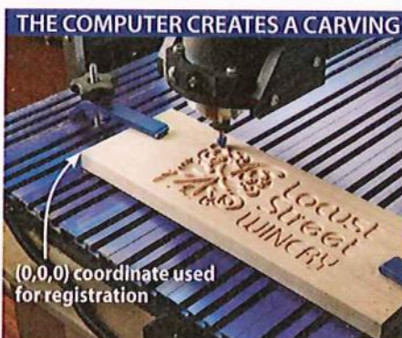
After registering the bit's point on the workpiece's corner to set the (0, 0, 0) point, start the carving, sit back, and watch.
