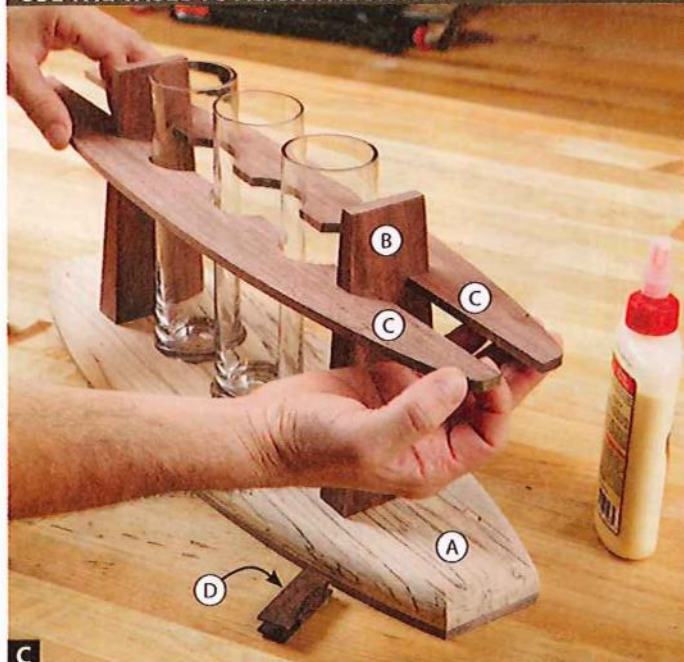
C Dry-fit the retainer strips (C) in the notches in the uprights (B). Position the strips to center the vases in the openings without the vases touching the strips.
