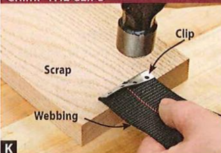
K Rest a clip on a scrap, place the webbing in the clip, and then hammer the clip closed. Teeth inside each clip bite into the webbing.
