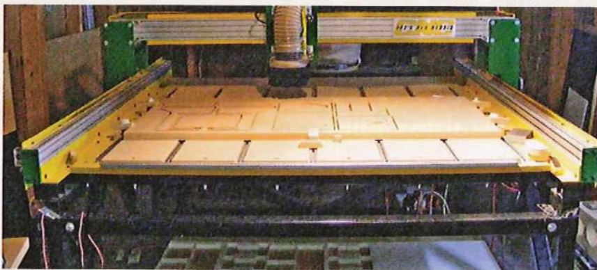
Joe's do-it-yourself CNC machine has a 48x48" envelope—nearly three times the area of the largest-capacity commercial benchtop machine—but costs less than half as much to build.
