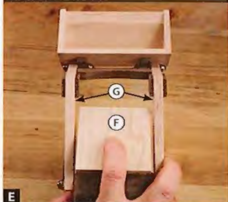
E After gluing the roof (F) in place, raise and lower the loader arms (G) to ensure they clear the sides of the roof.
