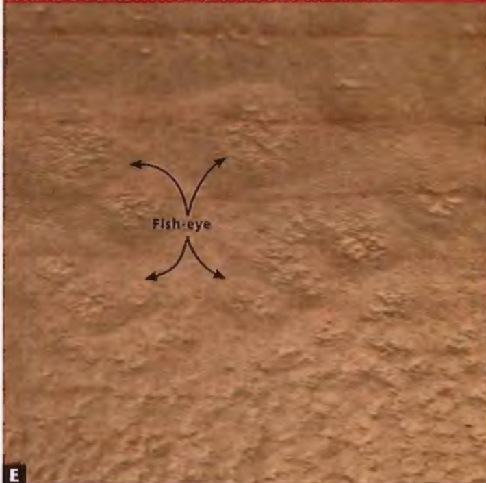
E Silicone from some furniture polishes causes additional coats of finish to bead up like water drops on a waxed car, an effect called fish-eye.
