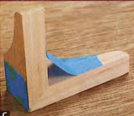
Gluing up the feet (H) requires force on both sides to hold the halves together—apply painter's tape along the inside and outside for a tight joint.
