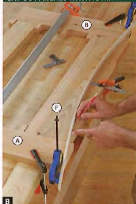
B Flex a \frac{1}{4} "-thick strip between two clamps. A metal rule or scrap clamped in place holds the strip 2" in at the centerpoint of the arch.
