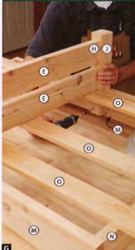
G Rest the center armrest assembly (E/H-K) on several inner seat slats (O), centered on the base (M/N) width, then screw the assembly in place.
