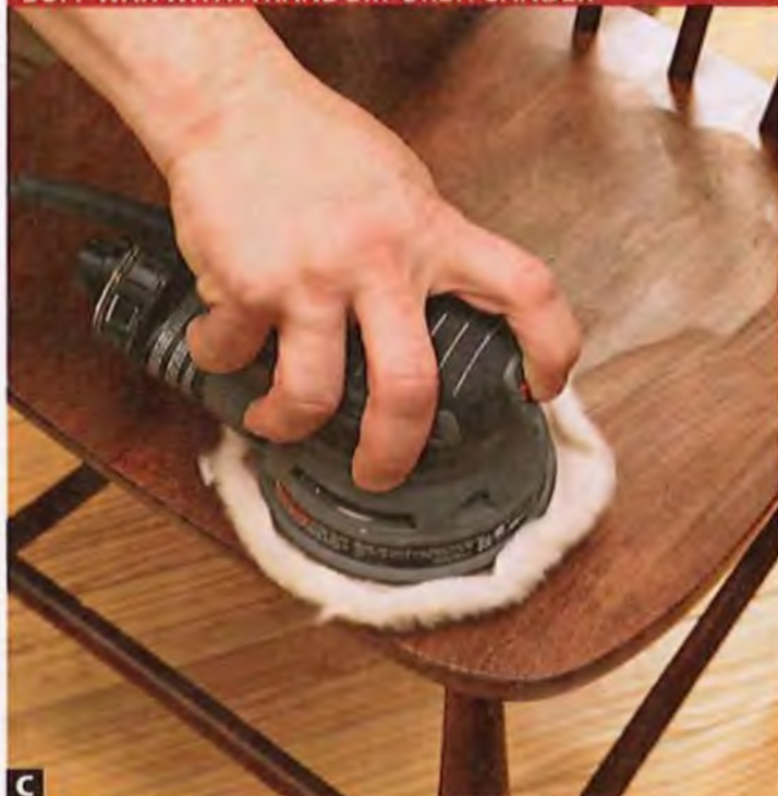
C To make a random orbit sander buffing pad, attach the pad to the grit side of a sanding disc using adhesive strips. (See Sources.)
