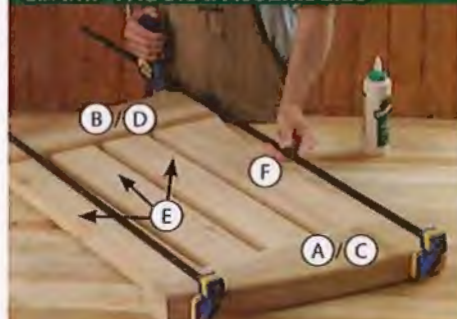
E Glue the side rails (E) and side bottom rail (F) into a front leg assembly (A/C), then clamp the back leg assembly (B/D) to the rails.
