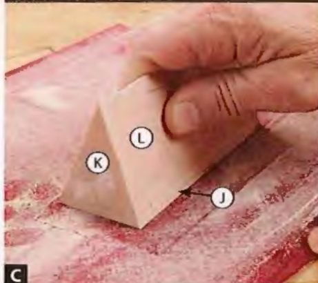
C Lay a piece of 220-grit sandpaper on your bench and sand the edges of the bucket sides (K) flush with the faces of the back (J) and bottom (L).
