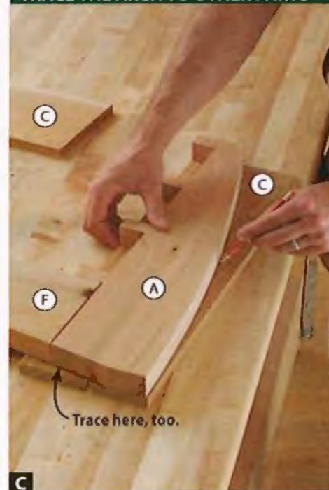
C Align the ends and notched edges of the leg cores (A, B) with the edge and ends of the leg skins (C, D), then trace the curves.
