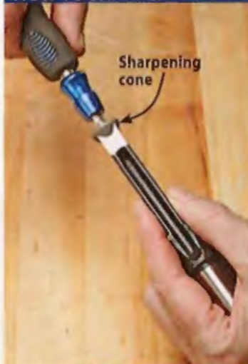
Step 1: Spin the diamond cone tool to hone the inside hollow point of the chisel. Follow up with a finer-grit cone for best results.
