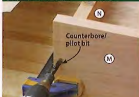
F A counterbore/pilot bit drills the pilot hole and countersink in one step. Clamp the mating pieces together so the holes align.
