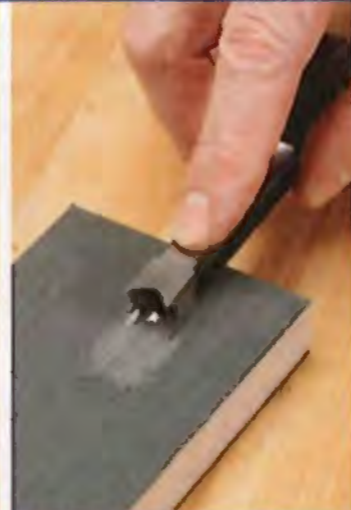
Step 2: After honing the inside, remove the burr on the outside of the chisel by rubbing it lightly a few strokes on 800-grit sandpaper.
