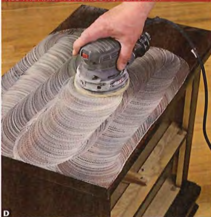
D Remove sanding scratches using Finesse-It II Machine Polish and a white, non-woven cleaning pad. Check the finish often as you work.
