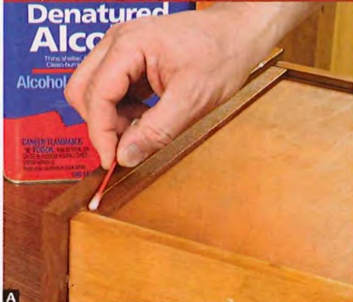
A The underside of a drawer provides an ideal place to test for the type of finish using alcohol first and then lacquer thinner.
