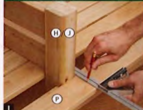
I Use a combination square to transfer the location of the post (H/J) to the outer slats (P). Bandsaw and file the notch to shape.
