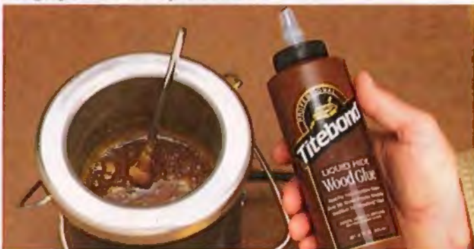
Some modern hide glues, such as Titebond's liquid hide glue, right, are made out of synthetic ingredients. To meet kosher standards, avoid traditional hide glues, left, made from animal by-products.
