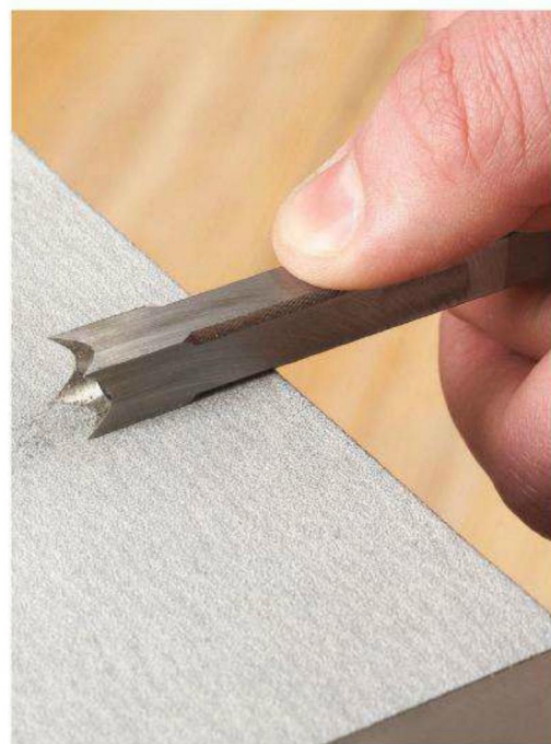
For an initial coarse sharpening, use adhesive-backed sandpaper to remove the burr. Switch to a 1,000-grit stone for subsequent honings.
