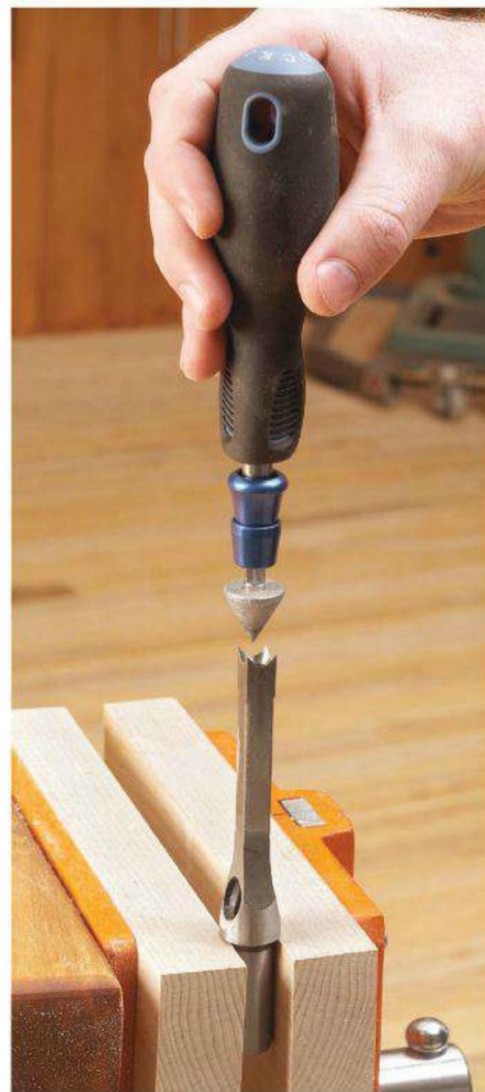
The cone-shaped sharpening stone seats itself in the chisel's bevel for fool-proof sharpening.
