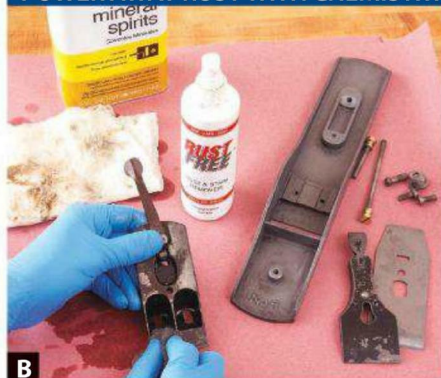
B Allow the rust remover to penetrate for 30 seconds before scrubbing with 0000 steel wool. Wipe clean with mineral spirits.
