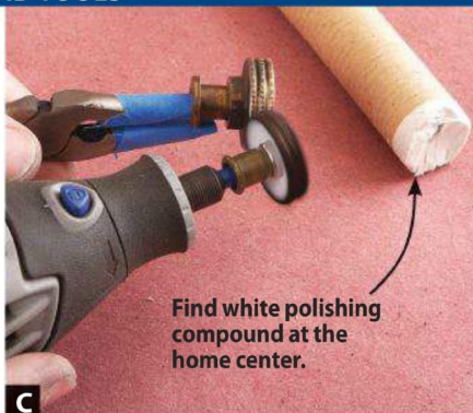
C A rotary tool or grinder with a polishing wheel makes quick work of shining brass knobs and nuts.
