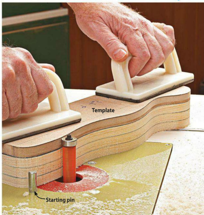
Bind multiple workpieces together with the template using double-faced tape. A starting pin helps anchor the stack when beginning the cut.
