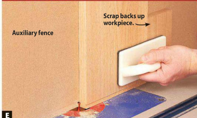
E Back up the workpiece with a scrap, then make a pass on each face. Move the fence back for a looser fit, forward for a tighter fit.
