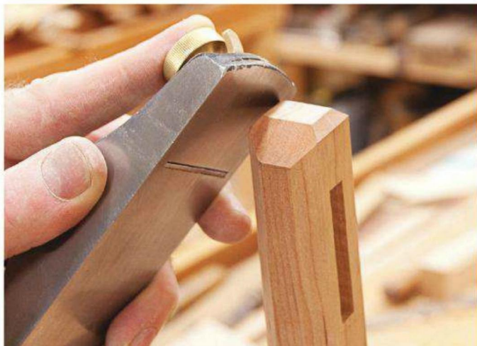
Chamfering the top of a dining-chair leg proves a snap when you use a sharp block plane. Setting up a router table for this task takes too much time.
