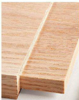
This tenon, also cut with a dado blade, will bond better because we removed the ridges with a shoulder plane.
