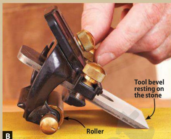
B The key to using a honing guide is to keep the roller and the tool's beveled edge in constant contact with the sharpening medium.
