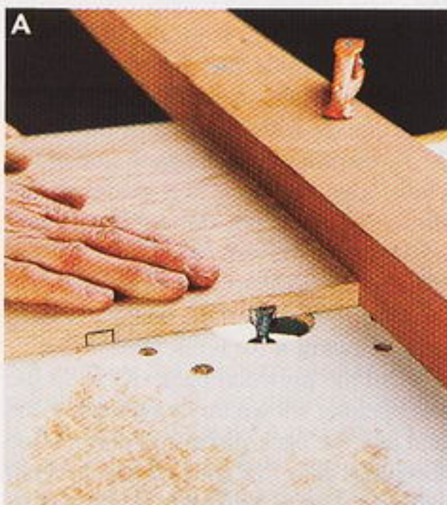
With a 1/2" dovetail bit, rout the first of three dovetail grooves in the side pieces.
