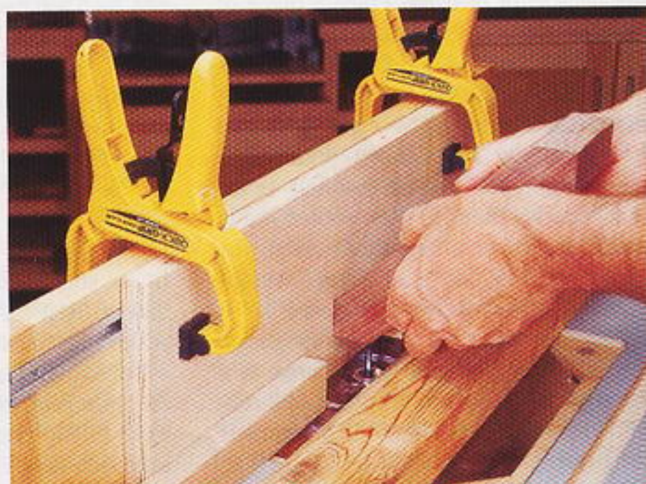
Cutting a spline slot is simple with this setup. Start at the right-hand stopblock, lower the workpiece onto the support guide, and slide it to the left stopblock.
