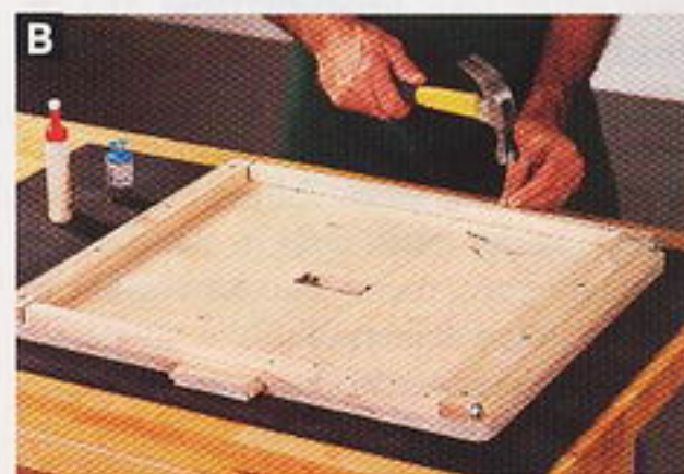
With the tables and spacers upside down, slide the all-thread rod through the clamp blocks and guides to align the pieces. Nail the guides in place.
