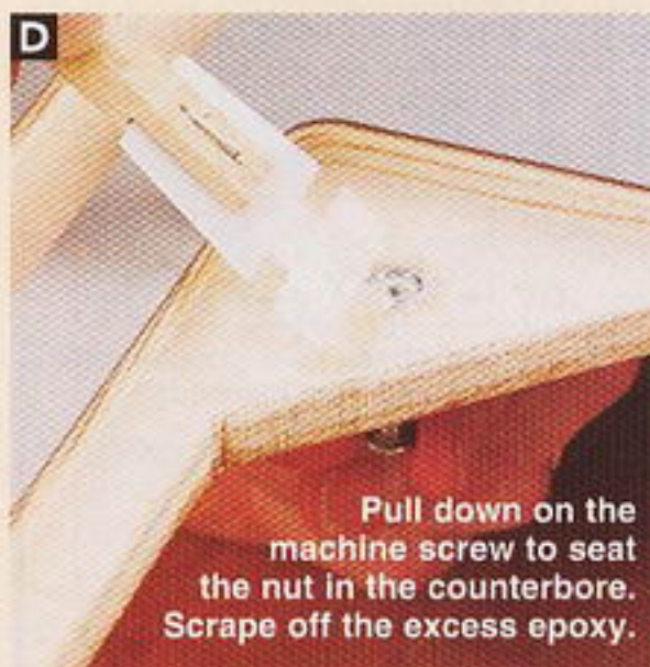
Mix some 5-minute epoxy. Fill the counterbore with epoxy while pulling up on the lock nut.
