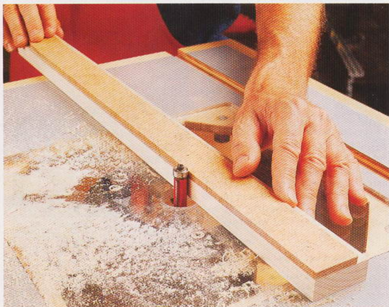
Cut the workpiece close to your template with a bandsaw before going to the router table. Trim bits are designed to handle light cuts only.
