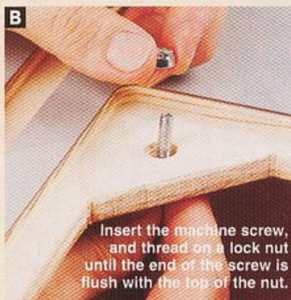
To keep the epoxy from sticking to it, apply petroleum jelly to a #10-24x2" machine screw.
