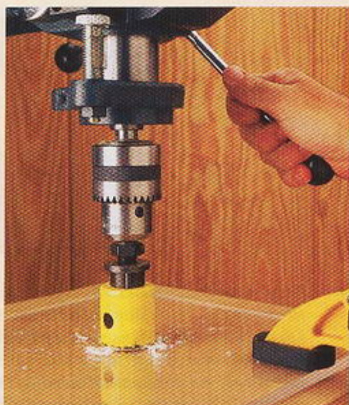
Clamp your insert-plate blank and a backer board to your drill-press table, centered under the bit of your holesaw. Drill slowly, and you'll get a clean cut.
