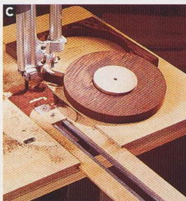
Using the guide is as simple as a twist of the wrist with our sliding trammel and taped-in-place trammel disc.
