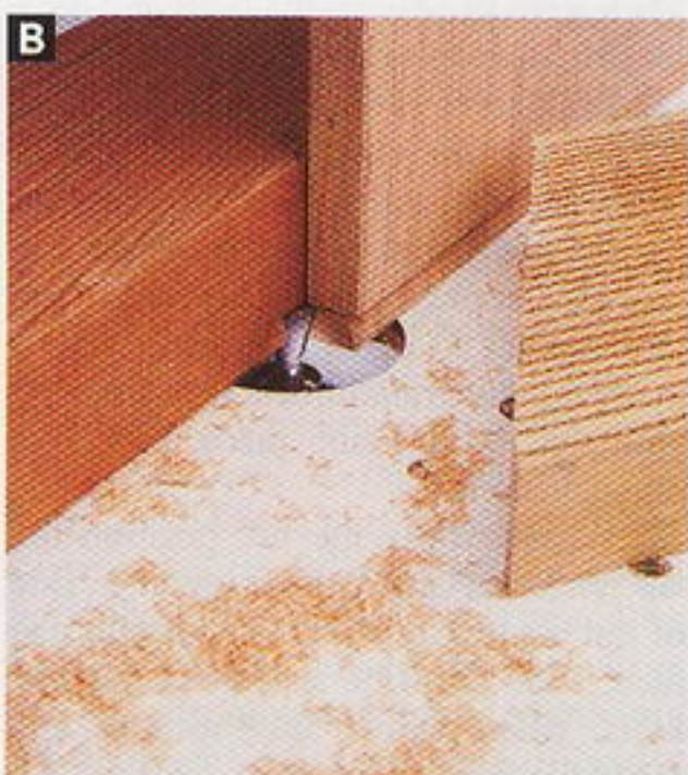
Rout a dovetail pin on one end of a drawer shelf, after testing on scrap wood.
