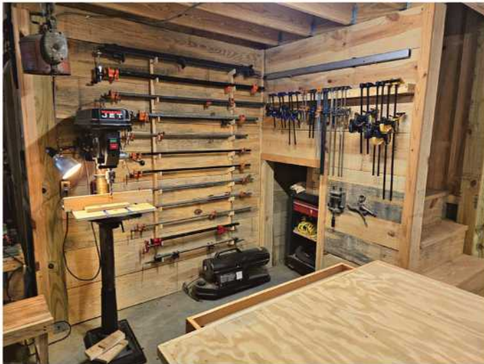
A side benefit to using rough-sawn lumber to line the walls is the rock-solid anchoring surface it provides for mounting custom storage racks.
