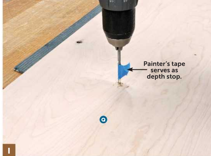
I Lay out and drill pilot holes in the underside of the top (Q) for screws to attach the lift hardware, taking care to avoid drilling completely through the top.
