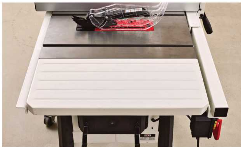
All of the saws (except for the Grizzly G0771Z) feature stamped steel wings like those on the Jet, pictured . Steel wings cut down on weight but lack the vibration-dampening qualities of cast iron.
