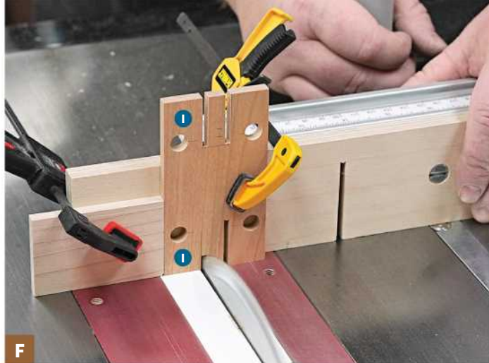
Use a stopblock clamped to your auxiliary miter-gauge fence to establish the edges of the doorway on each end of the ends (I) blank. Then make additional cuts to remove the waste between them.
