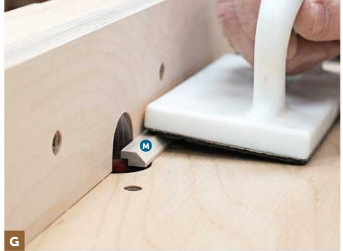
Use a push pad to guide the steps (M) blank past the router bit. If your router table has adjustable fence faces, move them as close to the bit as possible to keep the blank stable.
