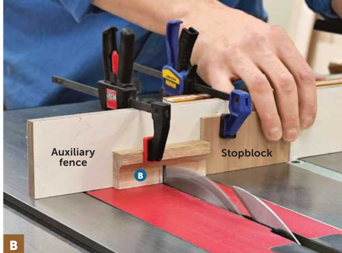
Line up and clamp a front/back (B) to cut one side of the notch. Add a stopblock and make the cut on both pieces. Adjust the stopblock and repeat to widen each notch.
