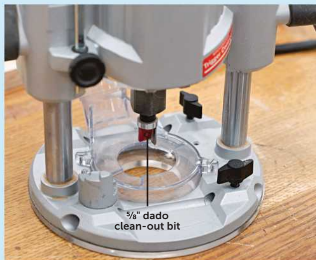
The bearing at the top of a dado clean-out bit matches the diameter of the cutter and rides along the guide rails of the jig.
