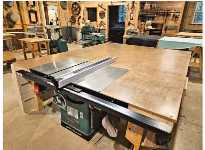
Paul surrounded his tablesaw with additional workpiece support, particularly for cutting sheet goods. The space underneath provides storage for jigs and accessories.
