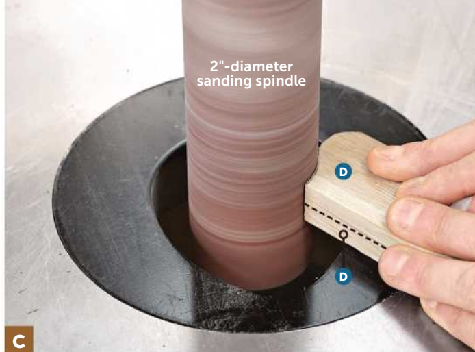
Keep the sides (D) taped face to face after bandsawing the curved shape close to your layout lines while you finish shaping with a spindle sander or a dowel wrapped in sandpaper.
