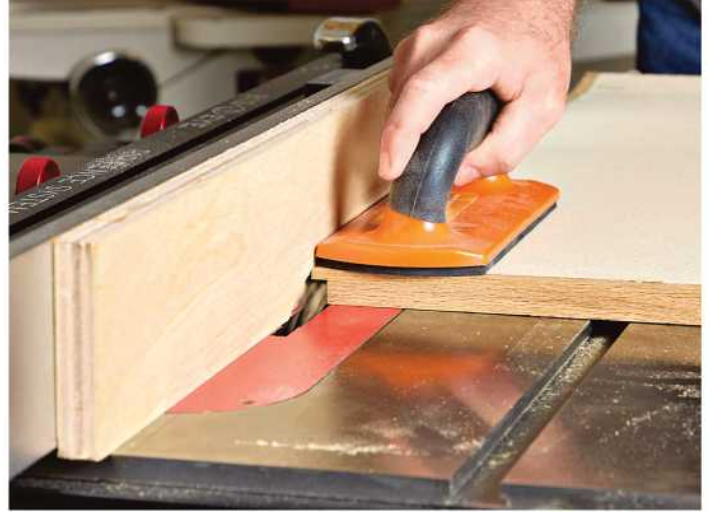
With the canvas facing up, rabbet the ends of the tambour assembly to form a tongue to ride in the track. Use a push pad over the blade to hold the tambour flat and keep the tongue thickness consistent.
