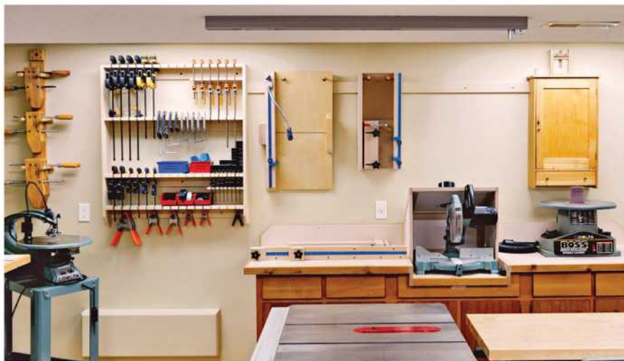
Tim thoroughly enjoys building jigs, fixtures, and custom storage racks for his shop. The French cleat hanging system provides a simple, sturdy method for mounting cabinets and racks.
