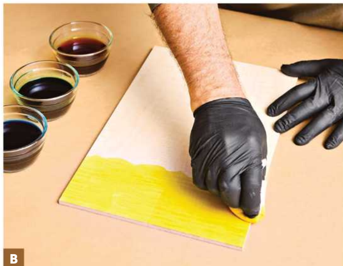
B To create a color gradient, start with the lightest color (in this case, yellow). Dip a clean rag into the dye and saturate the upper third of the board, applying a second coat if necessary.
