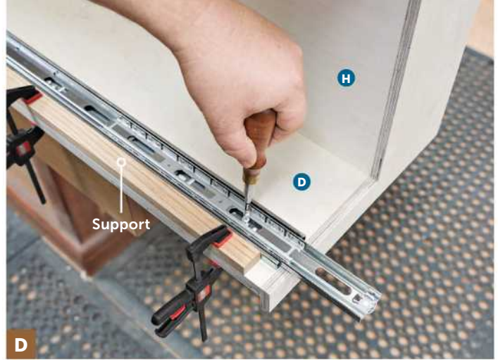
With no bottom to the sink drawer, there's plenty of access for installing the cabinet half of the drawer slides.
