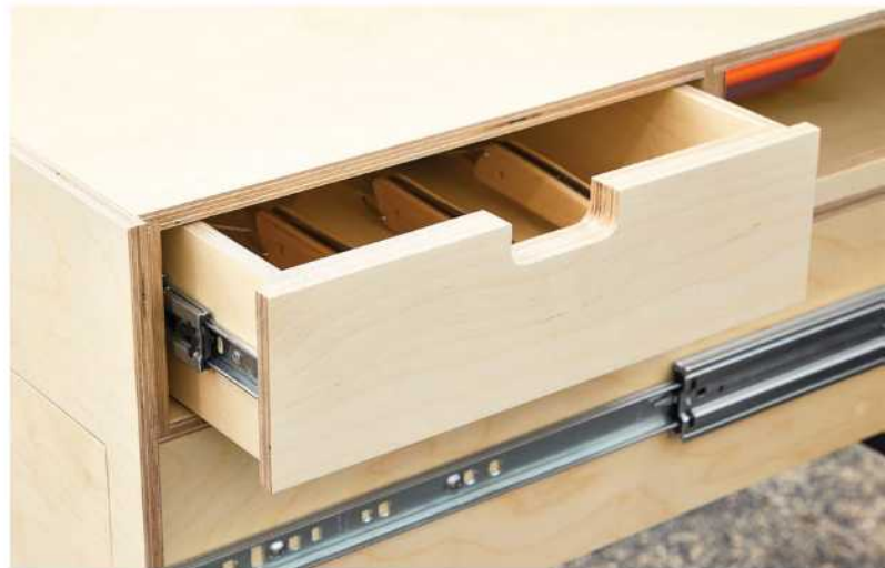
With no bottom to the sink drawer, there's plenty of access for installing the cabinet half of the drawer slides.
