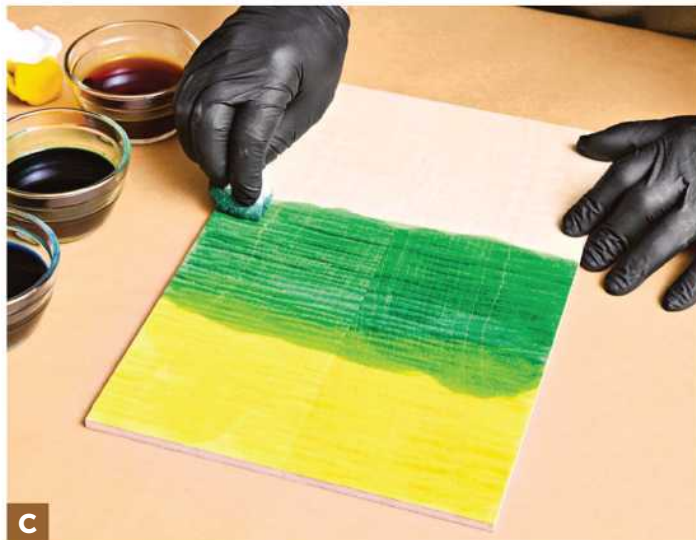
C Add the second color (green) to middle third of the panel, slightly overlapping the first color.
