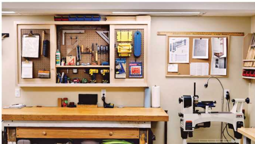
Tim's dad built this workbench 60 years ago. Tim added the large drawer and a hardwood top salvaged from an old building. The cabinet above is equipped with sliding doors for easy access.
