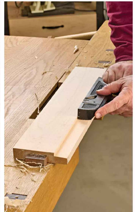
Place the plane on its side to trim the shoulder of a rabbet. Most rabbet planes can be used from either direction, depending upon the grain direction.
