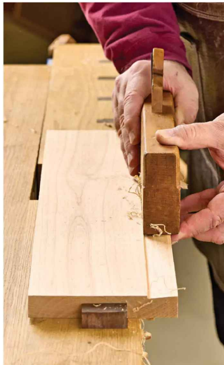
Widen the cut by taking additional passes, gradually returning the plane to an upright position. Use your fingers as a fence to help regulate the rabbet's width.
