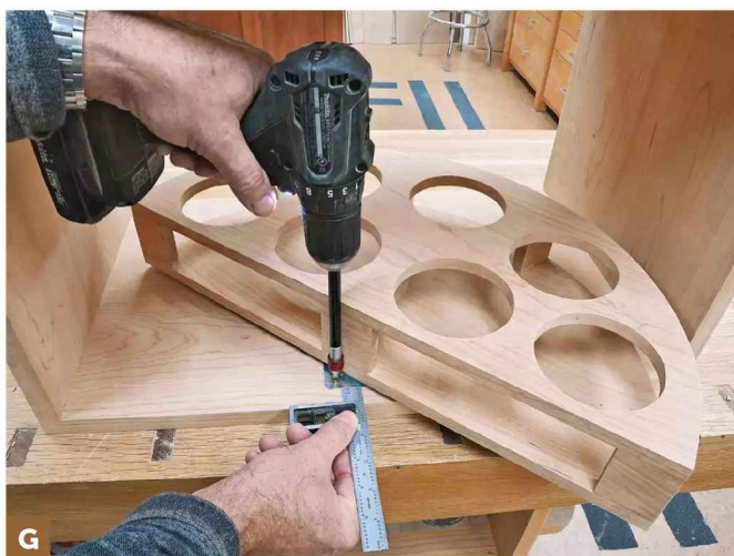
G Position the bottle rack assembly ¾" from the front of the case and centered side-to-side. Screw the bottom plate of the lazy Susan to the bottom of the case, rotating the bottle rack to reach each screw.
