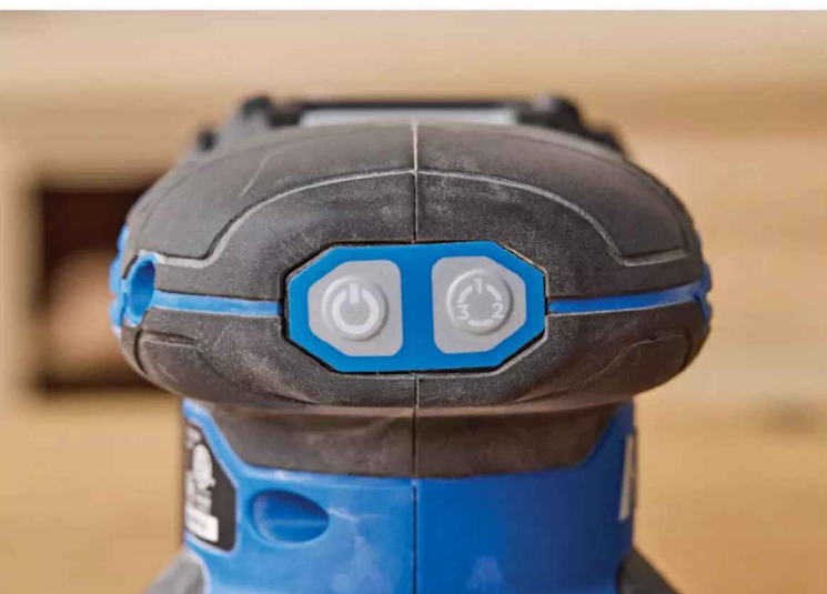
Because the soft-touch switches on the Kreg sander look so similar, it's difficult to distinguish between the power button ( left ) and the speed control button ( right ) from a casual glance.
