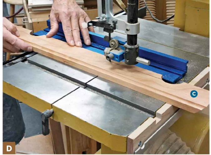
Position the bandsaw fence ¾" from the far side of the blade and trim off the lower edge of each base part between the half-circles.
