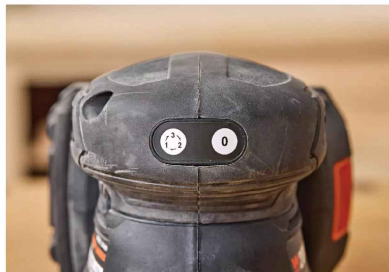
We found the poor labeling and separate power-on ( left ) and power-off ( right ) buttons on the Wen sander confusing. The power-on button also controls the motor speed.
