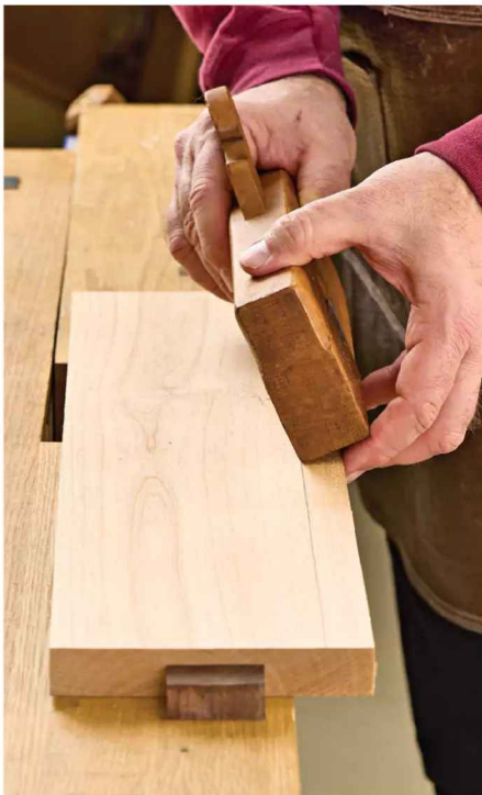
With the plane slightly tilted, place the corner of the blade in the scribed layout line and cut a narrow furrow along the shoulder of the rabbet for the plane to ride in.
