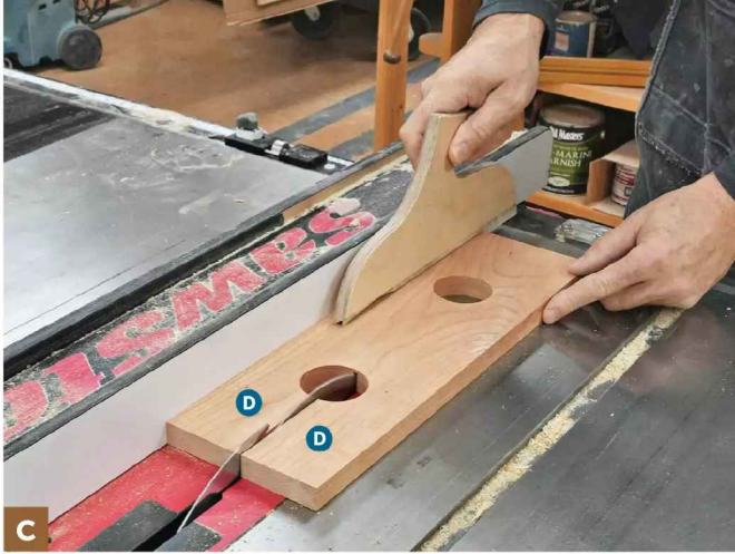
Ripcut each base blank down the center to form two 2½"-wide base fronts/back (C) as well as two base ends (D).
