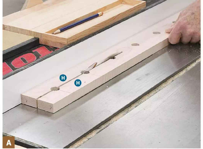
A After drilling the holes in the shelf standard (H, I) blanks, rip the blanks in half to create the semicircular notches that accept the ends of the shelf cleats (J).
