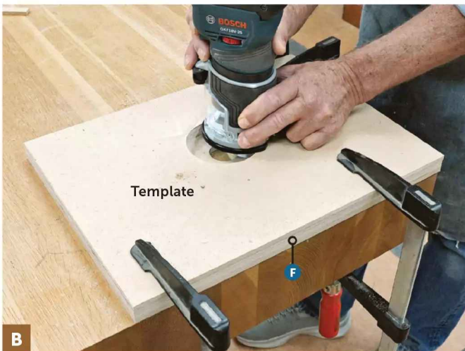
Clamp a hardboard template to the top (F) flush with its edges and use a pattern bit to rout the 3/8"-deep recess for the router base. Rout the recess in stages, lowering the bit between passes.
