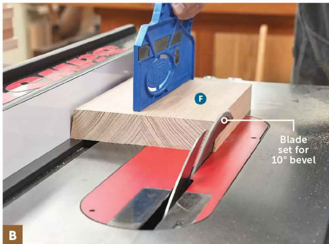
Tilt the tablesaw blade 10° and set the fence to bevel-rip the box ends (F) without reducing their width. Cut one edge, flip the stock over, and bevel-rip the other edge, ensuring the angles are parallel.
