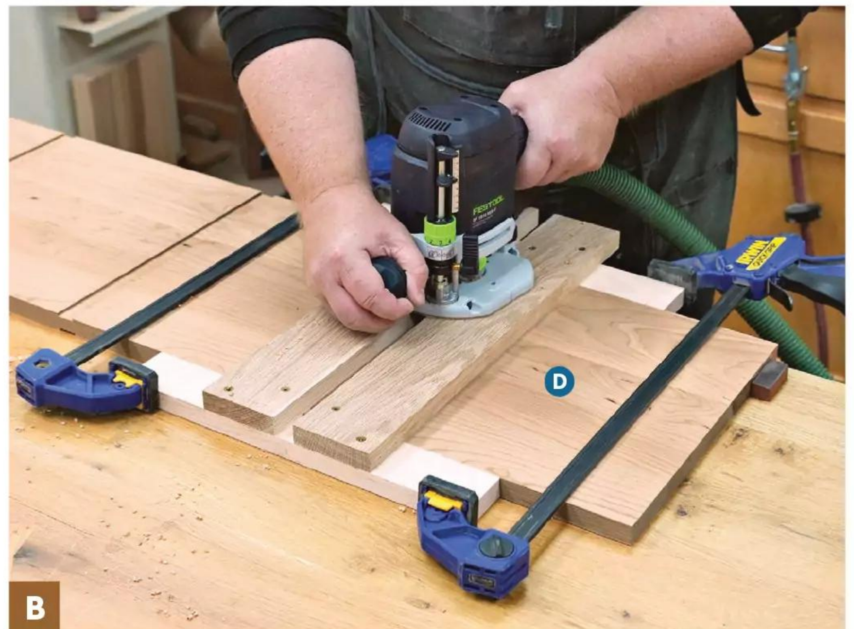
Remove the stop from the jig and move the back cleat in by 1/2" to straddle the top (B), drawer shelf (C), shoe shelves (D), and bottom (E) as you rout the 1/8"-deep through-dadoes.
