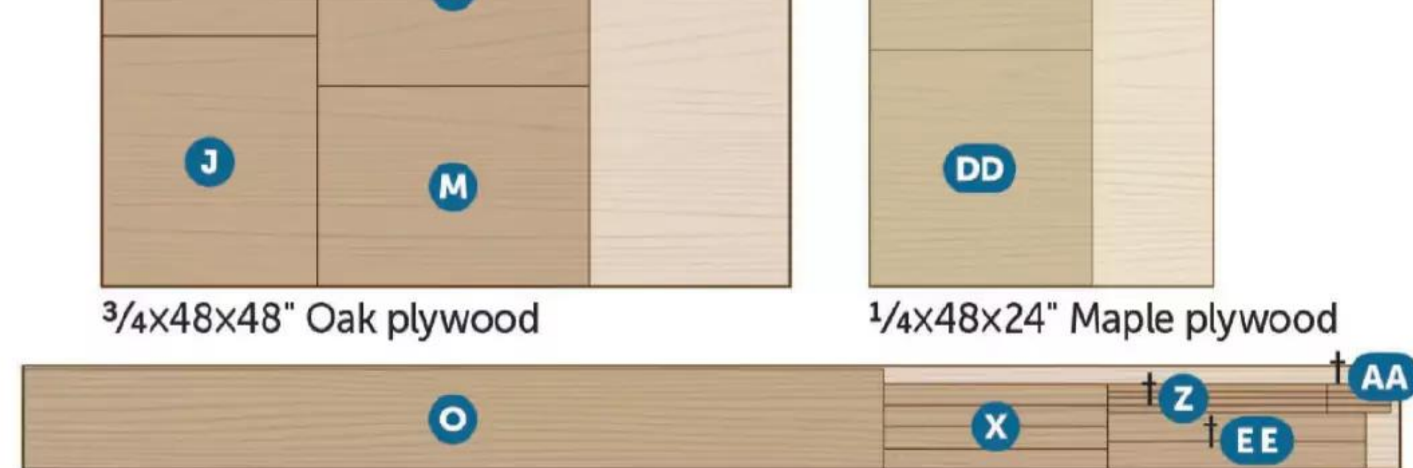
3/4x7 1/4x96" Oak †Plane or resaw to the thickness listed in the Parts List.
