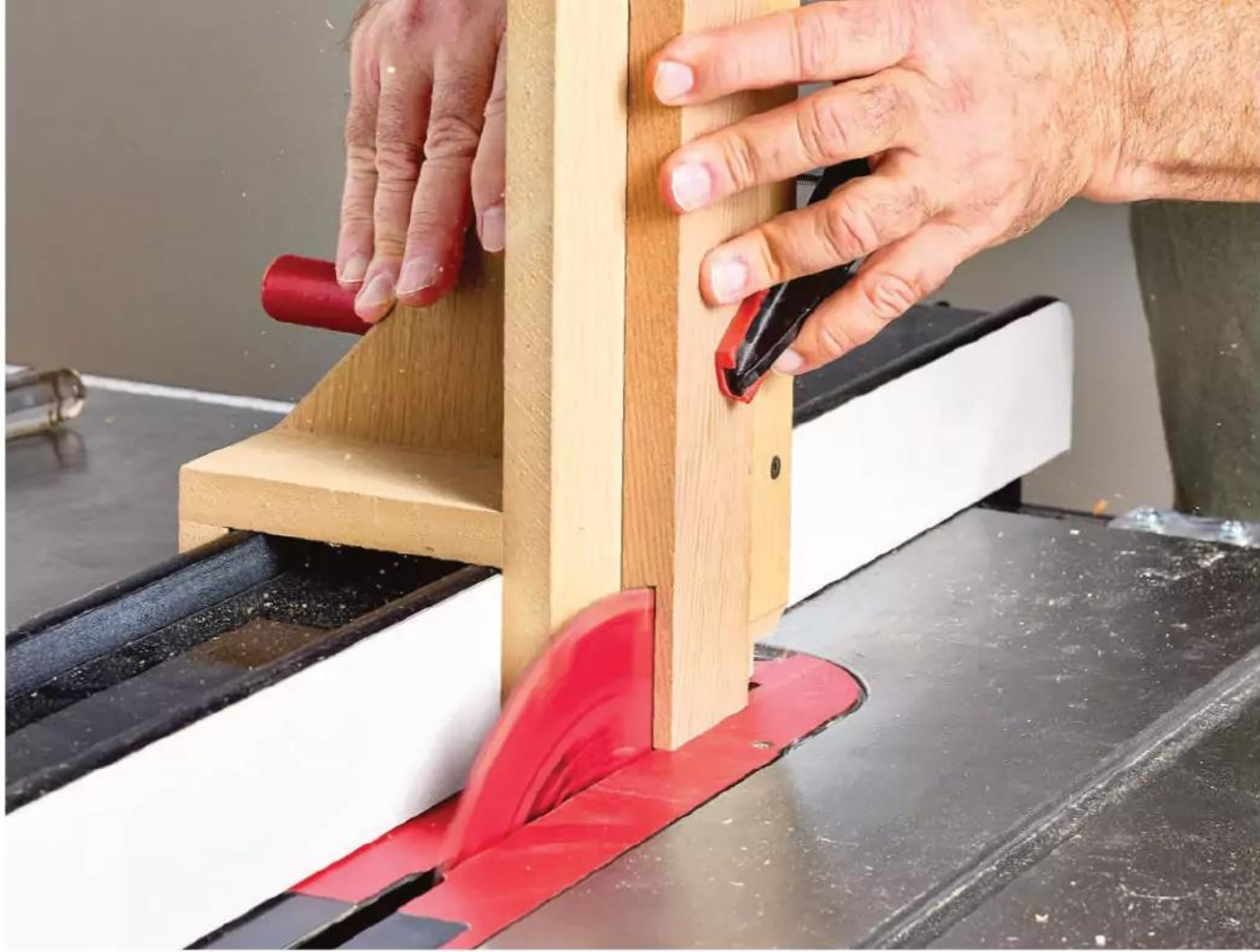
Raise the blade to match the width of the tenon workpiece. Then with the mortise workpiece clamped to a jig for support, cut the first wall of the open mortise.
