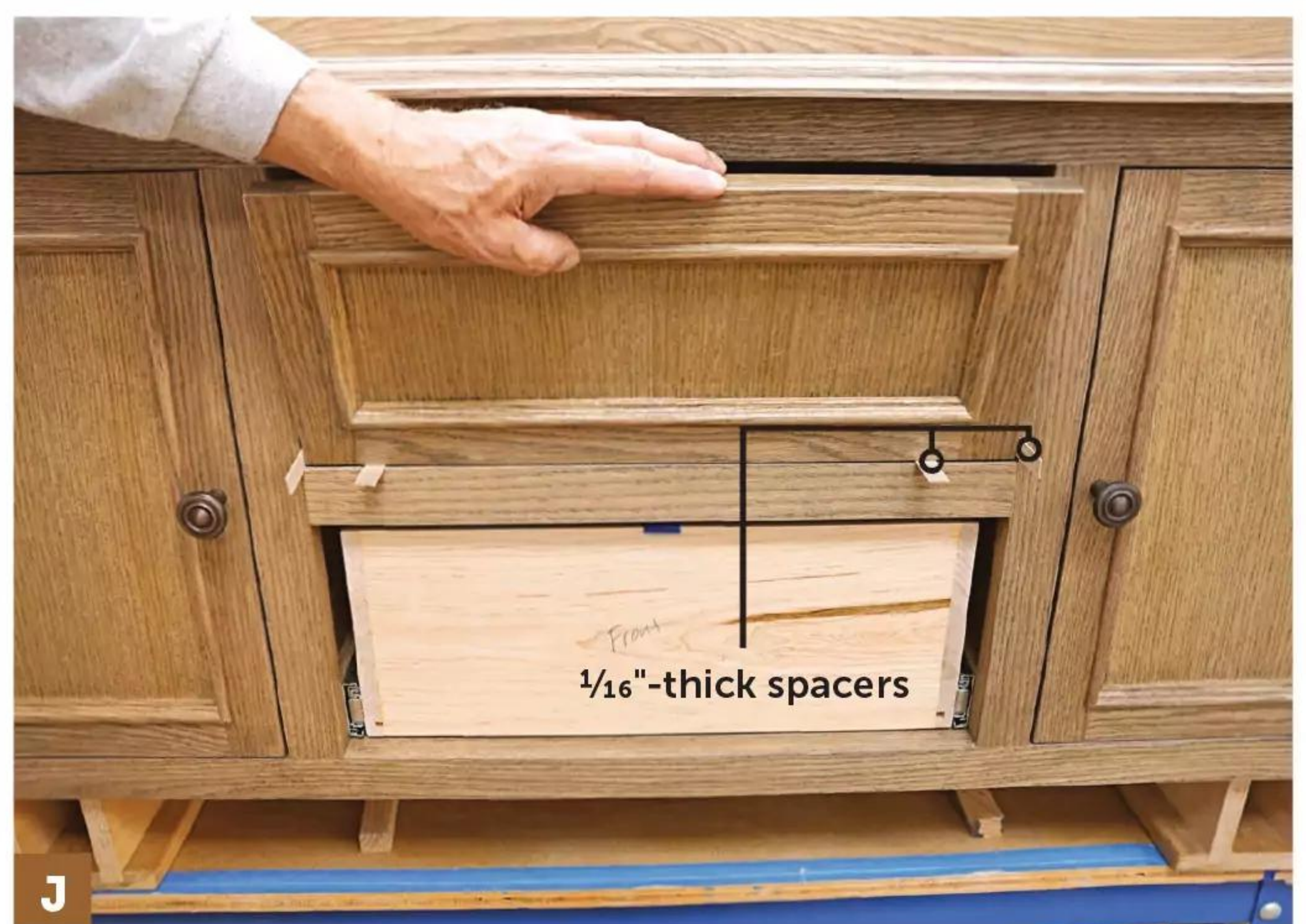
J Apply double-faced tape to the back of the false front's rails. Place \frac{1}{16} " spacers underneath the front and on each end to position it in the drawer opening. Then adhere the false front to the drawer box.
