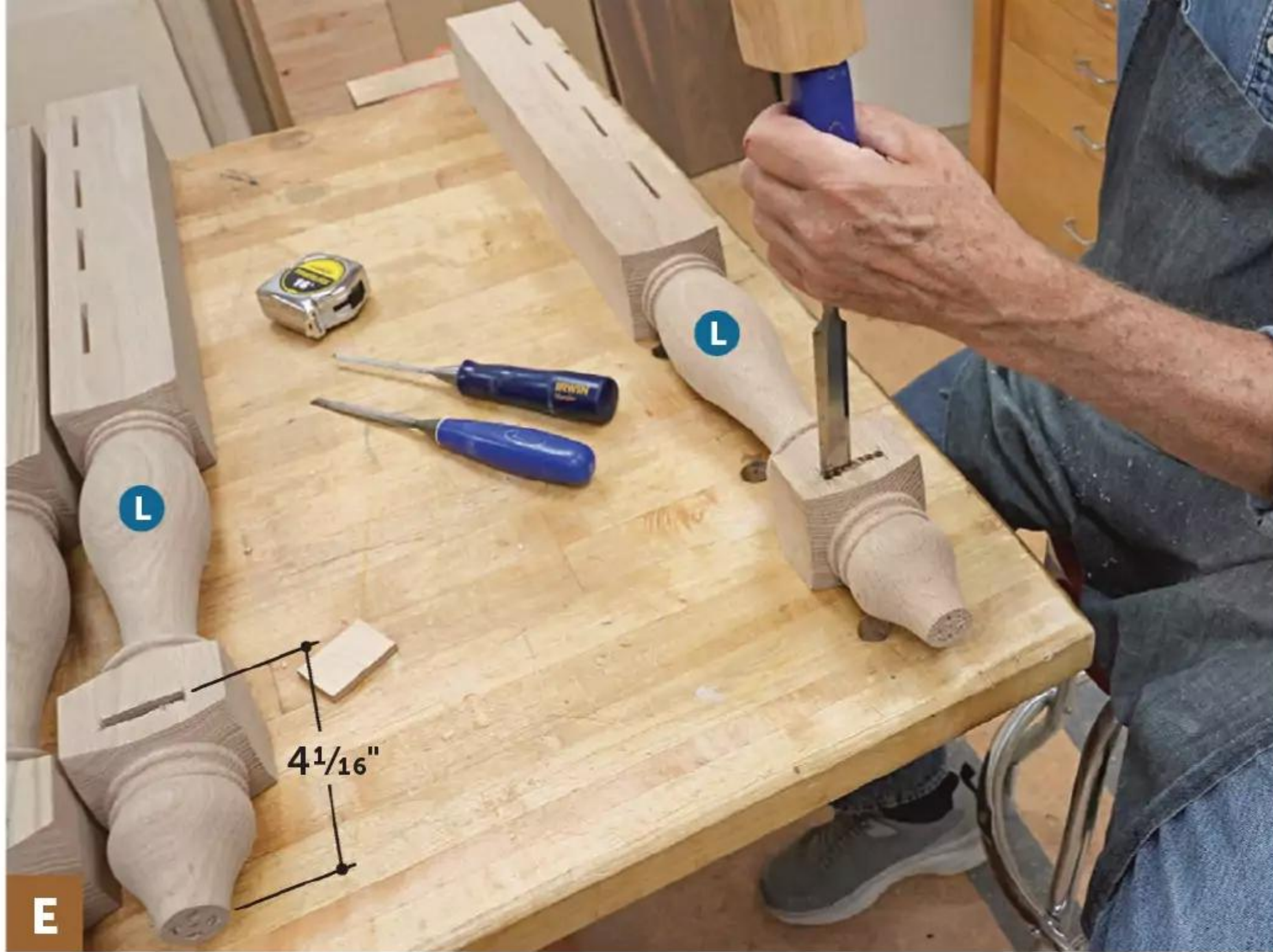
E On the leg face with biscuit slots, drill out a \frac{1}{4} \times 1\frac{1}{2} " mortise, \frac{3}{4} " deep and centered 4\frac{1}{16} " from the bottom of the leg. Use a \frac{1}{4} " chisel to square the mortise ends and a wider chisel to smooth out the sides.
