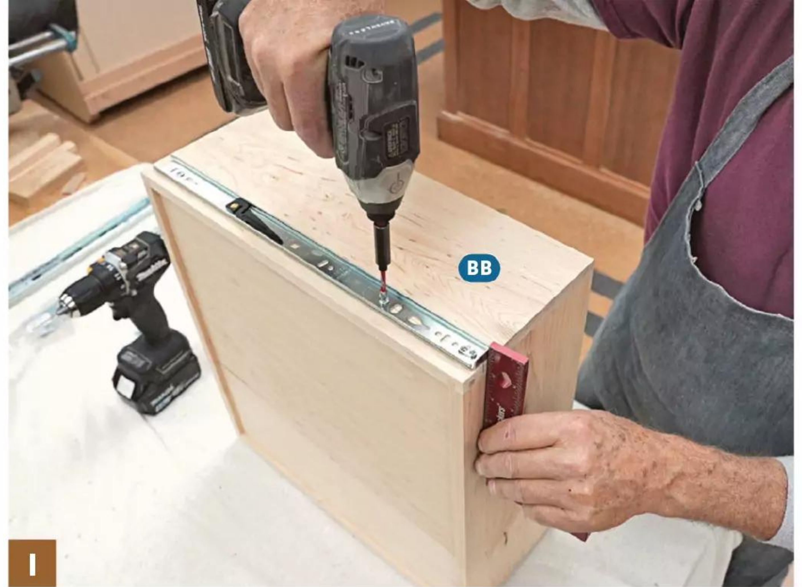
I Draw a line on the drawer box sides \frac{7}{8} " from the bottom edge. Center the mounting holes in the slide on the line and make sure the front of the slide is flush with the front edge of the drawer box.
