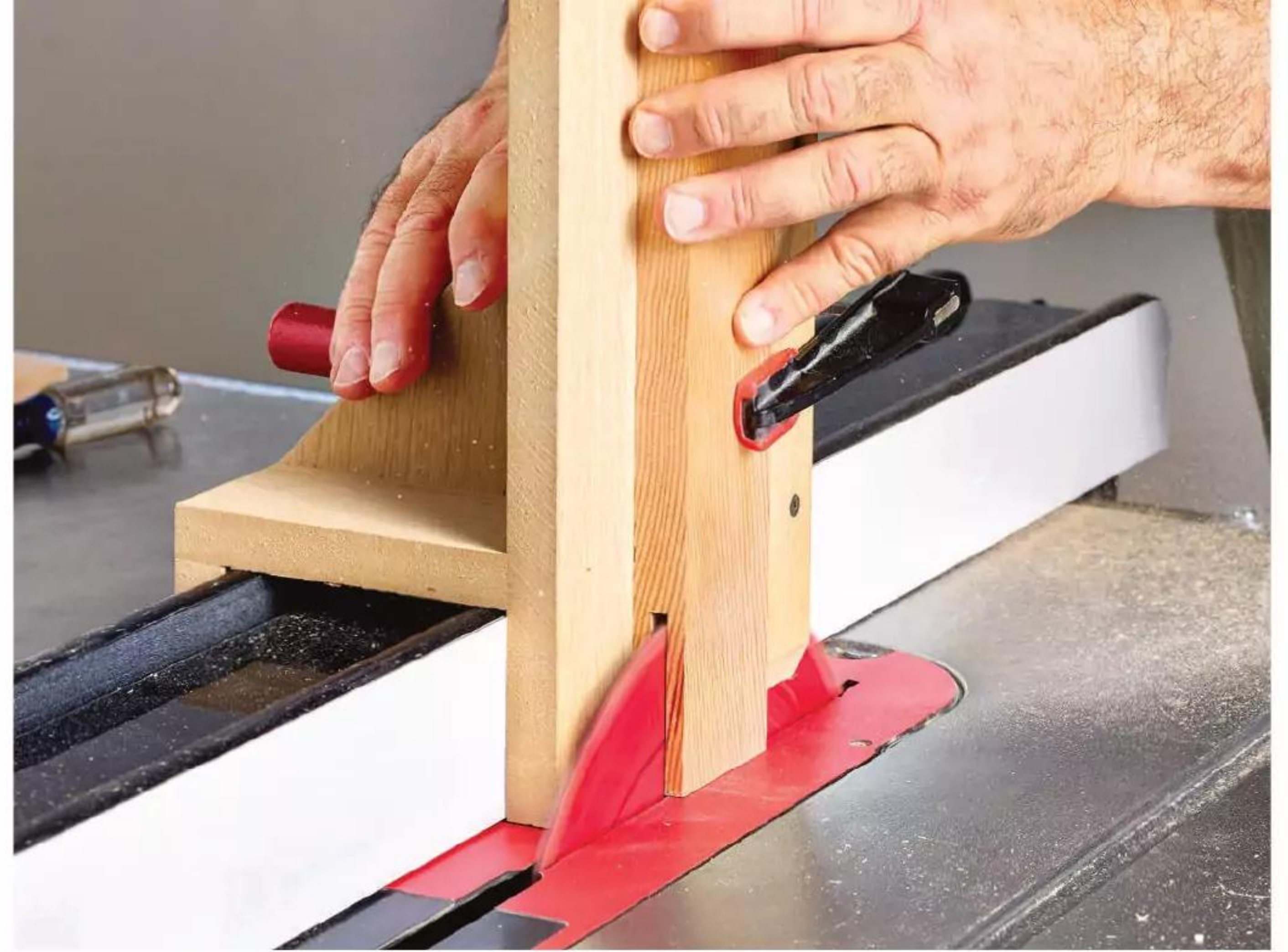
Flip the workpiece around to cut the second wall of the mortise. If any waste remains between the two cuts, reposition your rip fence and make additional passes to remove it.
