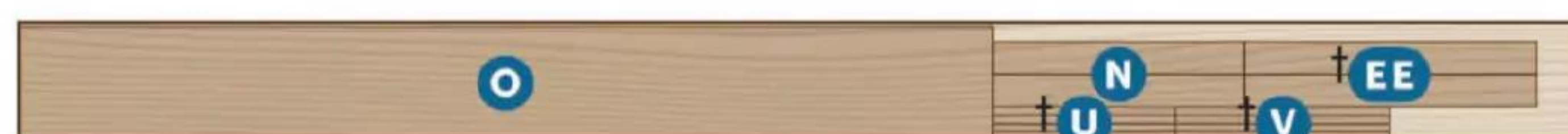
3/4x7 1/4x96" Oak †Plane or resaw to the thickness listed in the Parts List.
