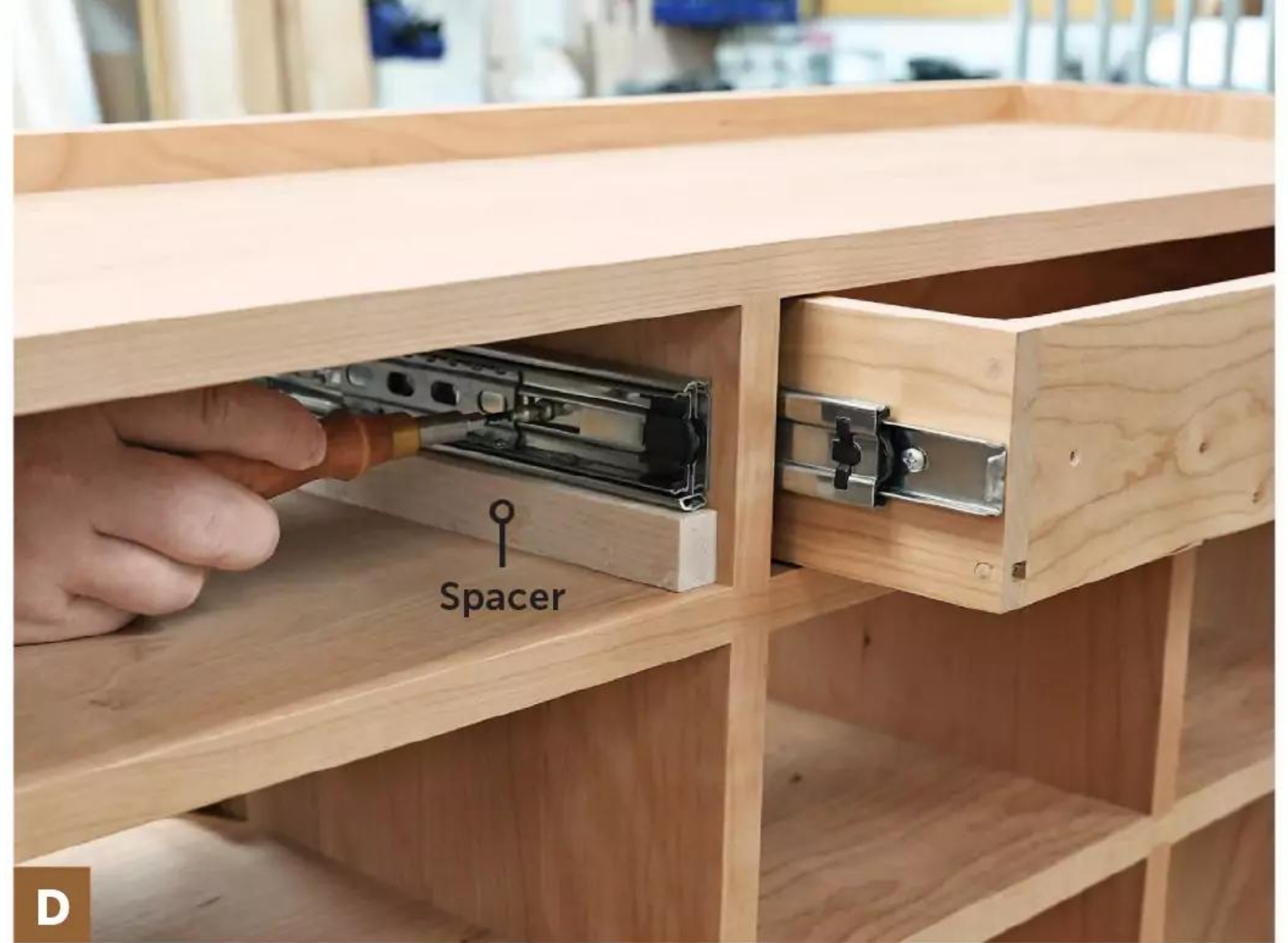
With the slide resting on a 1 1/8"-wide spacer, install the drawer slides 1/2" back from the front edge of the drawer divider (I) and sides (A). Use the slotted screw holes so you can make any adjustments.
