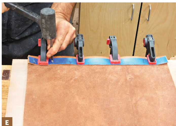
Fold over 1\frac{3}{8} " of the end of the leather, suede side to suede side, and clamp it to a piece of scrapwood. Then use a 3mm hole punch and a hammer to cut holes, where marked, through both layers of leather.
