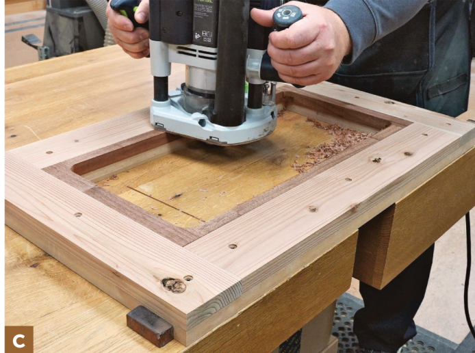
Secure the jig with bench dogs or clamps. If you use clamps, you'll need to stop and reposition them as you work around the assembly.
