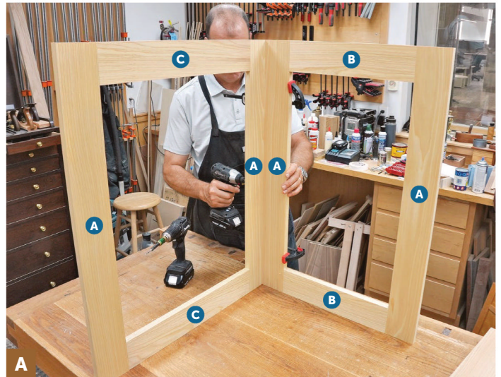
With the back frame (A/C) glued and clamped to one side frame (A/B), drill countersunk pilot holes through the rear frame stile into the edge of the side frame and drive exterior-grade screws.
