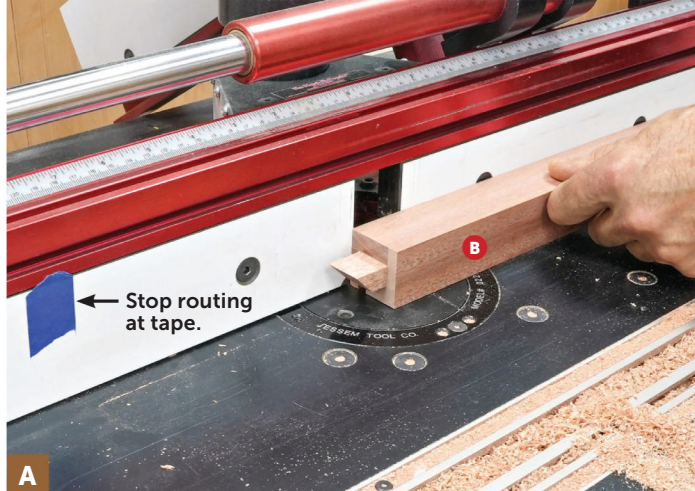
Route a 1/4" stopped groove 1/4" deep in the upper stretchers (B). A piece of tape on the router fence shows you where to stop the groove cut. Reset the fence to make the cut on the mirror-image piece.
