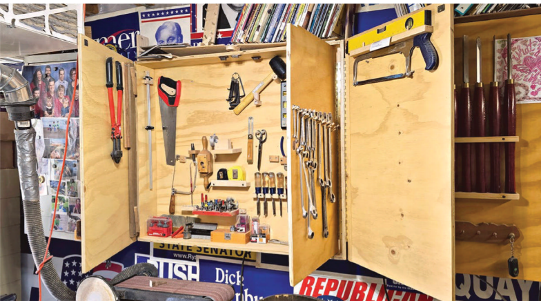
An interior hinged partition vastly increases the amount of square footage available for hanging tools. Magnetic catches hold the partition and doors closed.
