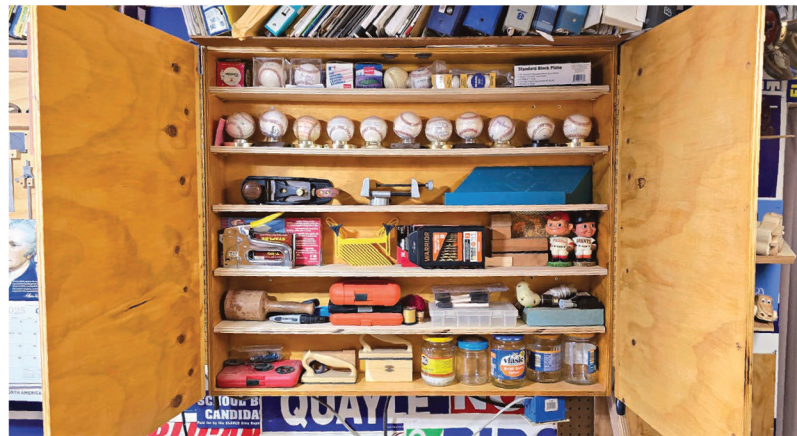
A simple plywood wall cabinet houses Chuck's small tools and supplies, along with his treasured baseball collection. Sturdy continuous hinges support the doors.
