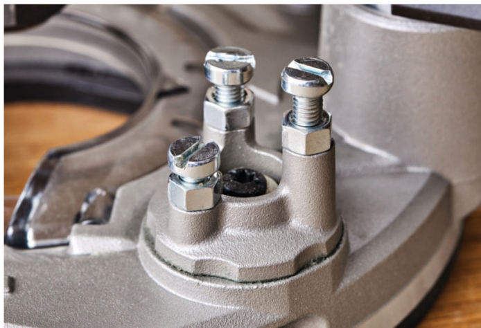
Turrets with screw stops (like those on the Metabo, shown , Makita, and DeWalt routers) allow you adjust the stop height. But it's difficult to access the screws and they can work loose inadvertently.
