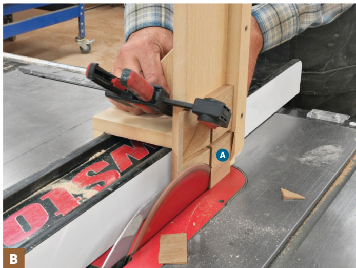
Position the rip fence so the inside face of the blade just intersects the bottom of the dado along the outside edge of the base (A). Rotate the base 90^\circ between passes to cut the four bevels.
