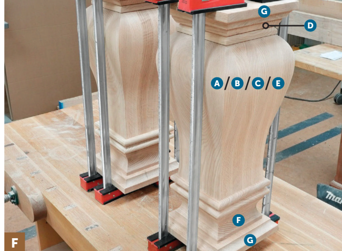
Glue the additional layers—the cove blocks (F), the large chamfer blocks (D), and fillet blocks (G)—to the pedestal assembly. Keep glue about 1/8" from the edges of each block to minimize squeeze-out.
