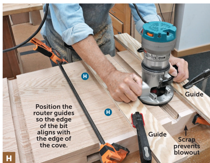
Install a 1 1/2" core box bit in your router and measure from the edge of the bit to the edge of the base. Clamp the bases (H) together with scrap on each edge, then clamp guides in place and rout the cove.
