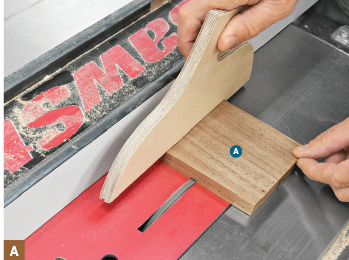
Make test cuts in a scrap the same size as the base to ensure the blade is centered on the workpiece. Then cut a groove and intersecting dado in the base (A).
