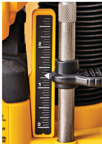
The scale and pointer on the DeWalt router, left , are clear and easy to read. The imperial scale on the Metabo router, right , is partially obscured by the depth rod.
