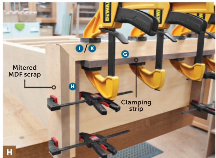
Using the mitered MDF scraps again, glue the front crown assembly (I/K) to the case. A \frac{1}{2} "-thick clamping strip fills the offset between the molding and the case to provide a solid footing for the clamps.
