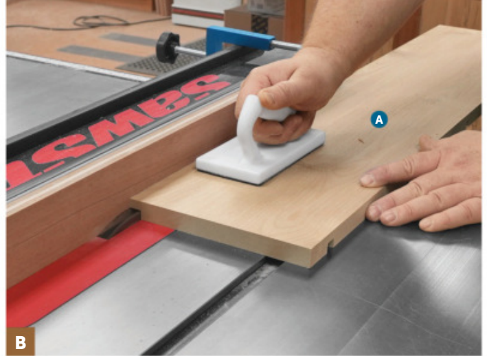
Clamp an auxiliary face to your rip fence and position it just touching the dado blade. Cut a rabbet on the inside back edge of each side (A), creating a mirrored pair.
