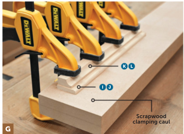
Keeping the square edges flush, glue the cove moldings (K, L) to the round-over moldings (I, J). A thick clamping caul makes it easier to position the clamps on the small moldings.
