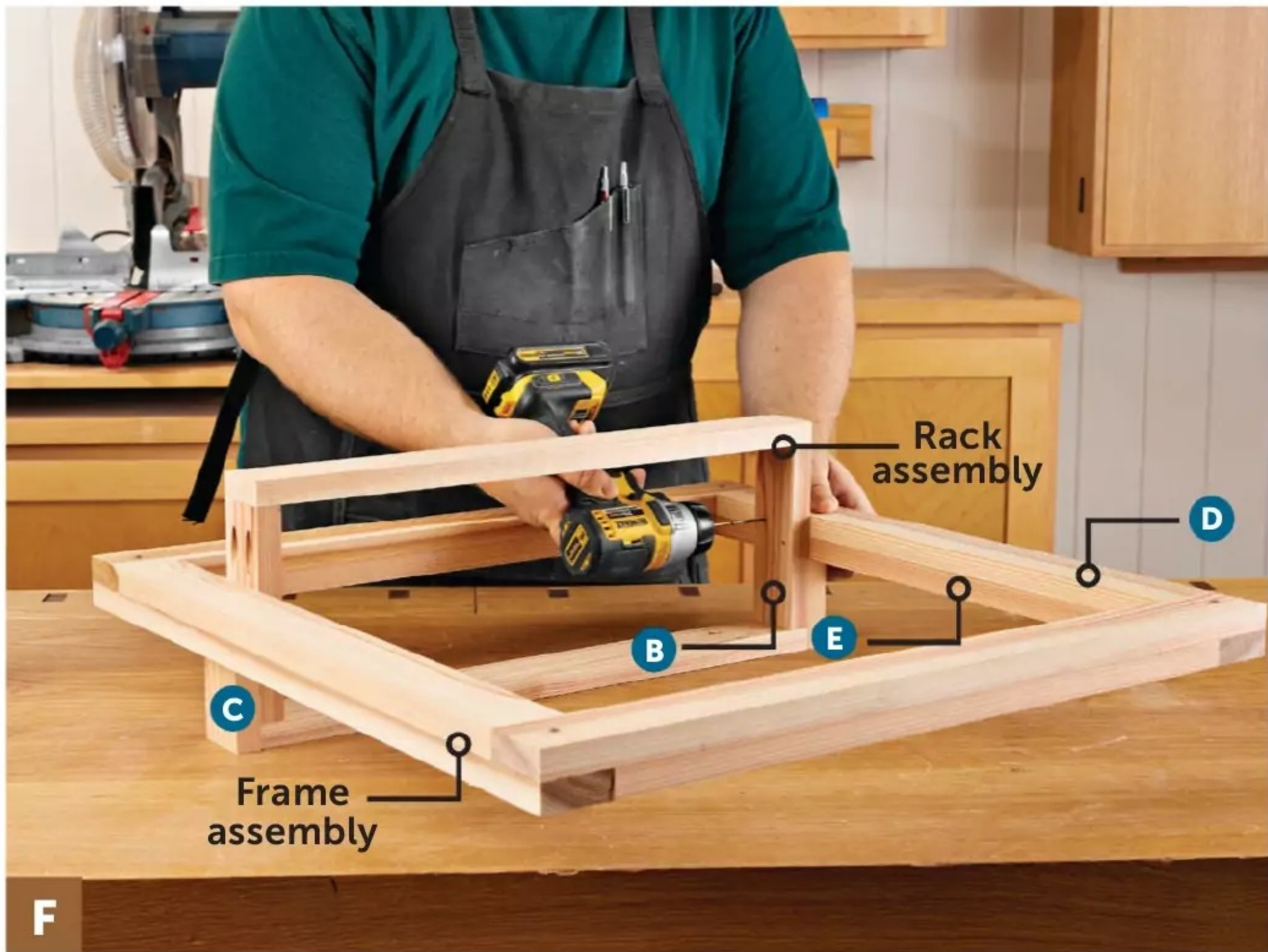
Attach the rack 3 1/4" from the bottom rail of the frame assembly with glue and exterior-grade trim screws. Stagger the screws to avoid the joint line between the two halves of the frame.
