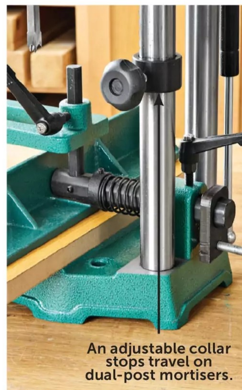
Collars on two-post machines like the Grizzly T33127 (left) work well with adequate tightening. The Grizzly G0645 (right) and the Delta use a hooked stop that comes to rest on top of the post and flexes easily.
