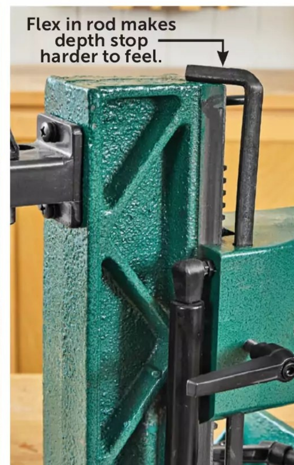
Collars on two-post machines like the Grizzly T33127 (left) work well with adequate tightening. The Grizzly G0645 (right) and the Delta use a hooked stop that comes to rest on top of the post and flexes easily.
