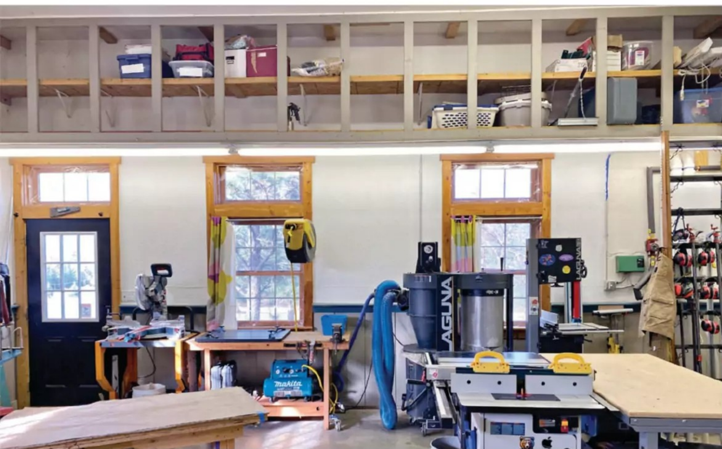
The 14'-high ceilings allow room for two levels of storage cubbies above the work area and a place to mount LED lighting fixtures to illuminate the work area.
