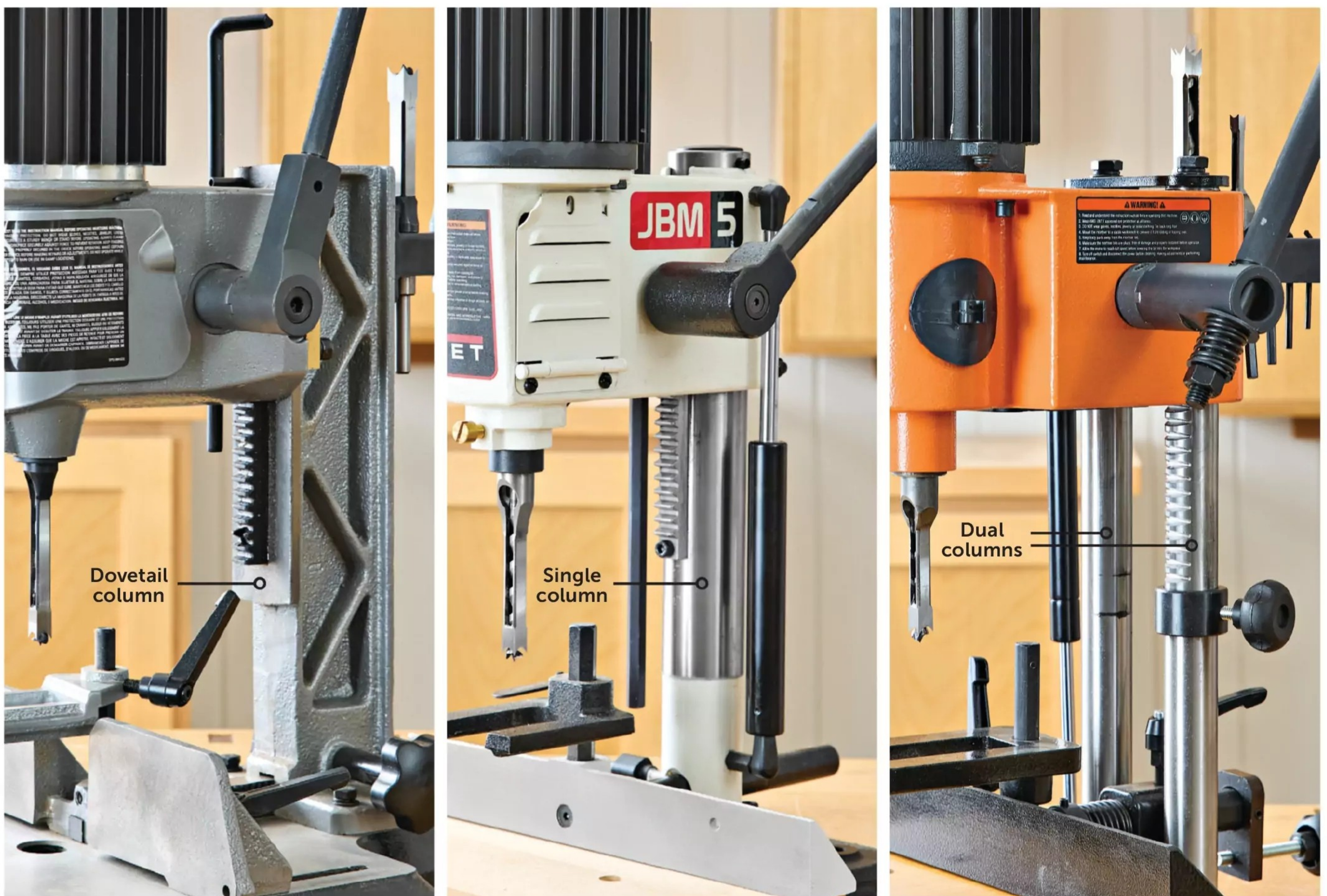
Dovetail-columns ( left ) offer precise vertical movement of the powerhead and are adjustable to remove side-to-side play. Jet's cylindrical single column ( middle ) also allows play adjustment. Dual-column machines ( right ) rely on column positioning to prevent powerhead side-play.
