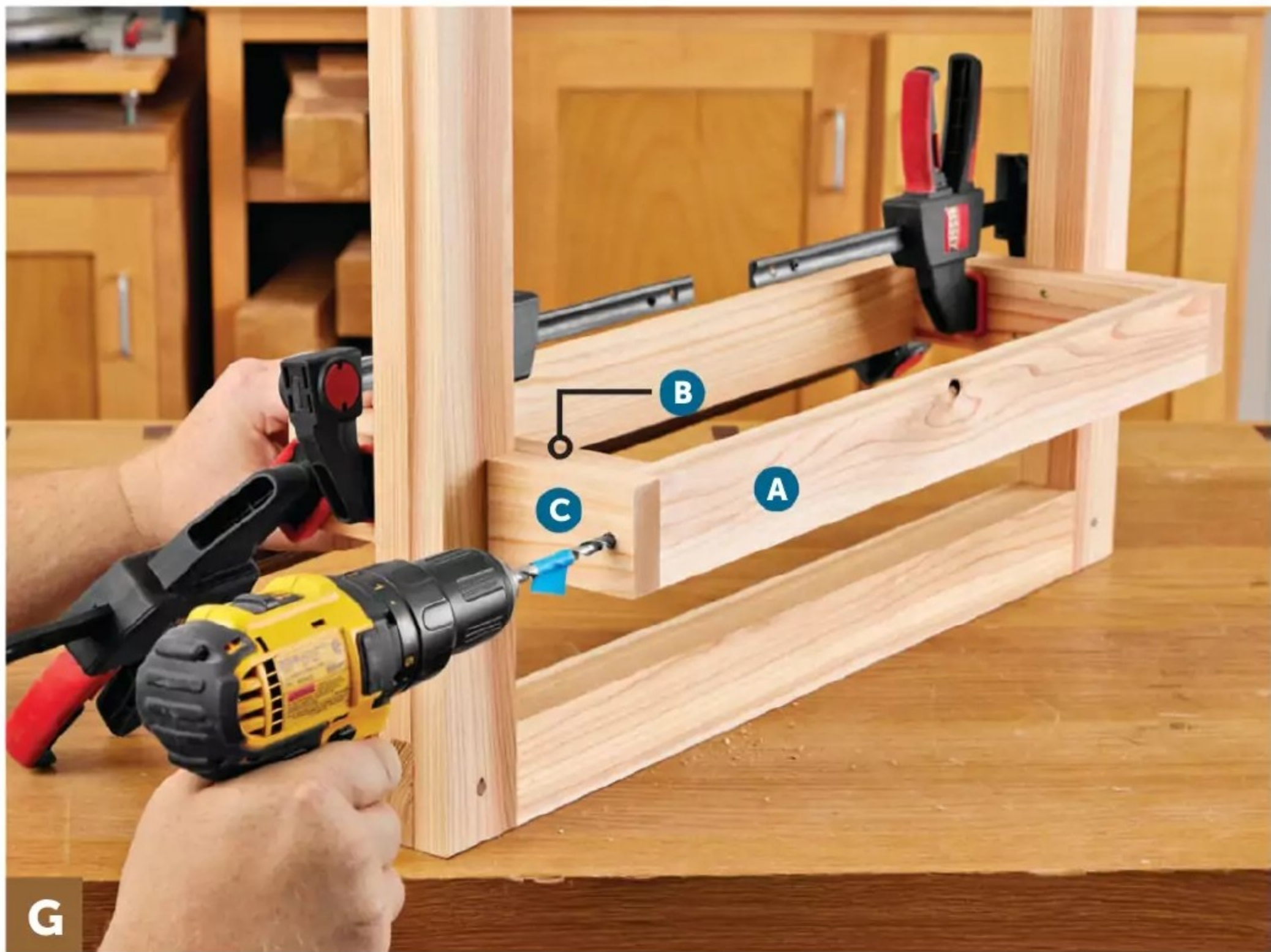
Glue and clamp the remaining end caps (C) to the rack assembly. After the glue dries, remove the clamp, drill holes, and drive a dowel pin into each corner.
