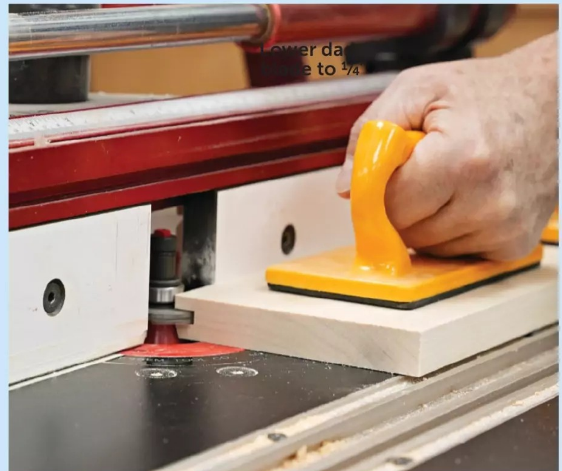
Adjust the bit height and fence to cut a centered groove, \frac{7}{16} " deep, in each rail and stile.
