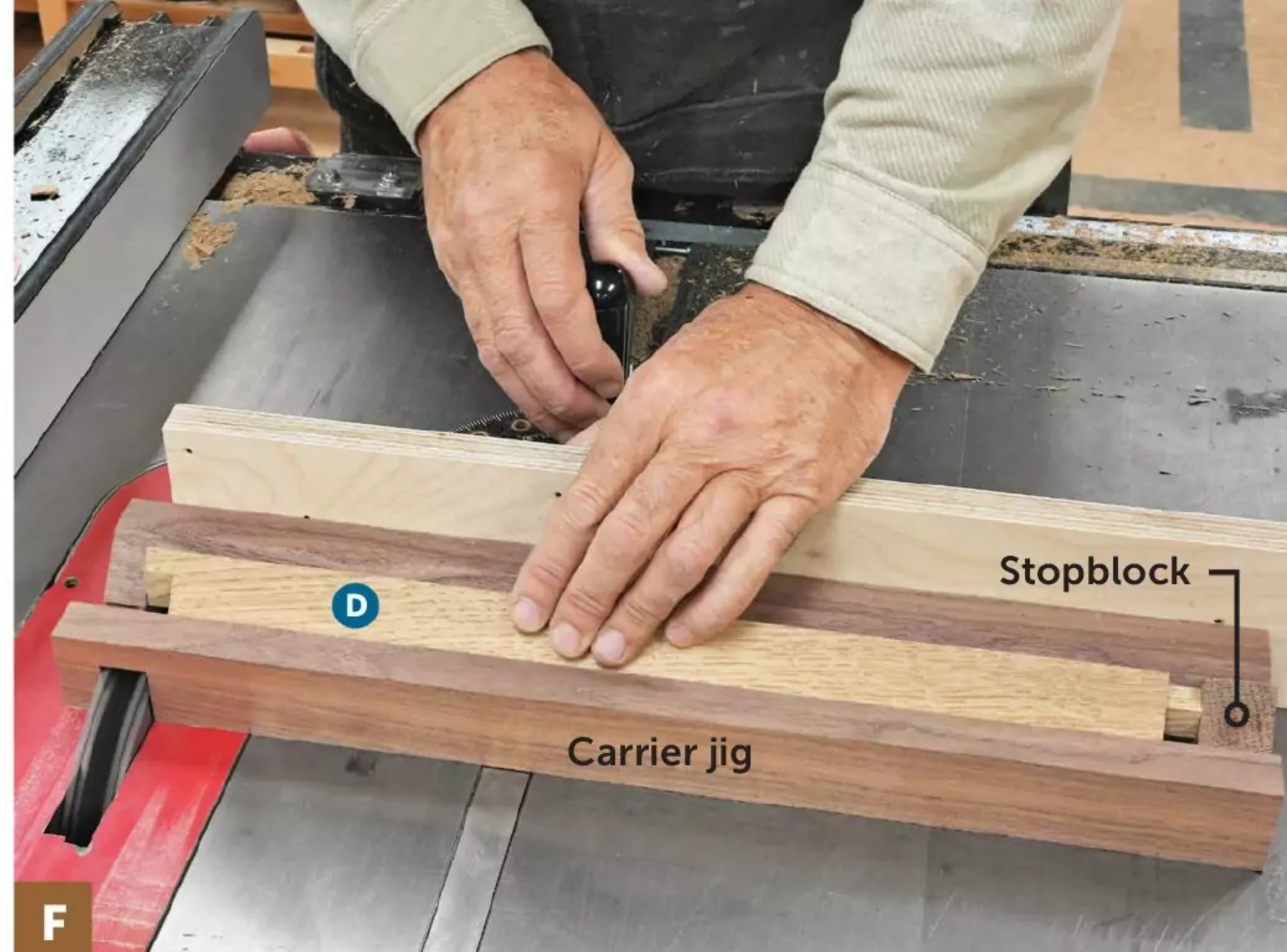
Attach a stopblock to the carrier jig to establish the \frac{1}{2} " length of the tenons. Make a pass on all four sides of the crossbar (D) to create the centered tenon. Repeat on the opposite end.
