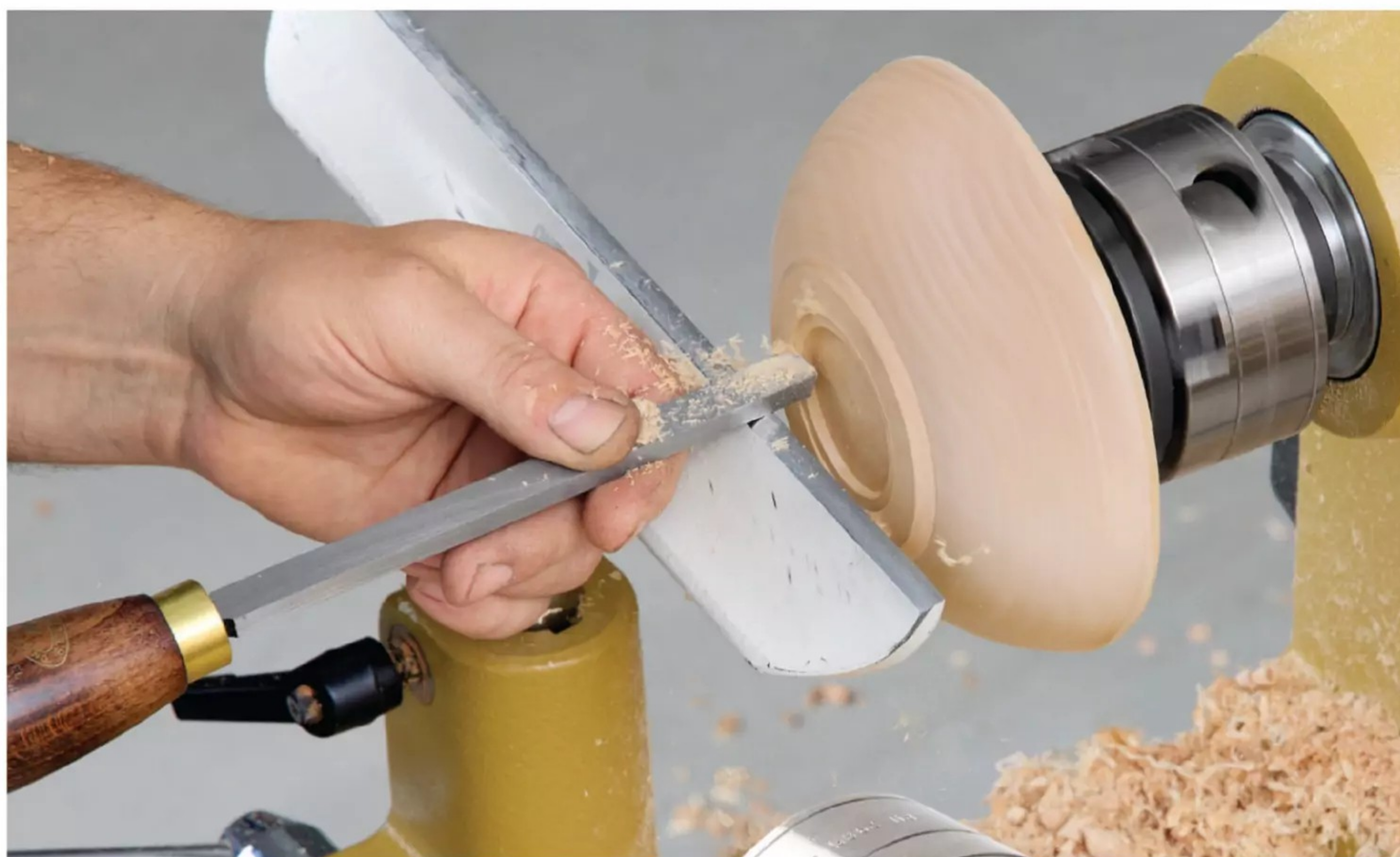
A four-jaw chuck can grip a tenon formed on the top face of a bowl blank as you shape the bowl's exterior. Use a square scraper to carve a recess on the bottom, then flip the bowl around so the jaws can expand outward to grip the recess.
