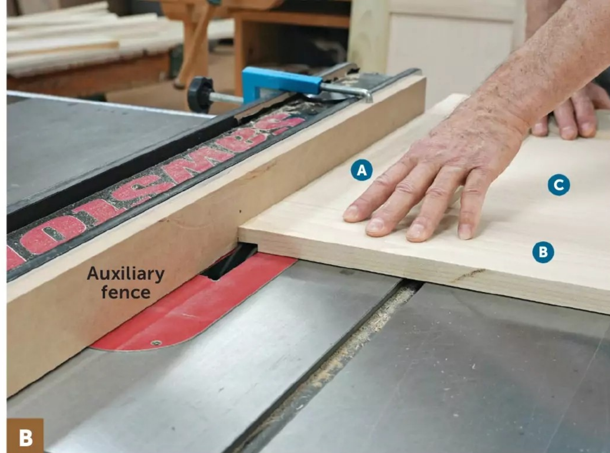
B Attach an auxiliary fence to the tablesaw rip fence and position it to just touch the side of the blade. Use firm downward pressure as you rabbet the top end of each side.
