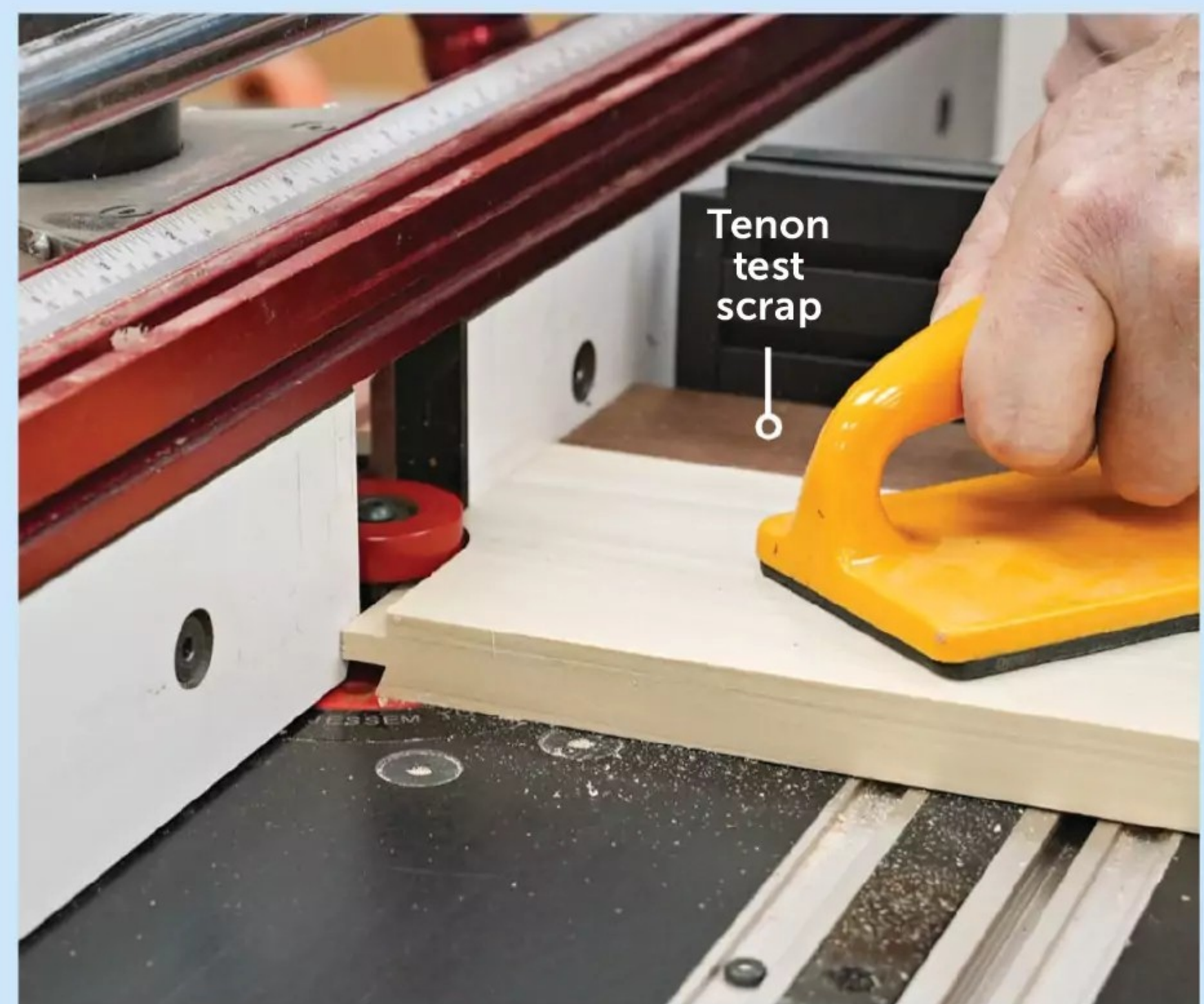
Rout the tenon on each end of the rail using the test scrap as a backer, mating the profiles for routing one end (above), then flipping it to back the square edge for the other.
