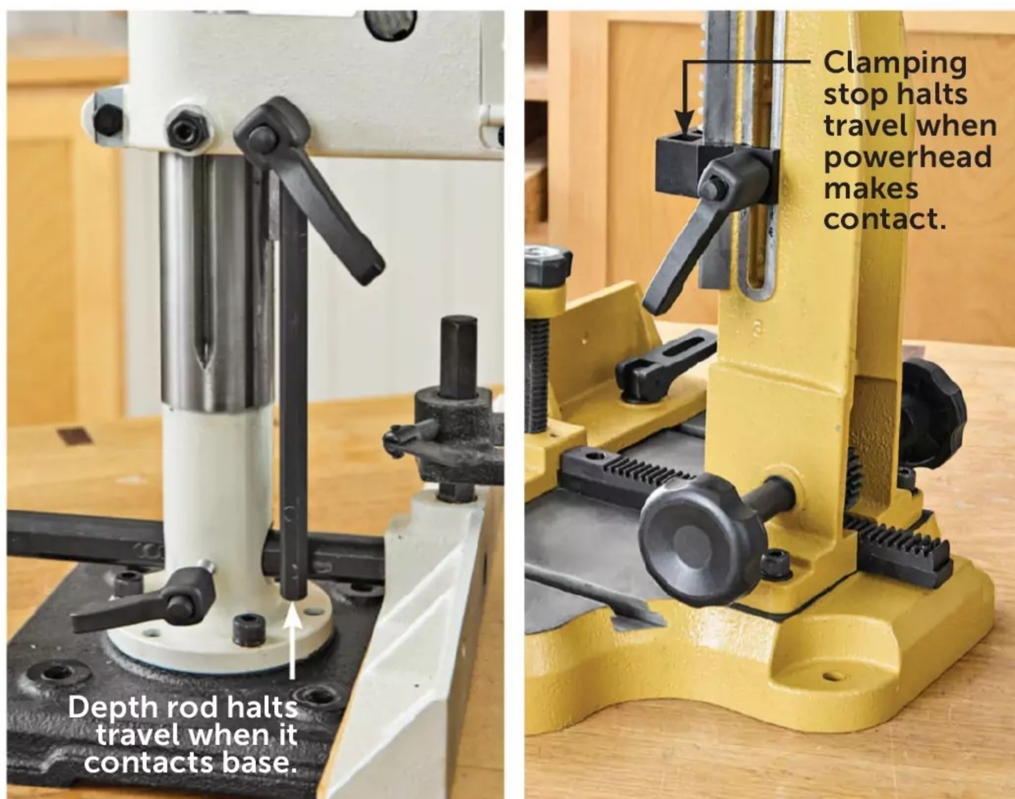
Jet's robust depth-stop rod (left), along with the similar Shop Fox, proved simple and reliable. Powermatic's dovetail-grabbing stop (right) could be knocked loose with an overly aggressive plunge.
