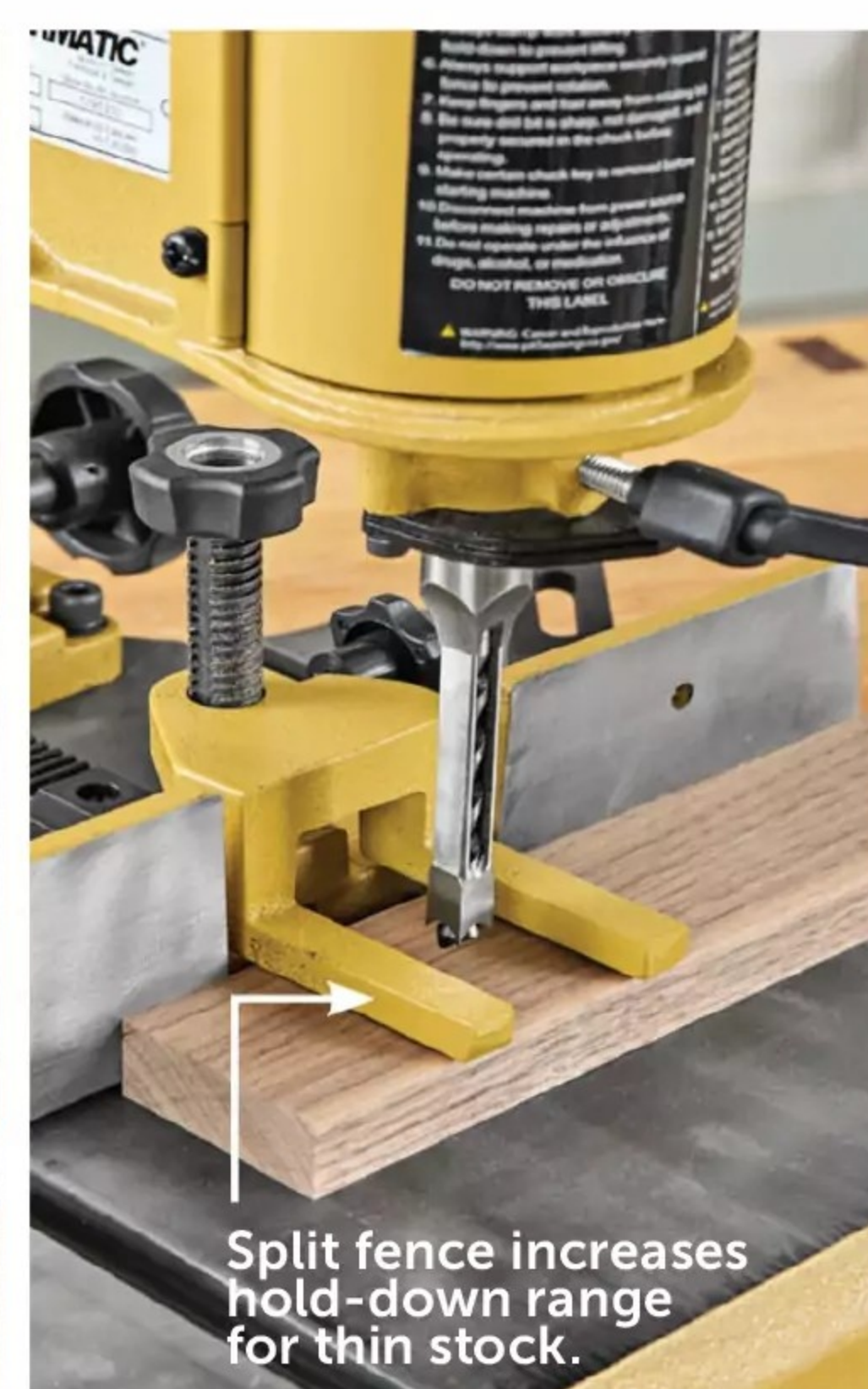
The fence height on six of the mortisers prevents fully lowering the hold-down fork (left), requiring spacers under thin stock. Split fences on the Powermatic (right), Delta, and Grizzly G0645 do not.
