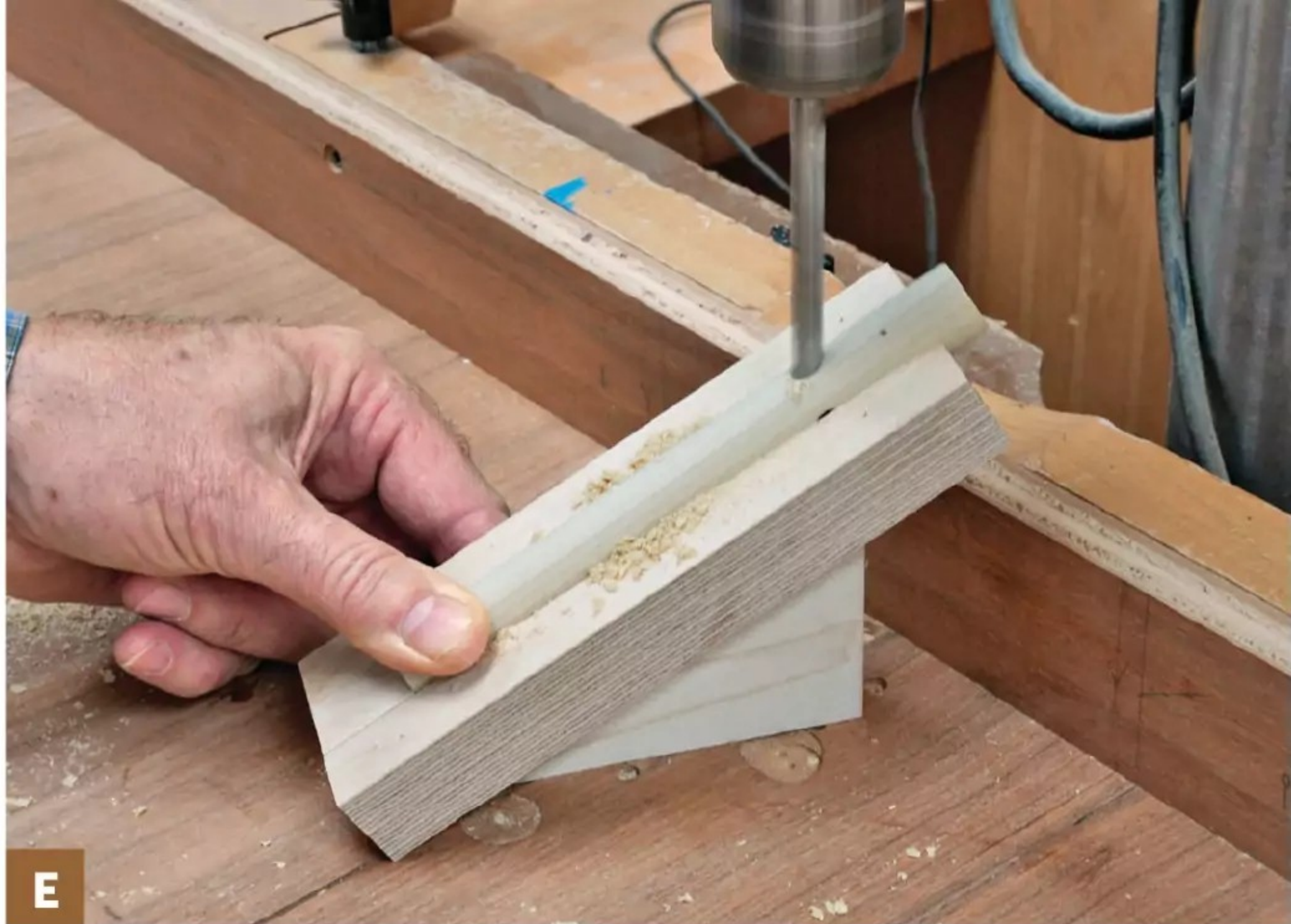
Position a trunk in the jig and drill holes where you want them for the branches. Brad-point bits prevent wandering as you start the holes.
