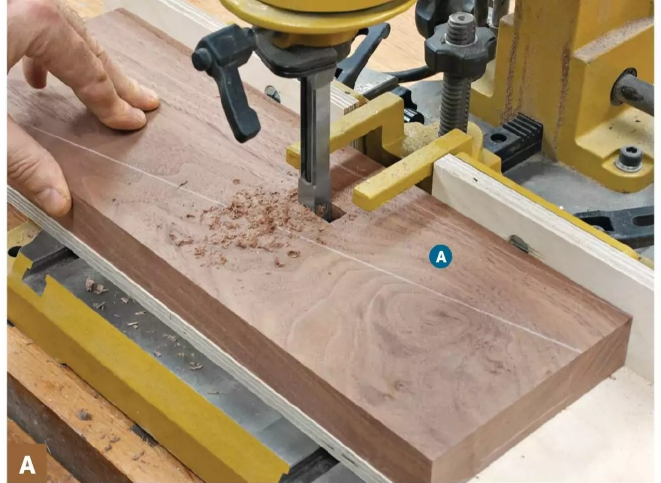
While the leg (A) blanks are still square, cut the mortises. We used a mortising machine with a \frac{1}{2} " chisel, but you can also drill overlapping \frac{1}{2} " holes at the drill press, then chisel the walls and ends square.
