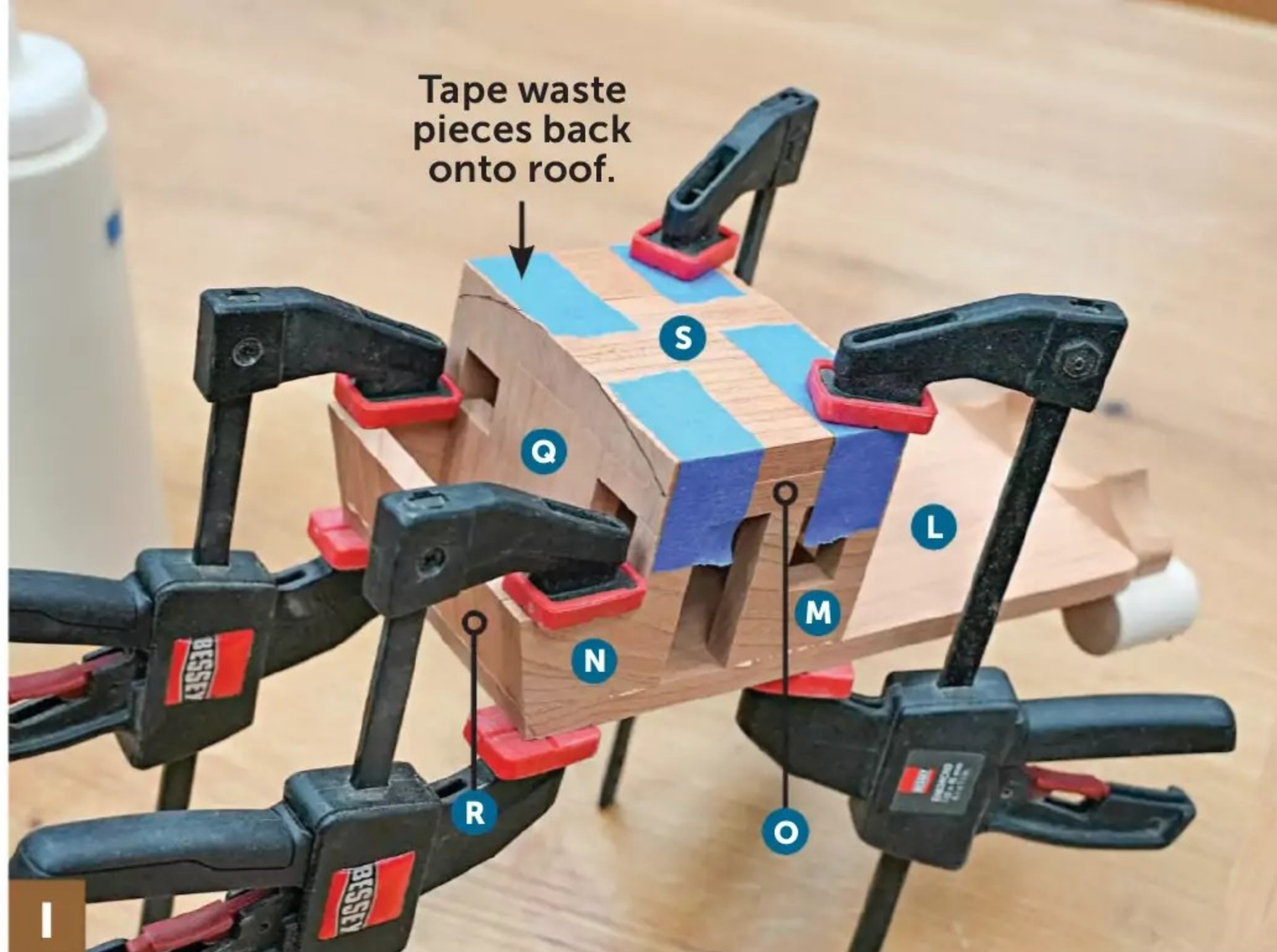
Tape the waste pieces from the roof to the cab assembly to provide a flat clamping surface. Glue and clamp the cab assembly to the back end of the platform, keeping the edges and end flush.
