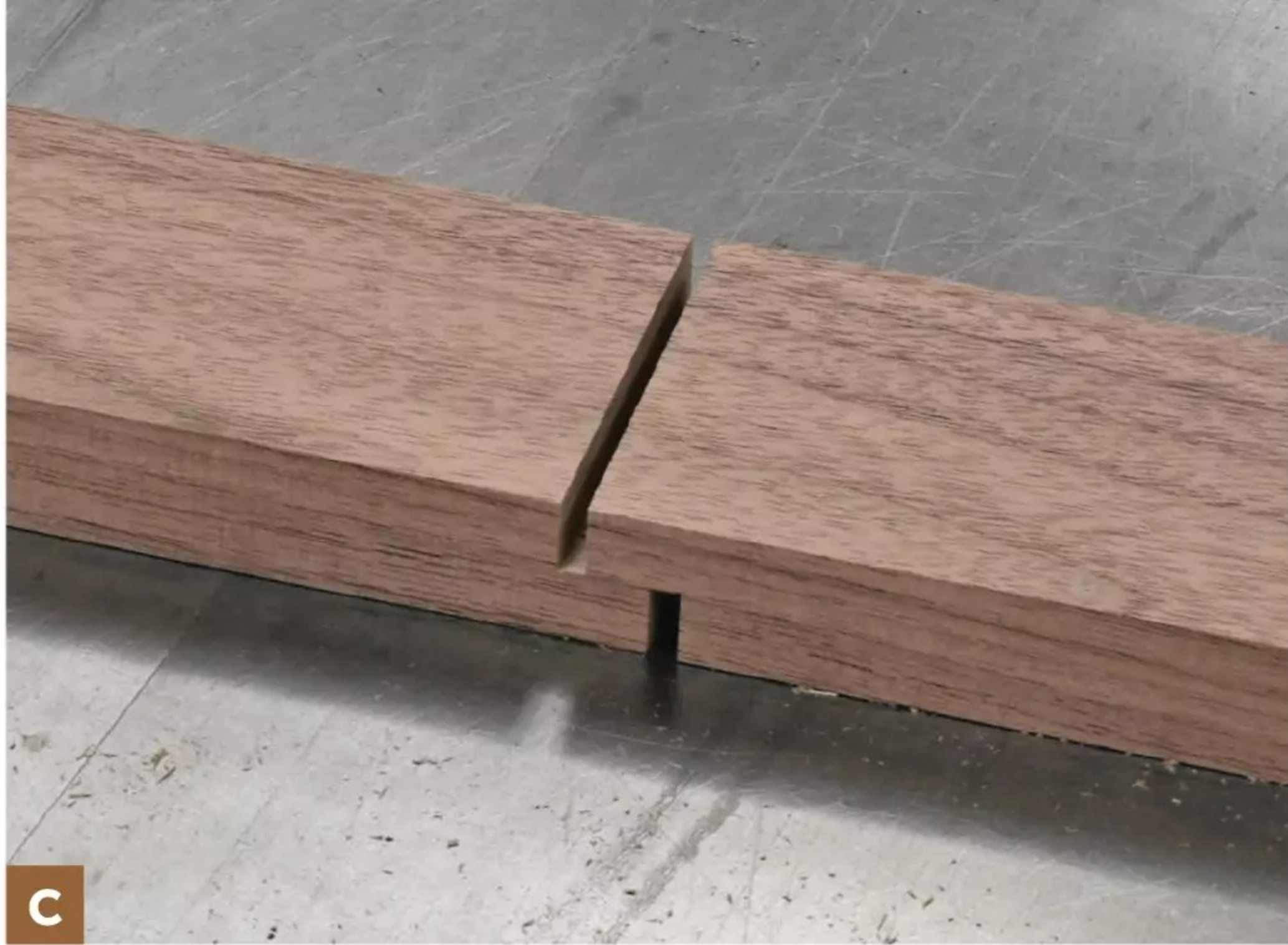
C The dado blade height is set correctly when the faces of the rabbets make contact while the test pieces rest flat on the tablesaw. Start with the blade a bit low and raise it between cuts to get a proper fit.
