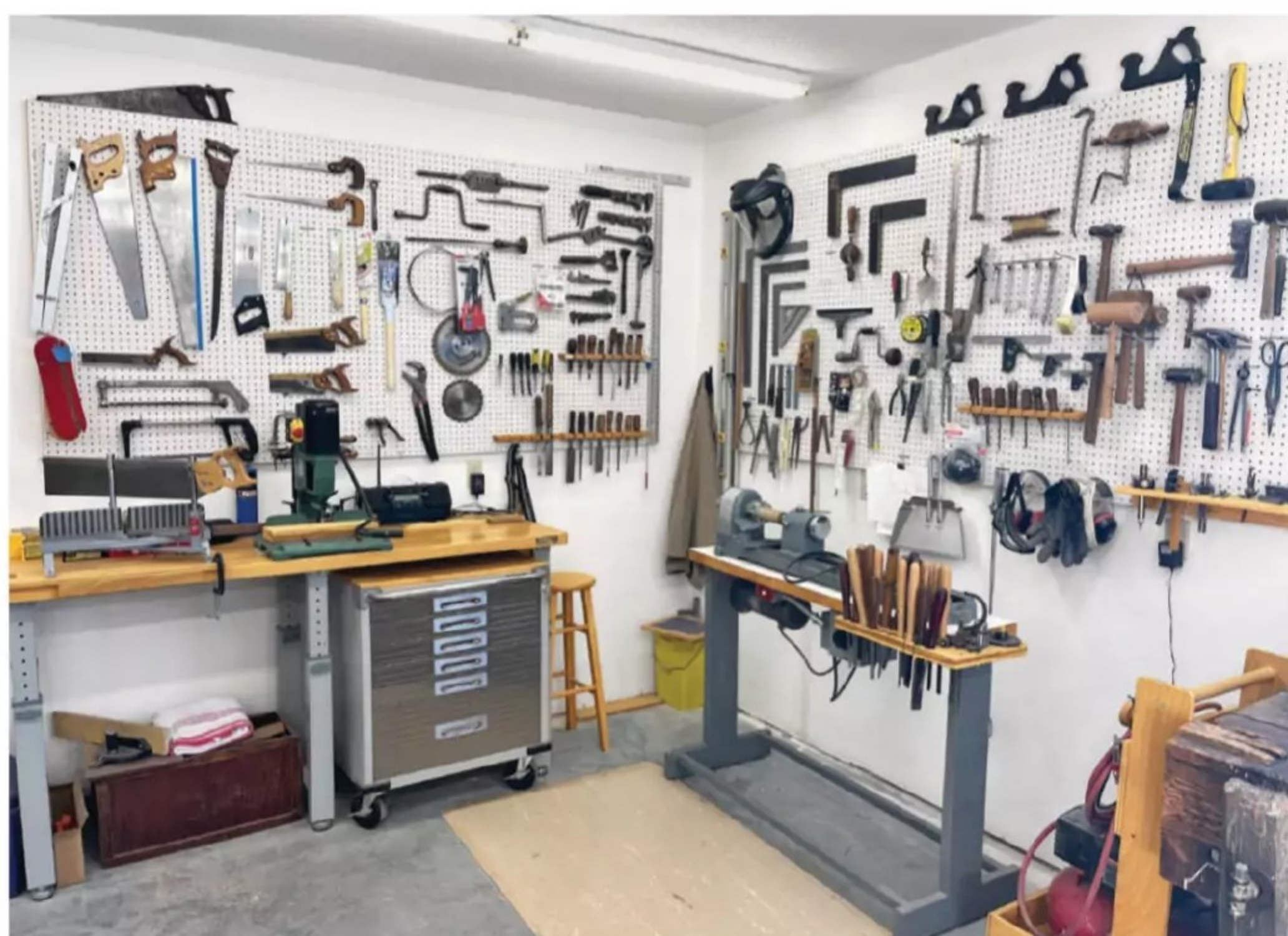
Pegboard panels proved the perfect solution for keeping hand tools organized and easily accessible. Karl says installing these was the first step in organizing the shop.
