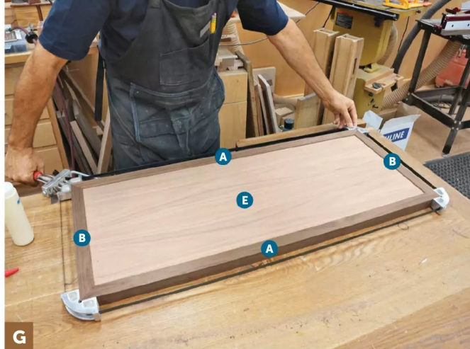
Apply glue to the splines and miters and clamp each side assembly together using a band clamp, checking for square. Clean any glue squeeze-out off of the inside face of the miters.
