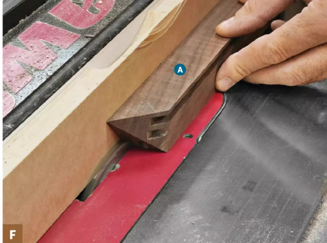
Attach an auxiliary fence to the tablesaw fence and adjust it until it just touches the dado blade. Rabbet the back face of both rear posts and rear rails.
