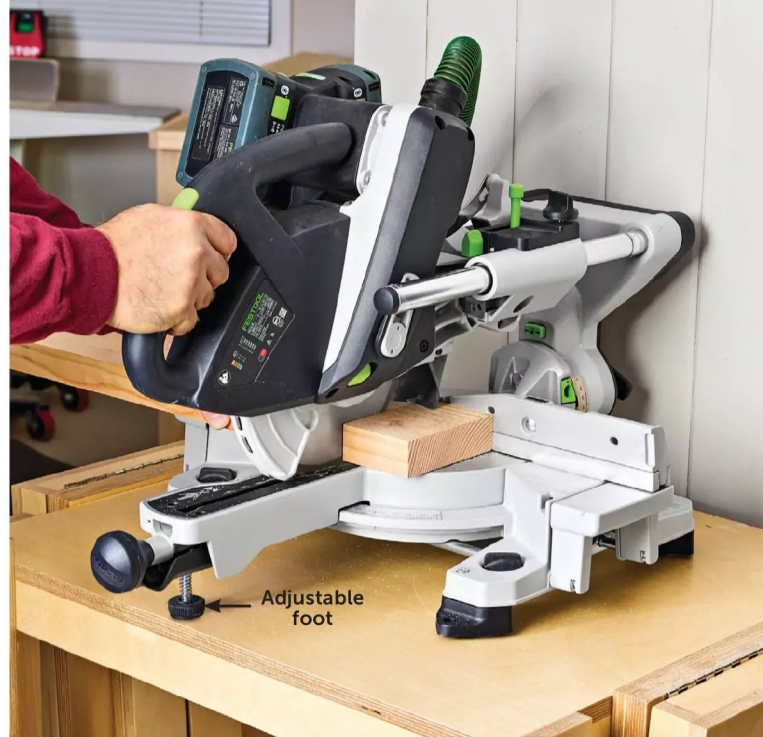
An adjustable foot, like the one on the Festool saw, stabilizes the saw when the blade and motor are pulled forward. The Bauer, Craftsman, Makita, Ryobi, and Worx saws also have this feature.
