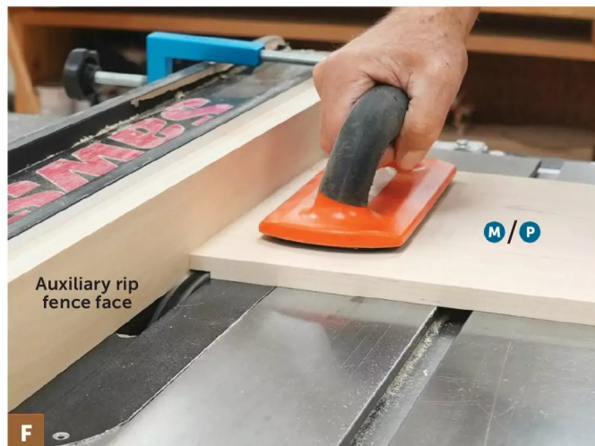
Position an auxiliary fence face so the blade just brushes against it. Rabbet each end of the upper case top and bottom (M) and the lower case sides (P).
