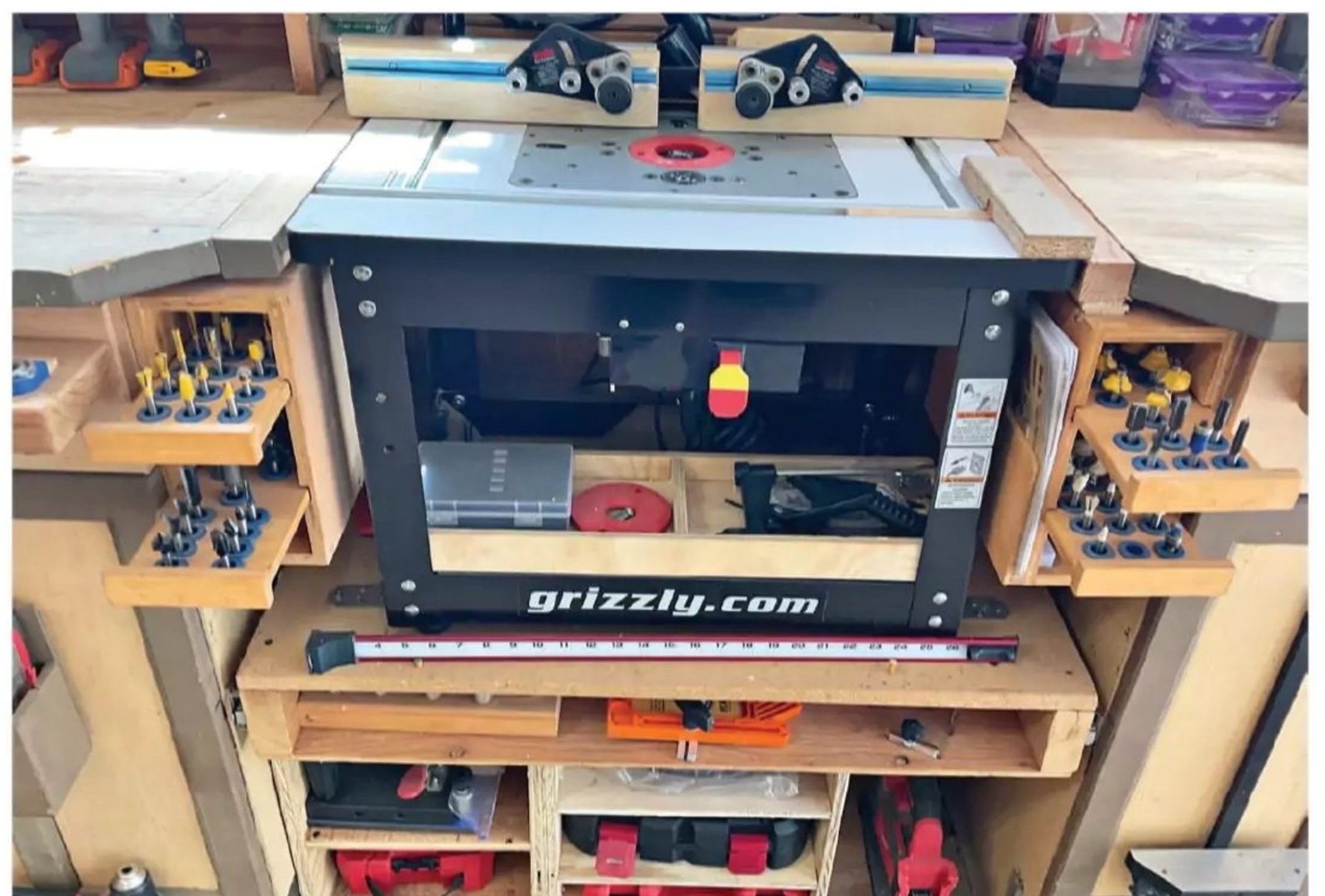
The benchtop router table sits on a sliding platform. Flanking the router table, a pair of cubbies with slide-out trays provide easy router-bit access.
