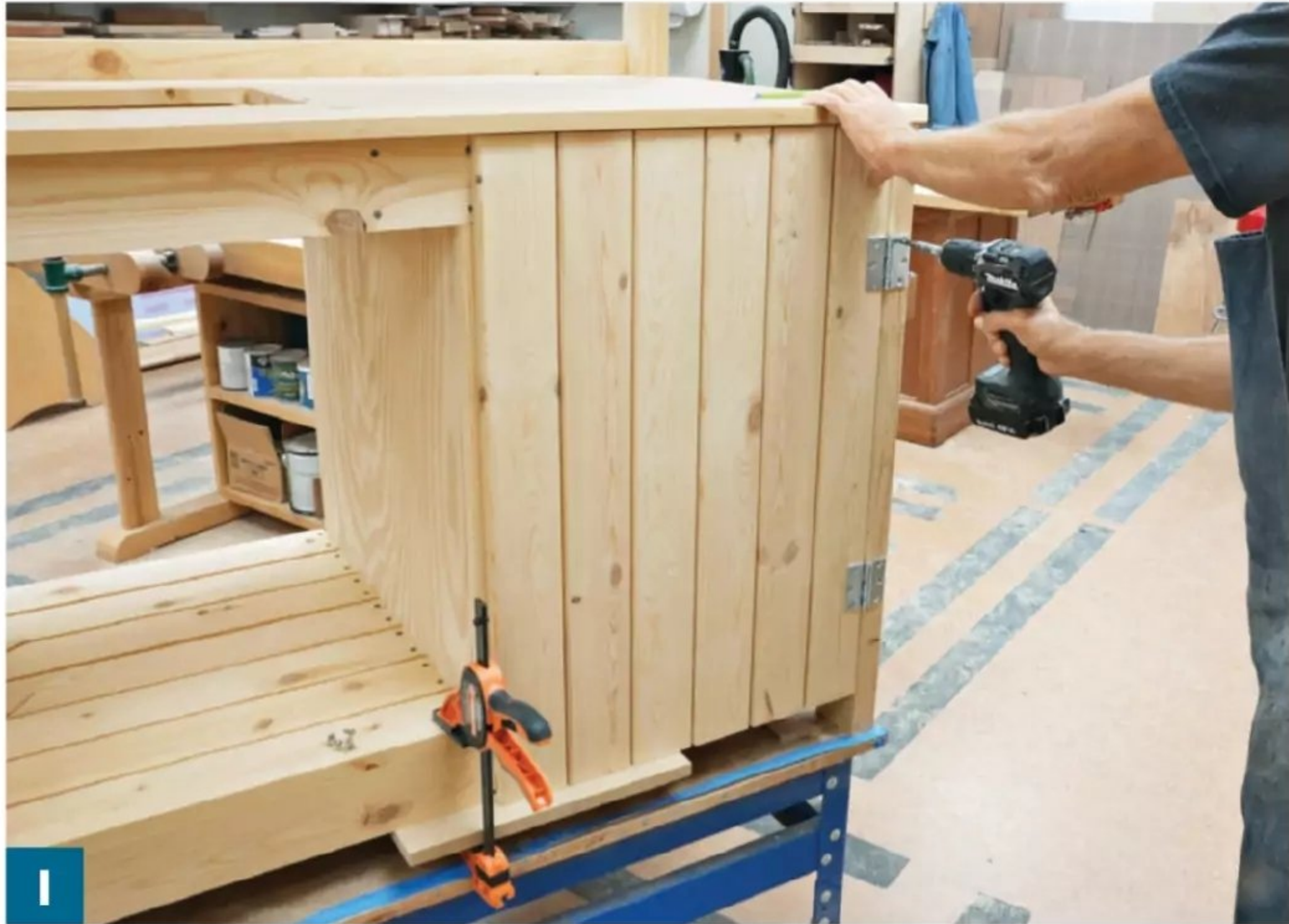
With the hinges attached to the door, clamp a block to the lower stretcher to support the door. Leave a 1/16" gap between the door and the front legs, then screw the hinges to the front leg.
