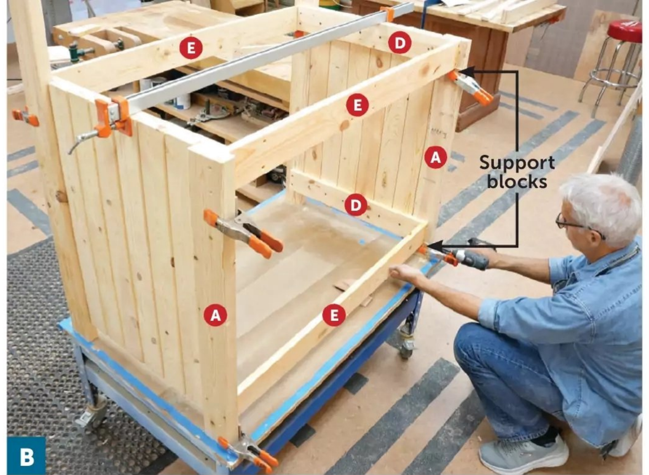
Clamp blocks to the legs (A) to position and support the stretchers (E). Glue the stretchers to the bench rails (D), drill countersunk holes, then drive in screws. Repeat to install the back stretchers.
