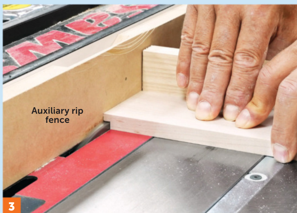
3 Lower the blade slightly and sneak up on the final thickness of the tongue on a test piece. Then, rabbet the drawer front and back. Apply consistent pressure during the cut for an even tongue thickness.
