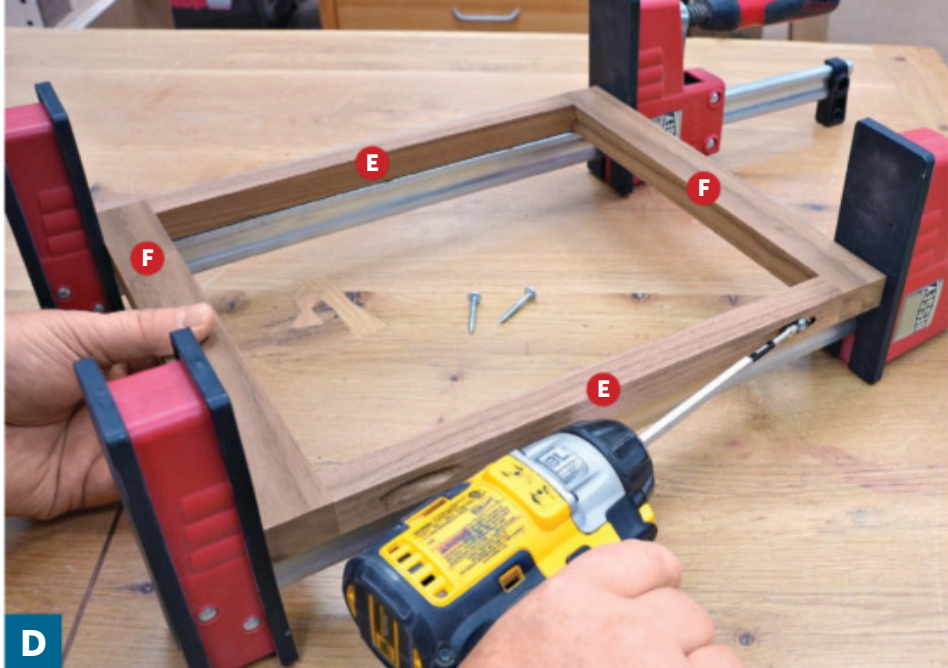
Glue and clamp the wall frame, checking for square. Then drive pocket-hole screws through the rails (E) and into the stiles (F) to reinforce the joints. These screws will be hidden by caps (G).
