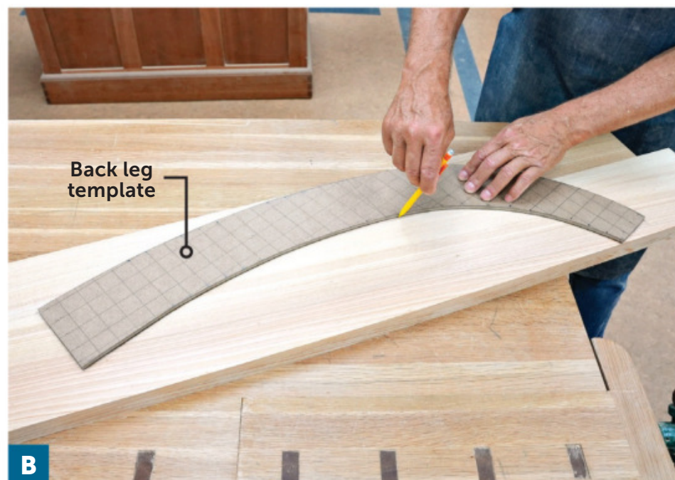
B Scribe the front (A) and back leg (B) templates on the workpiece blanks. Select the sides with the best looking faces and mark them in mirrored pairs so the best sides face out on the finished chair.
