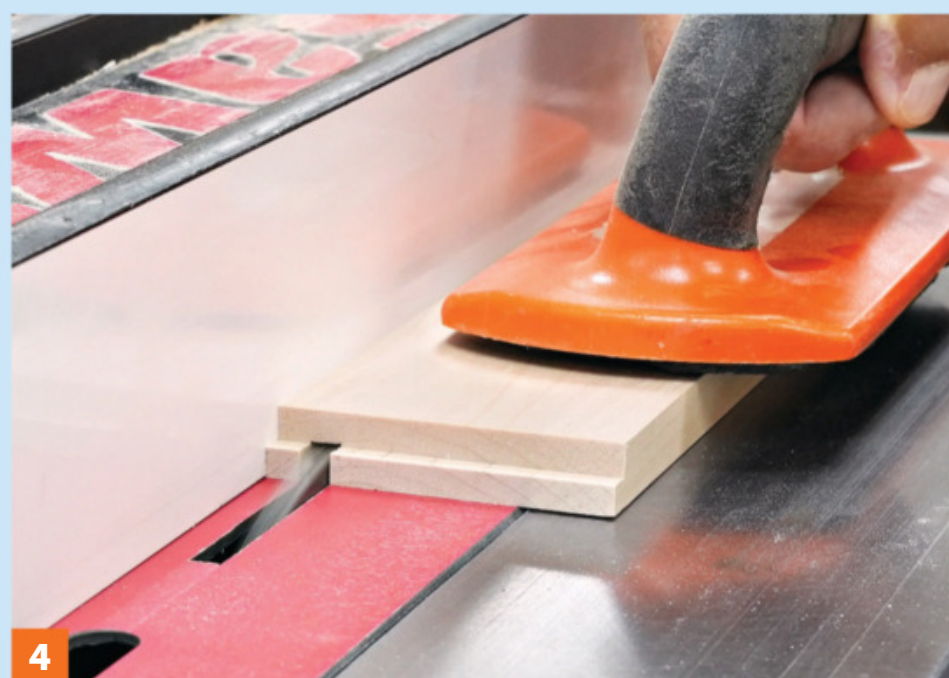
4 Cut the 1/4"-deep groove for the drawer bottom on the inside face of each drawer front, back, and side. A push pad helps apply even pressure throughout the cut.
